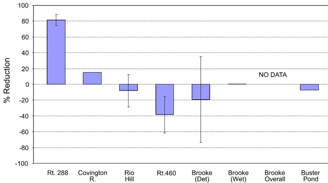
**Table 6. Removal Efficiency for Orthophosphates (OP)**
