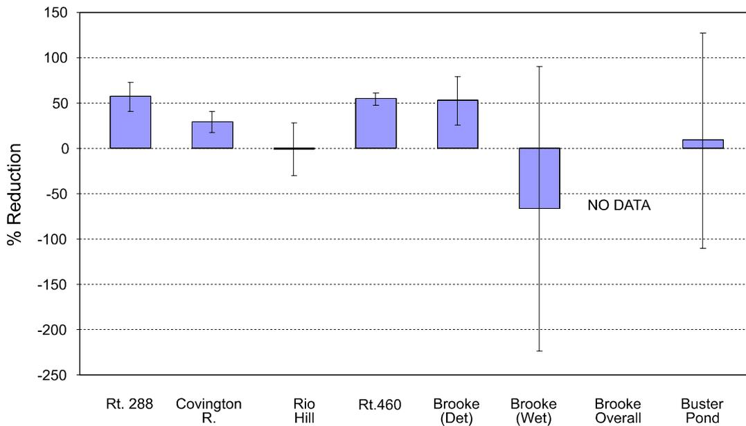
**Table 4. Removal Efficiency for Total Suspended Solids (TSS)**
