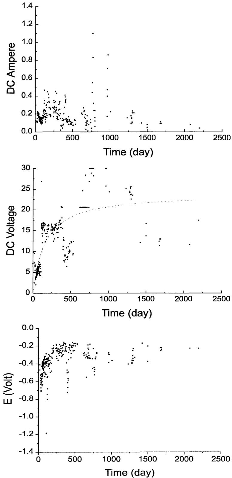
Figure 8. DC Current, Voltage, and Rebar Potential for Circuit 5, CP System 1, Since Installation
