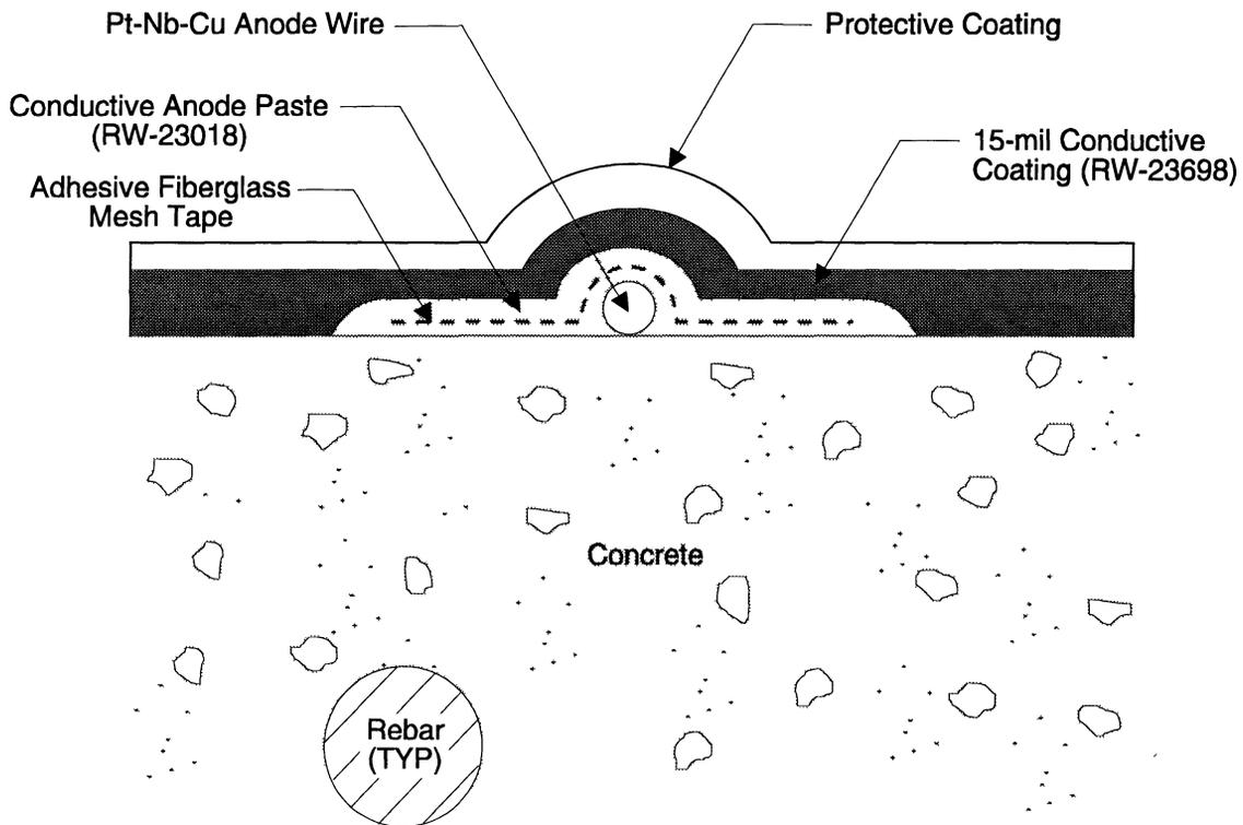
Figure 3. Installation of Anode Wires on Concrete Surface
