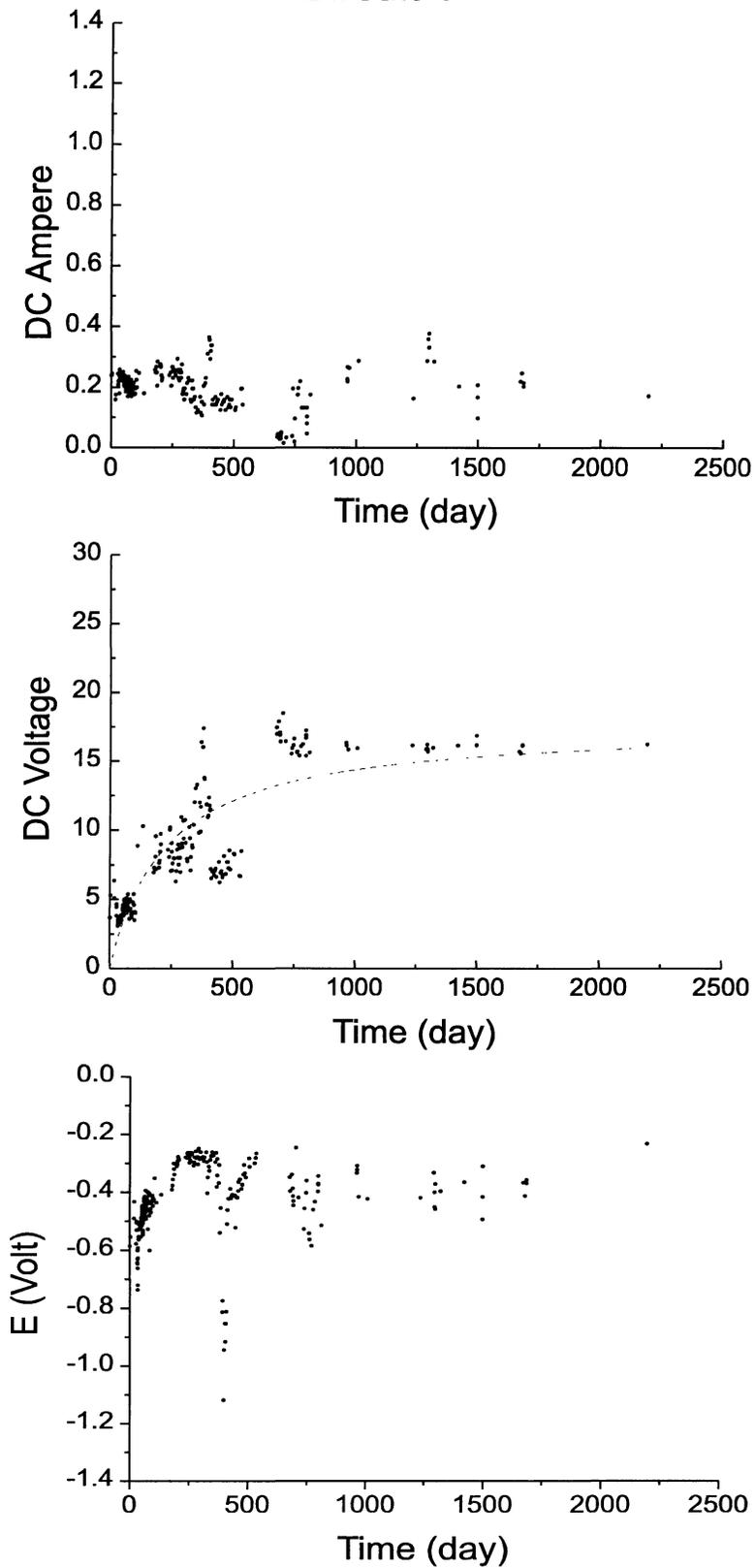
Figure 4. DC Current, Voltage and Rebar Potential for Circuit 1, CP System 1, Since Installation in 1989.
