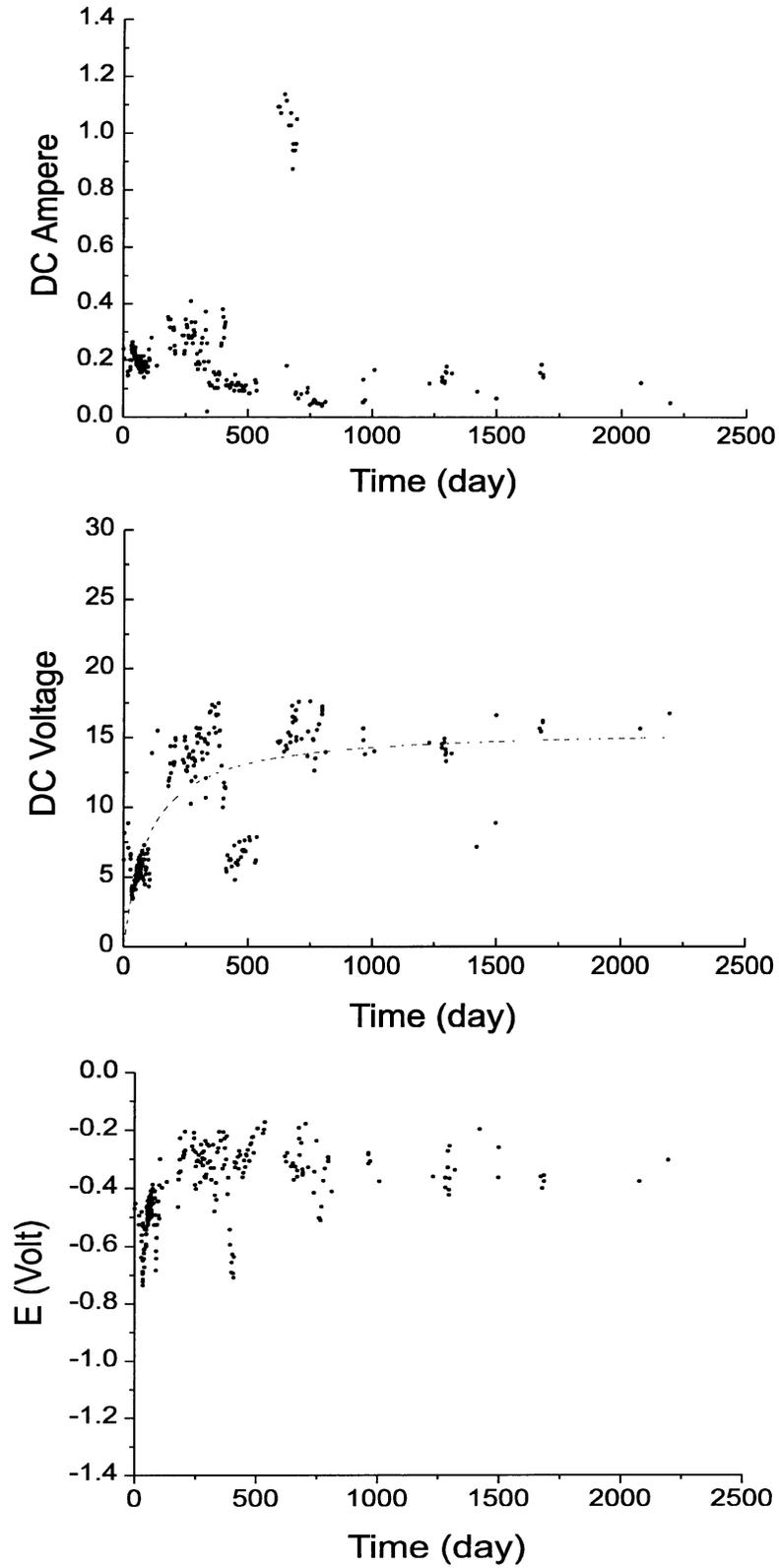
Figure 7. DC Current, Voltage, and Rebar Potential for Circuit 4,CP System 1, Since Installation
