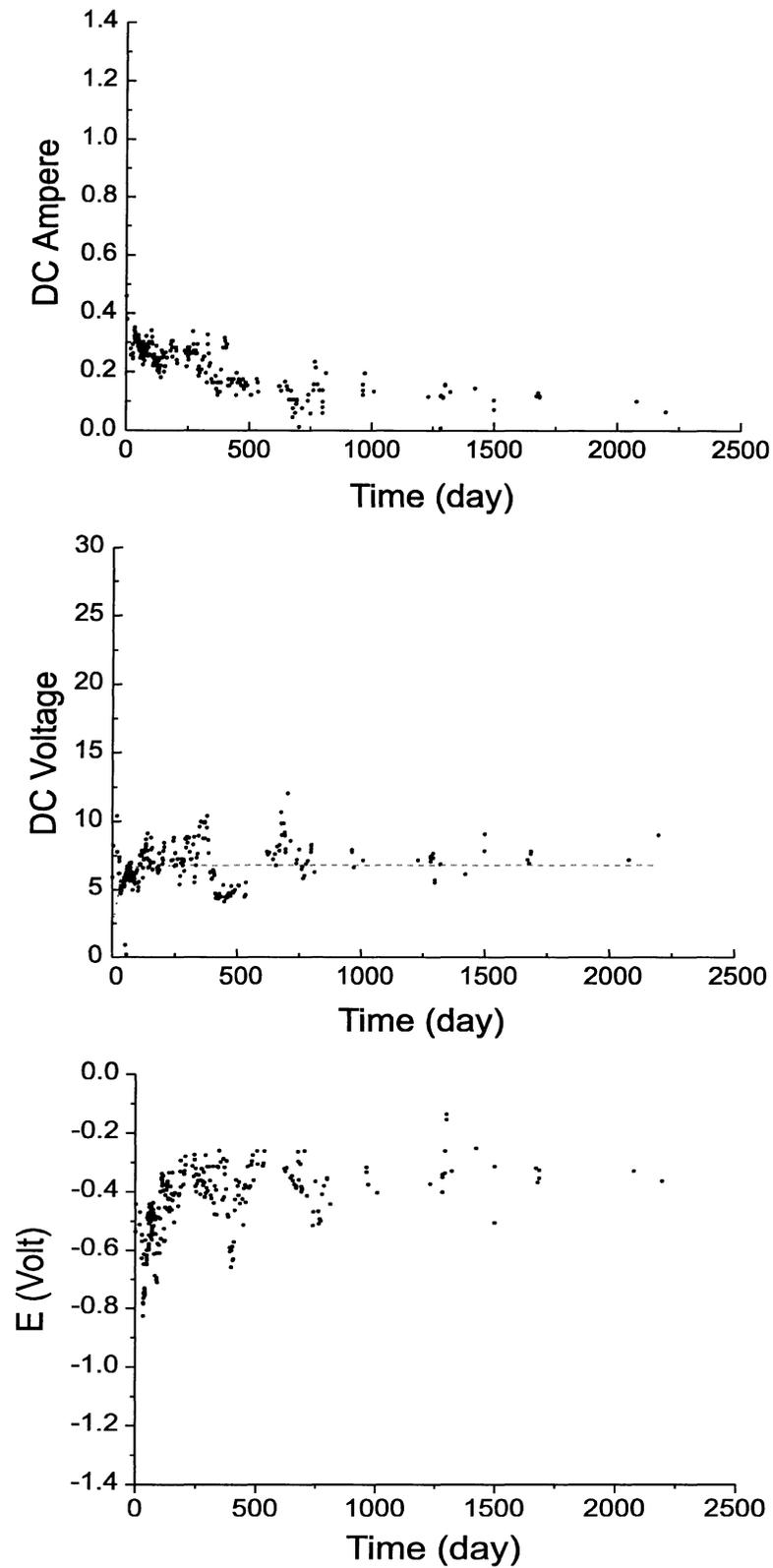
Figure 9. DC Current, Voltage, and Rebar Potential for Circuit 6, CP System 1, Since Installation
