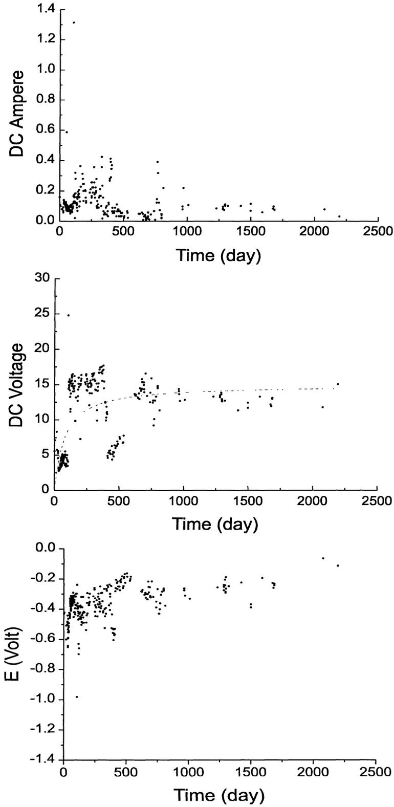
Figure 10. DC Current, Voltage, and Rebar Potential for Circuit 76, CP System 1, Since Installation
