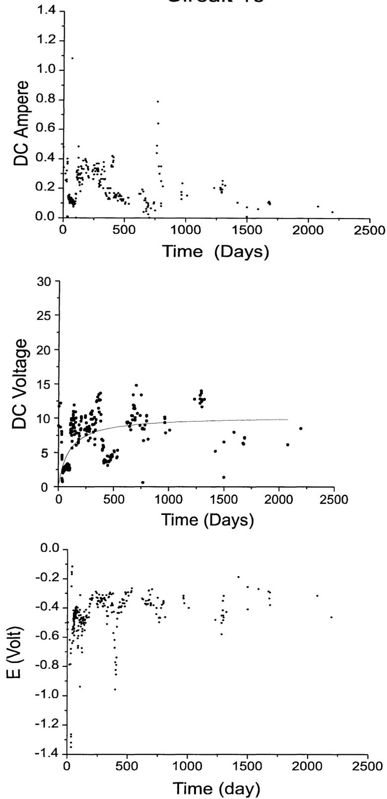
Figure 13. DC Current, Voltage, and Rebar Potential for Circuit 10, CP System 1, Since Installation
