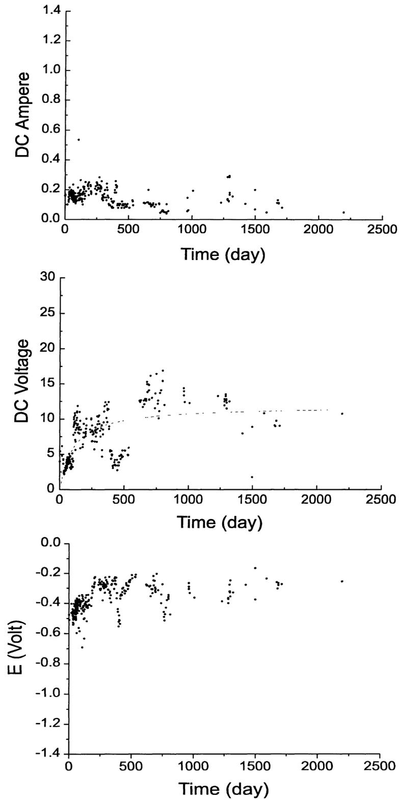
Figure 6. DC Current, Voltage, and Rebar Potential for Circuit 3, CP System 1, Since Installation
