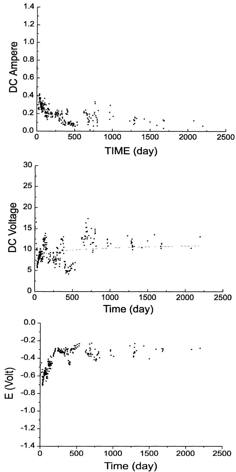
Figure 11. DC Current, Voltage, and Rebar Potential for Circuit 8, CP System 1, Since Installation
