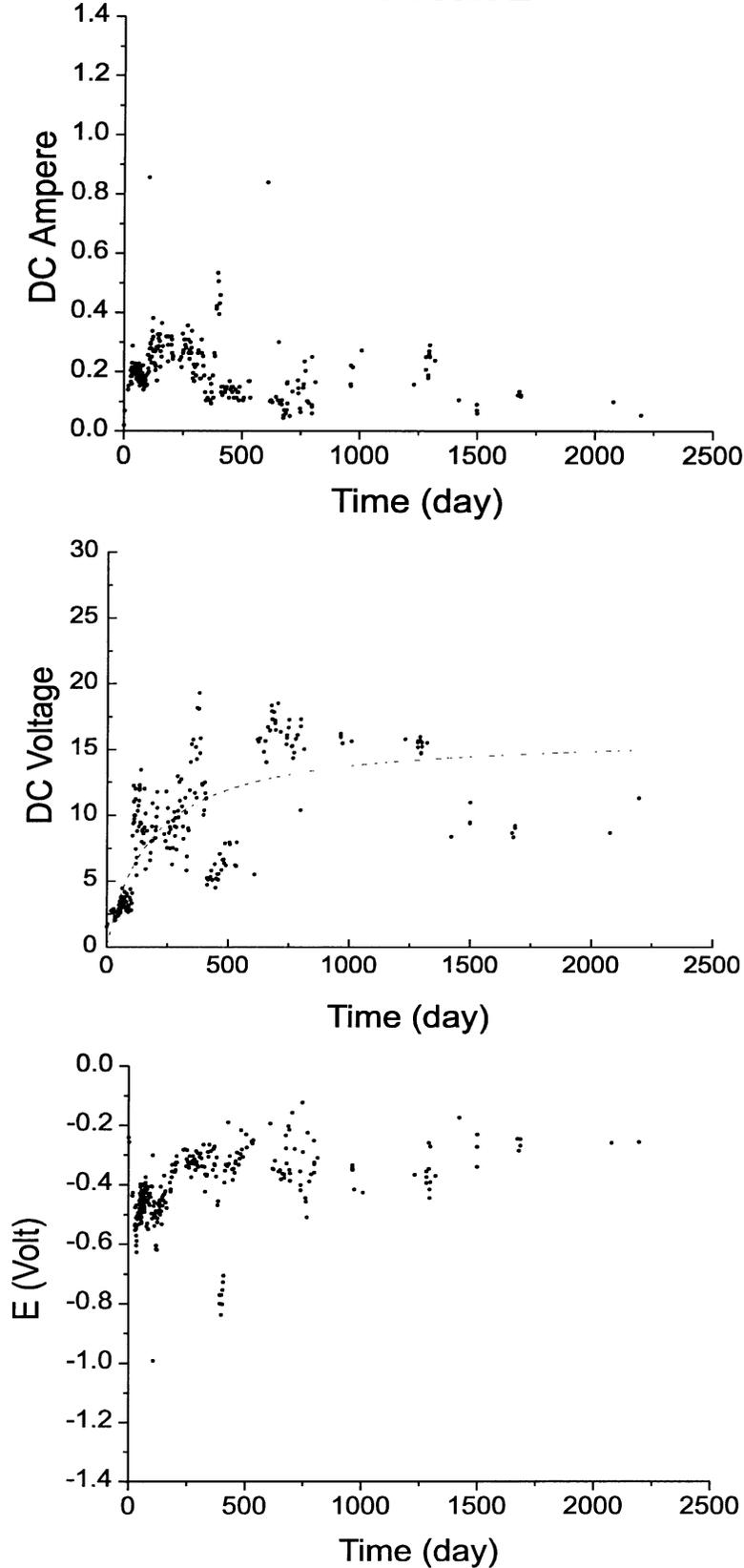
Figure 5. DC Current, Voltage, and Rebar Potential for Circuit 2, CP System 1, Since Installation
