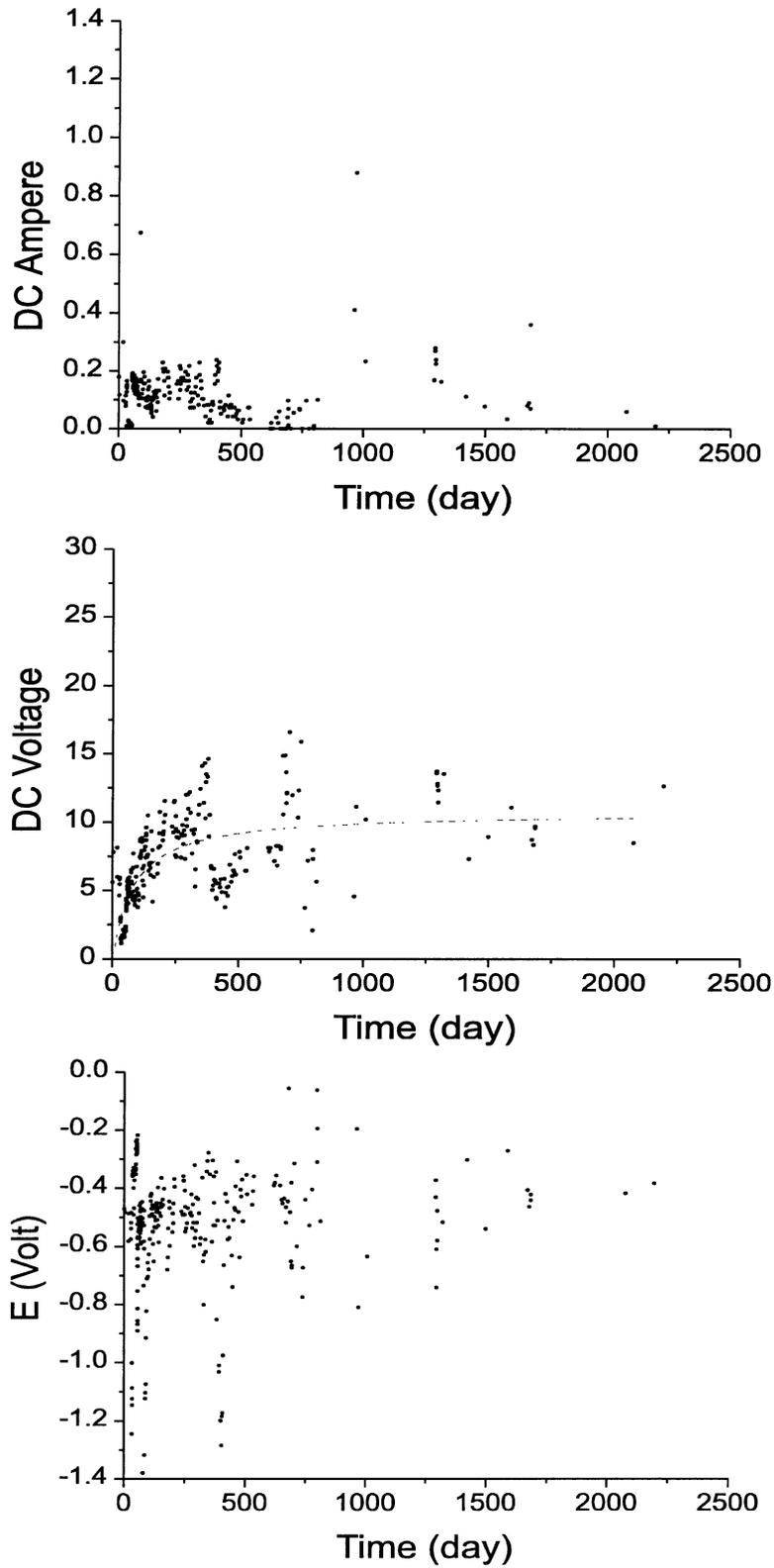
Figure 12. DC Current, Voltage, and Rebar Potential for Circuit 9, CP System 1, Since Installation
