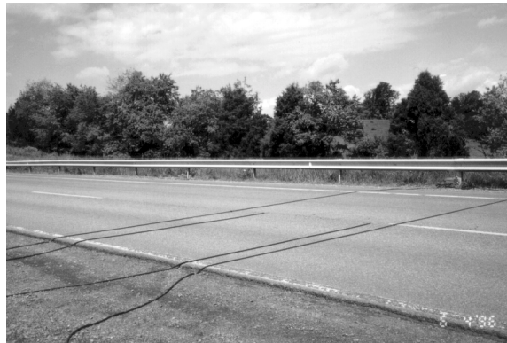
Figure 5. Layout of tubes across the road.
