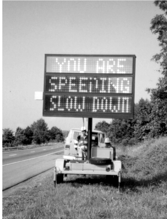
Figure 4. The CMS with message display.
