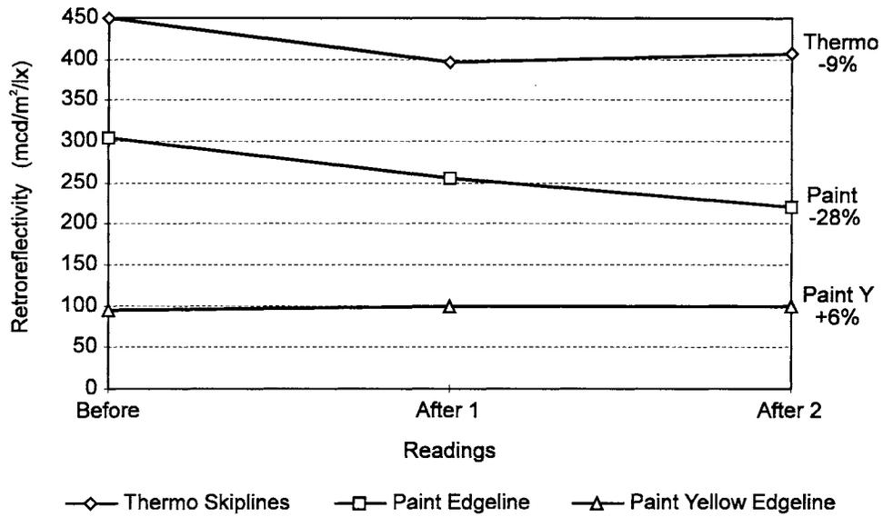
Figure 4. Site 5 (Paint vs. Thermoplastic)
