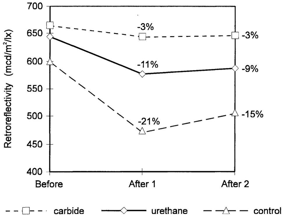
Figure 6. Retroreflectivity of Waffle Tape Skiplines
