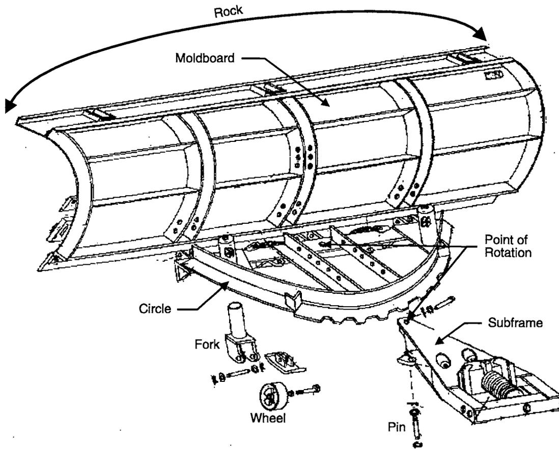
Figure 2. Plow Moldboard and Frame
