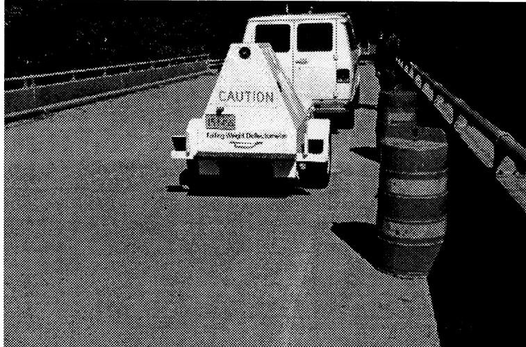
**Figure 2. Falling Weight Deflectometer**
