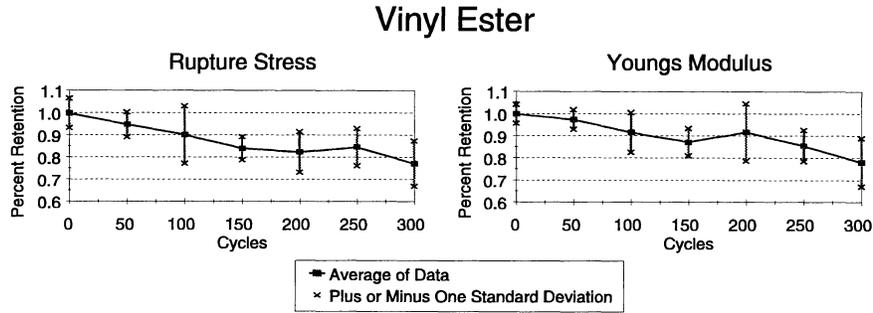
**Figure 5.** Rupture stress and Young’s modulus calculations for Vinyl Ester.
