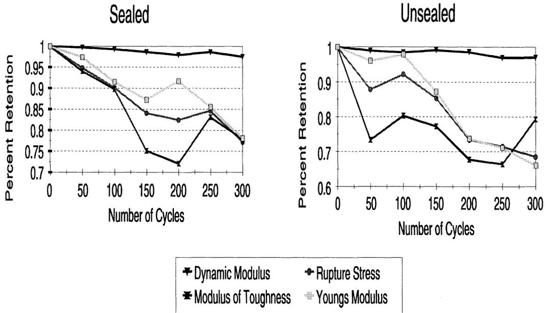
Figure 3. Vinyl Ester freeze/thaw degradation.
