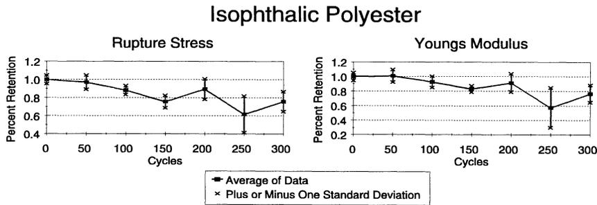
**Figure 6.** Rupture stress and Young’s modulus calculations for Isophthalic Polyester.
