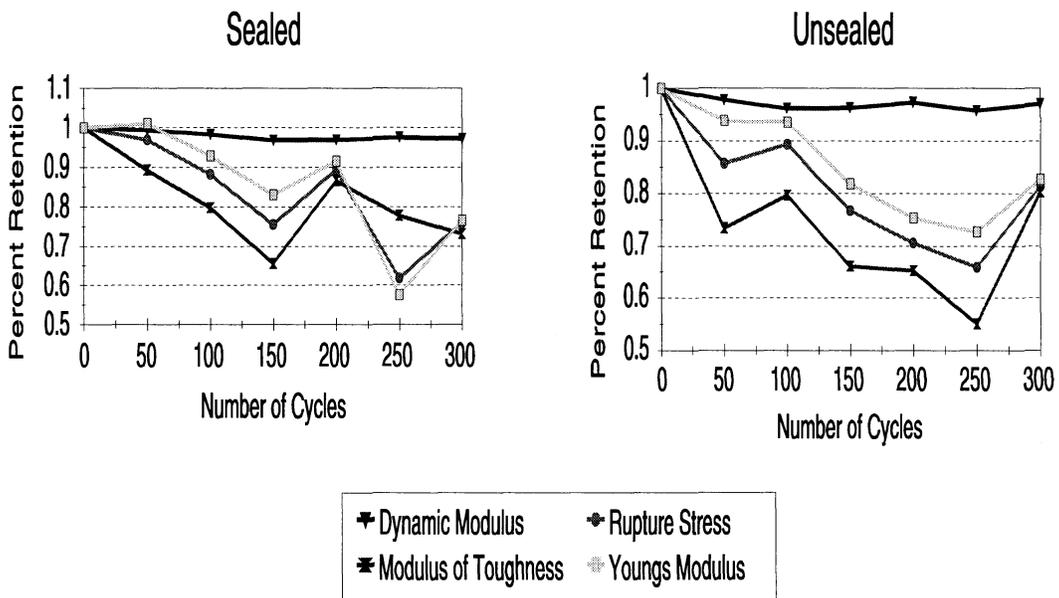
Figure 4. Isophthalic Polyester freeze/thaw degradation.
