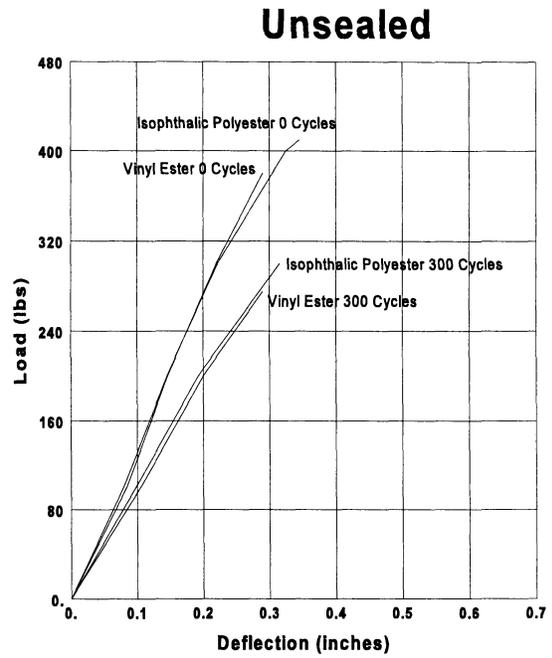
**Figure 1. Load vs. Deflection, Sealed Edges** **Figure 2. Load vs. Deflection, Unsealed Edges**
