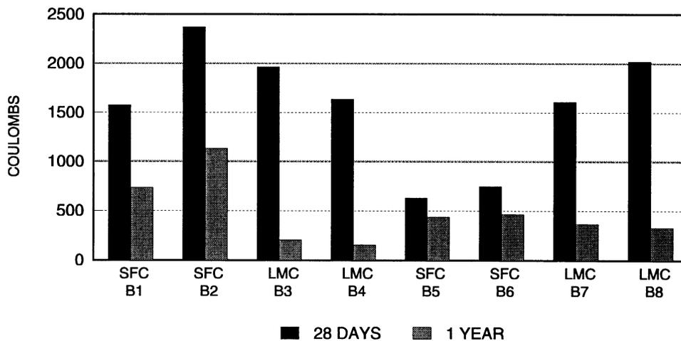
**Figure 4. Permeability of SFC and LMC at 28 Days and 1 Year**
