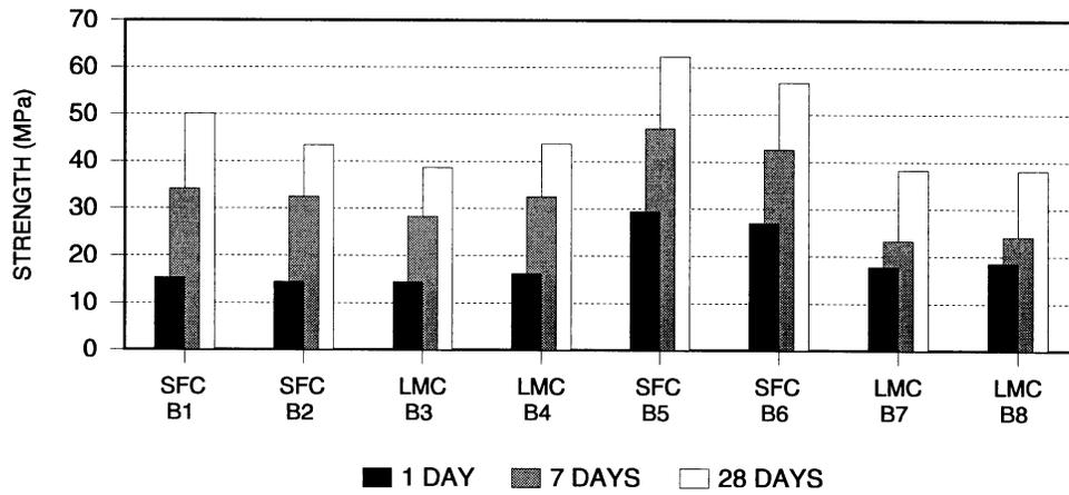
**Figure 1. Compressive Strength of SFC and LMC at 1, 7, and 28 Days**
