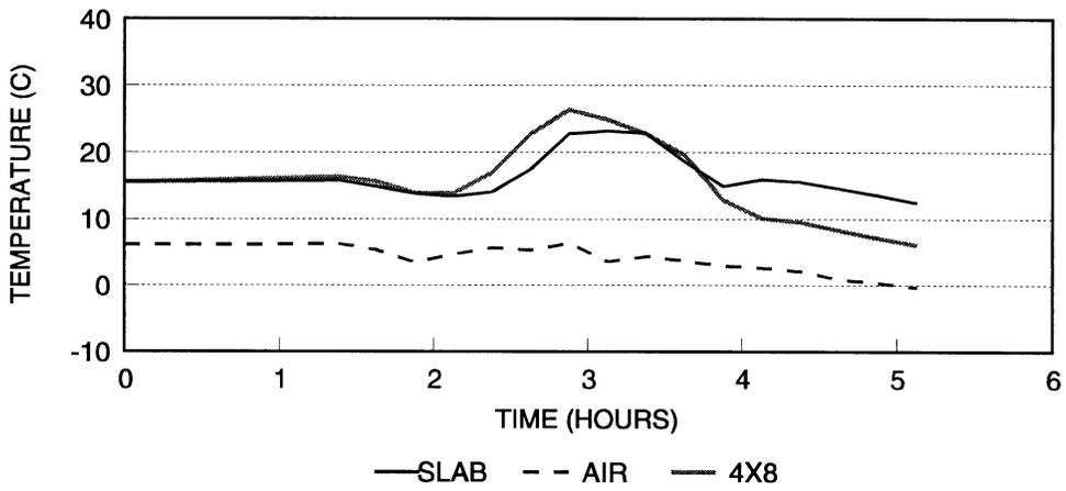
Figure 6. Temperature Development of PBCC at Low Ambient Temperatures
