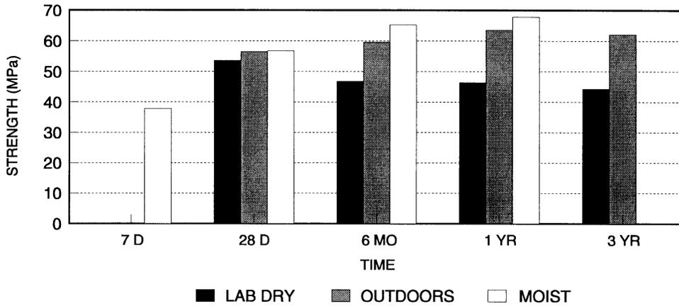
**Figure 2. Compressive Strength of SFC Under Different Curing Conditions**
