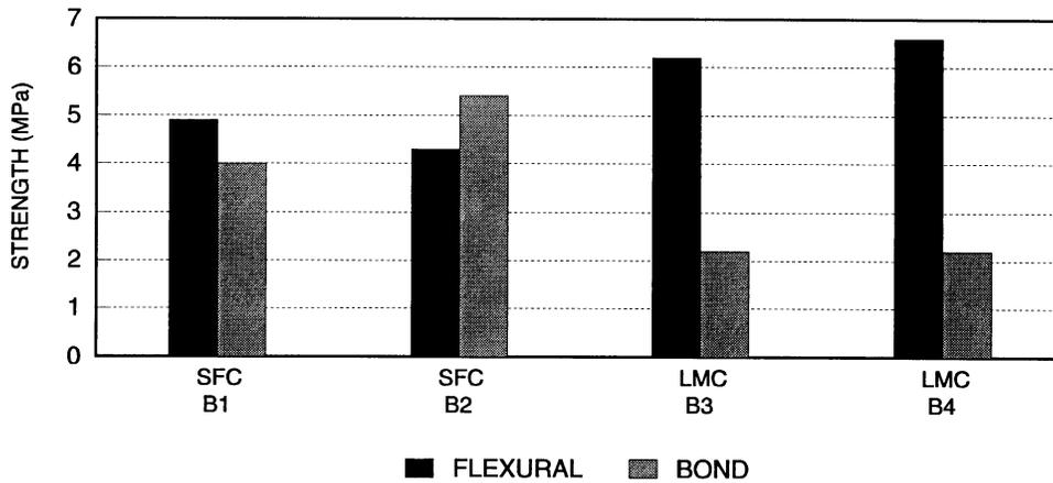
**Figure 3. Flexural and Bond Strength of SFC and LMC at 28 Days**
