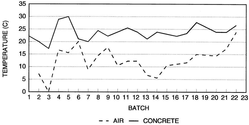
Figure 5. Air and Concrete Temperatures for PBCC
