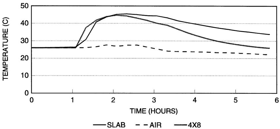
Figure 7. Temperature Development of PBCC at Moderate Ambient Temperatures
