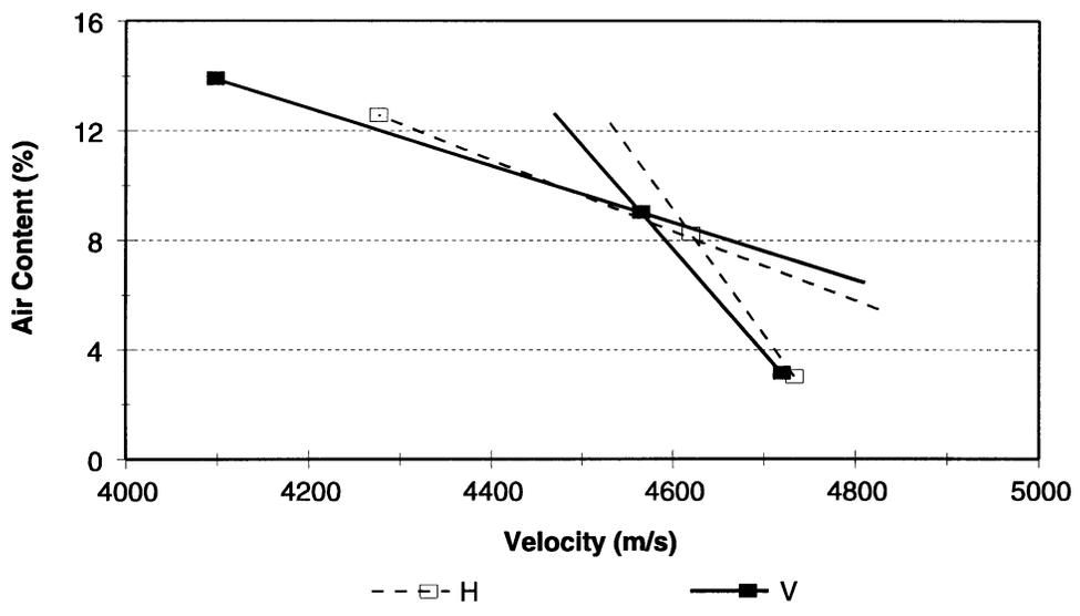
FIGURE 10. AIR CONTENT VERSUS VELOCITY
