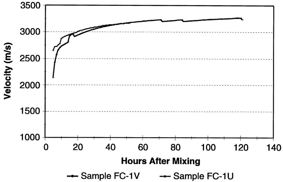
FIGURE 19. VELOCITY VERSUS TIME FOR VIBRATED AND HAND CONSOLIDATED CONCRETE WITH 3% AIR (1.3% ENTRAPPED)
