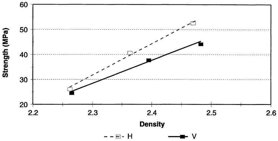
FIGURE 8. STRENGTH VERSUS DENSITY
