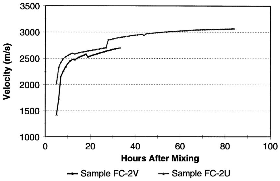
FIGURE 20. VELOCITY VERSUS TIME FOR HAND CONSOLIDATED CONCRETE WITH 8% AIR (1.5% ENTRAPPED) AND VIBRATED CONCRETE WITH 9% AIR (1.9% ENTRAPPED)
