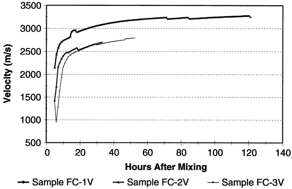
FIGURE 17. VELOCITY VERSUS TIME FOR VIBRATED CONCRETE AFTER MIXING
