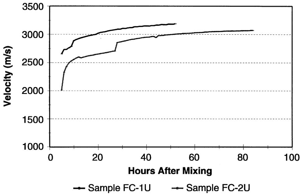
FIGURE 18. VELOCITY VERSUS TIME FOR HAND CONSOLIDATED CONCRETE AFTER MIXING
