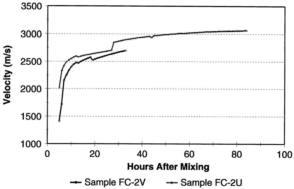
FIGURE 14. RATE OF CHANGE OF VELOCITY VERSUS TIME AFTER MIXING FOR VIBRATED CONCRETE WITH 3% AIR (1.3% ENTRAPMENT)
