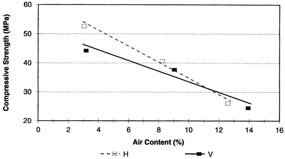
FIGURE 7. STRENGTH VERSUS AIR CONTENT
