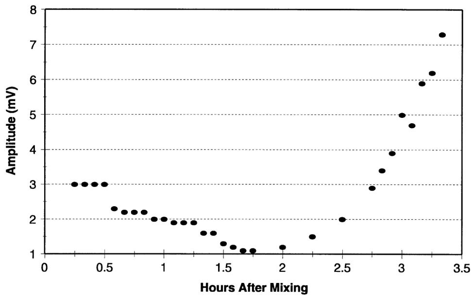
FIGURE 12. AMPLITUDE VERSUS TIME FOR FRESH CONCRETE WITH 3% AIR CONTENT (1.3% ENTRAPPED)
