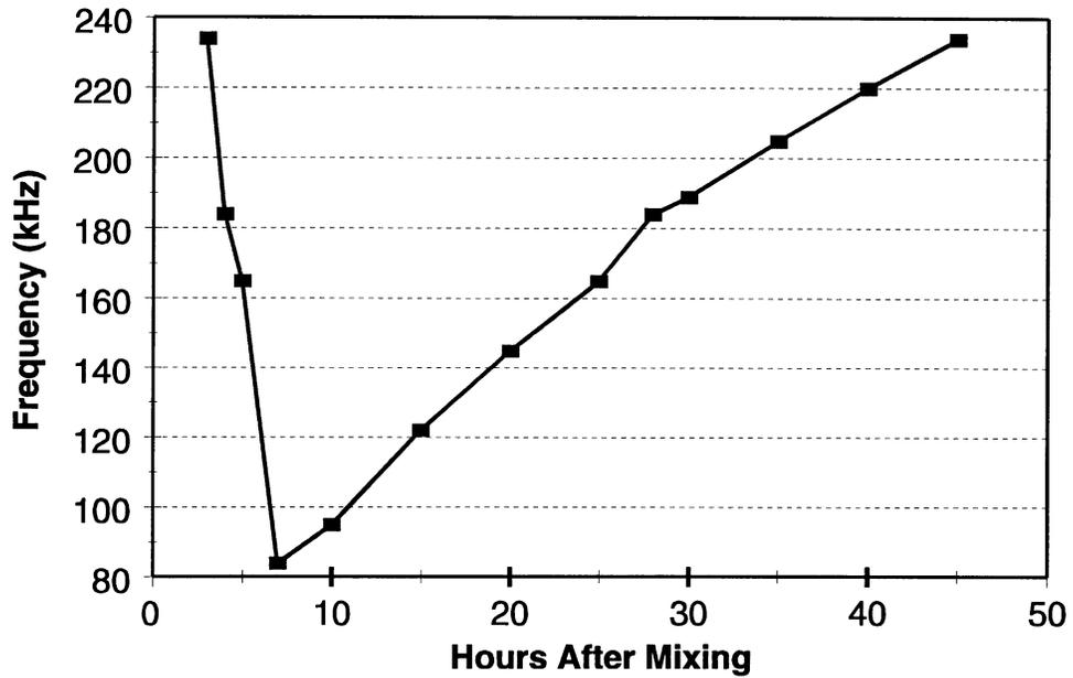
FIGURE 15. FREQUENCY VERSUS TIME AFTER MIXING FOR HYDRATING CONCRETE WITH 12% AIR (1.5% ENTRAPMENT)
