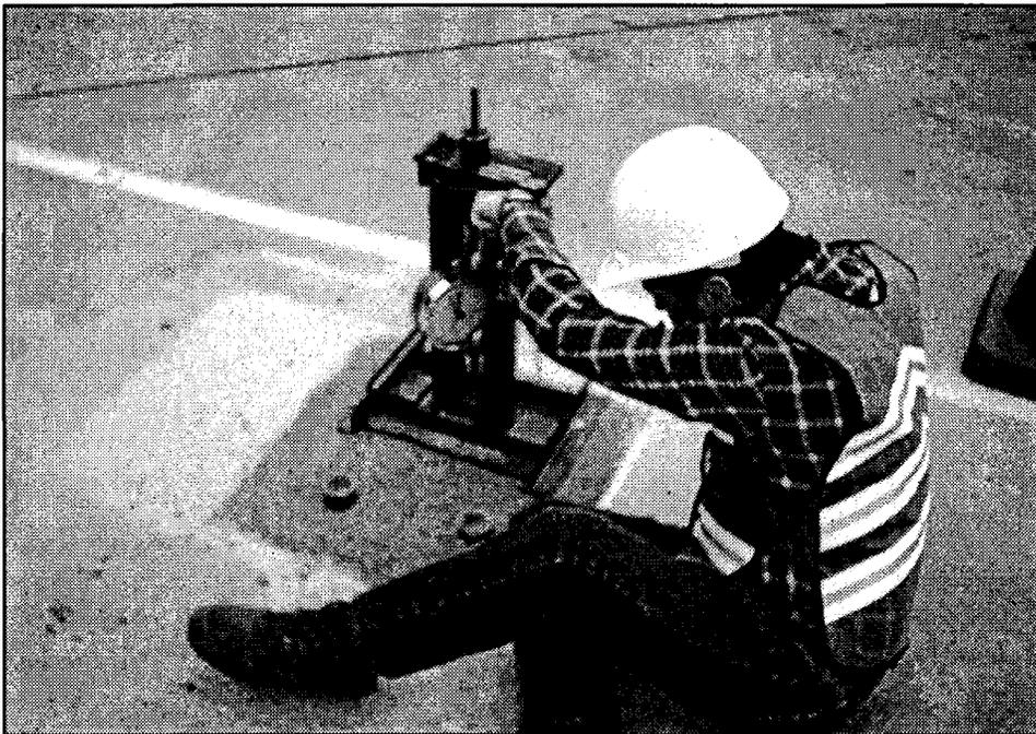
Figure 153. A dynamometer with a capacity of at least 2,000 lbs should be hooked to the pipe cap and the loading hook and the load applied at the rate of 100 lbs every 5 sec. The dynamometer reading at rupture and the type failure, as percent concrete, bond, and overlay should be recorded.
