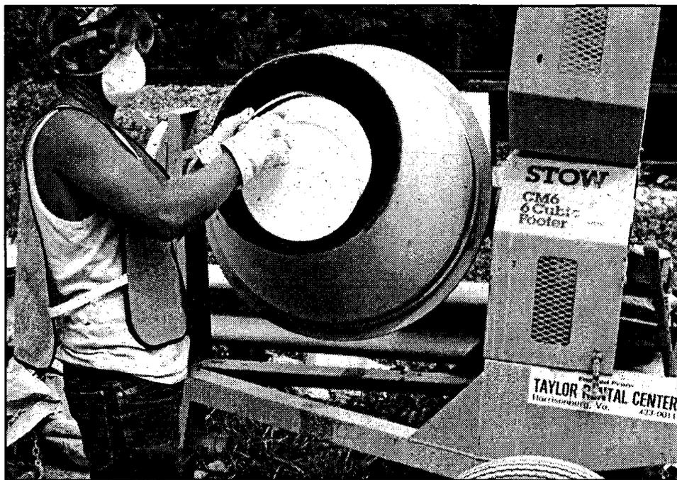
Figure 169. Polyester styrene resin is here added to the concrete mixer.
