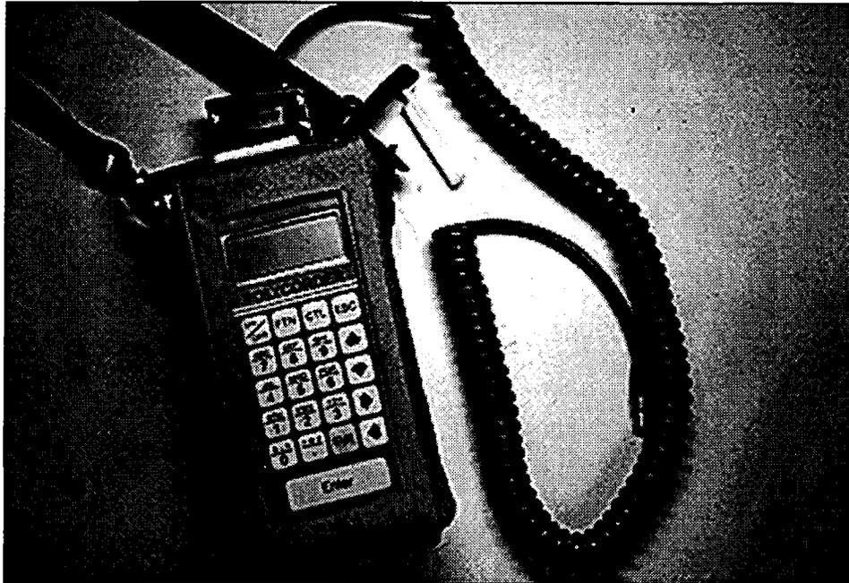
Figure 29. Half-cell potential measurements can be recorded on a datalogger and later downloaded onto a personal computer.
