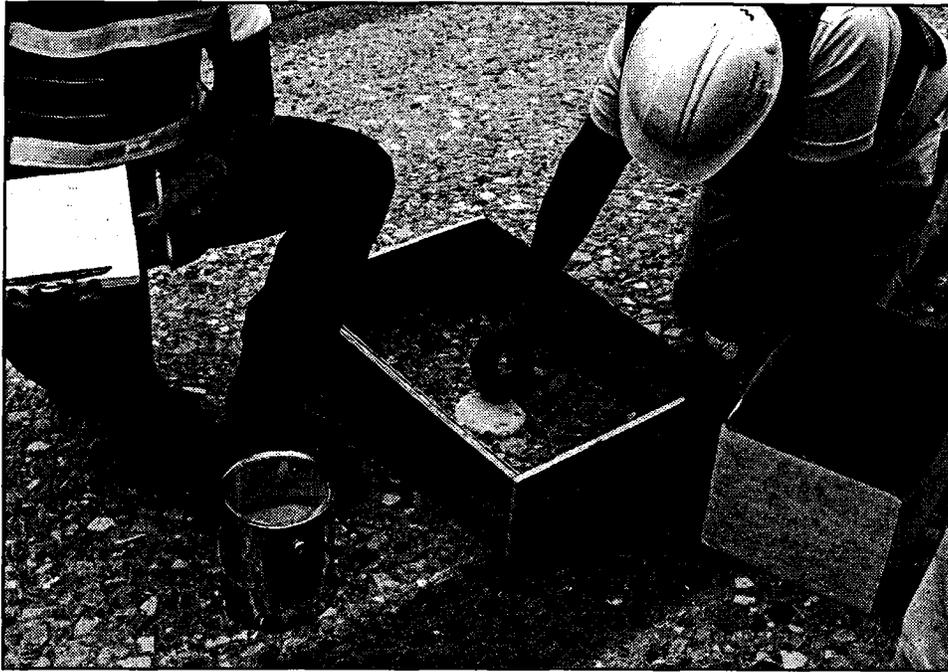
Figure 182. The deck surface must also be shotblasted to produce enough relief in the surface to provide good skid resistance. Tined surfaces usually have adequate relief and require less shotblasting. A sand patch test (ASTM E965) can be used to measure the relief in the blasted surface. A sand patch diameter of 7 in. or less (macrotexture depth of 0.04 in. or more) typically gives a good skid number.
