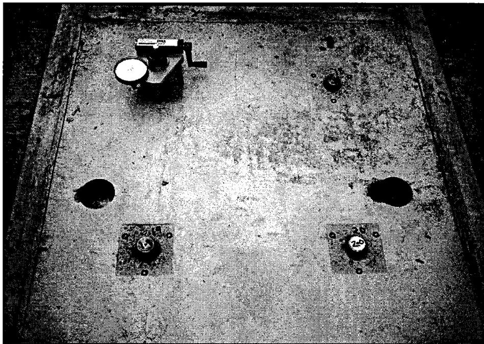
Figure 141. Tensile bond tests are here performed on an overlay test panel (VTM 92, ACI 503R). Four in. diameter cores have also been taken for rapid chloride permeability tests (AASHTO T277).
