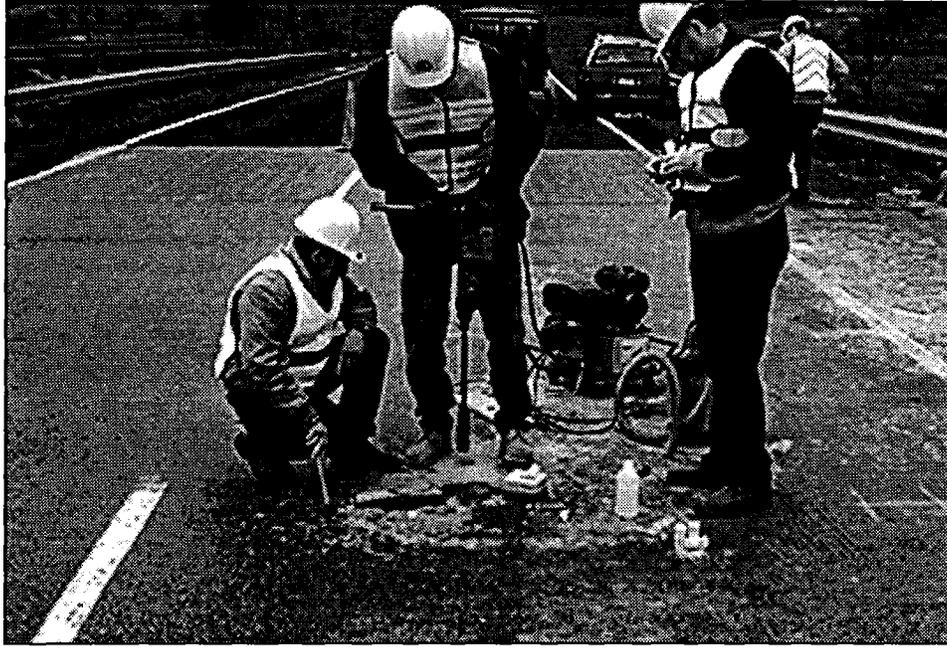
Figure 31. Chloride content measurements can be made on samples of pulverized concrete taken in the vicinity of the reinforcement. A pacometer can be used to locate and to provide an indication of the depth of cover over the reinforcement. A drill should be used to remove the concrete above the sample down to within approximately 1/2 in of the reinforcement. A vacuum can be used to remove concrete from the drill hole.
