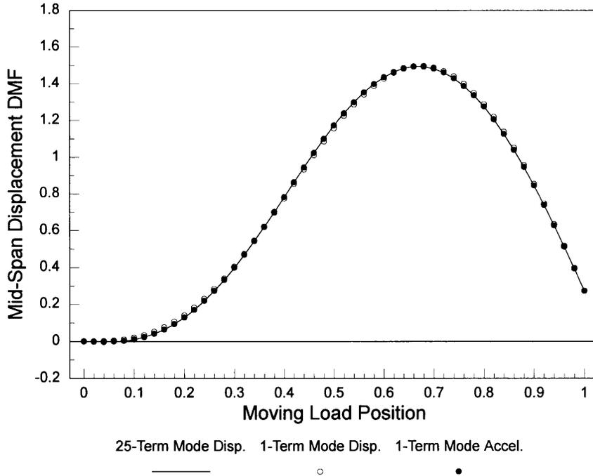
**Figure 5** Comparison of dynamic magnification factors for mid-span displacement based on 1-term and 25-term mode-displacement solutions and 1-term mode-acceleration solution.
