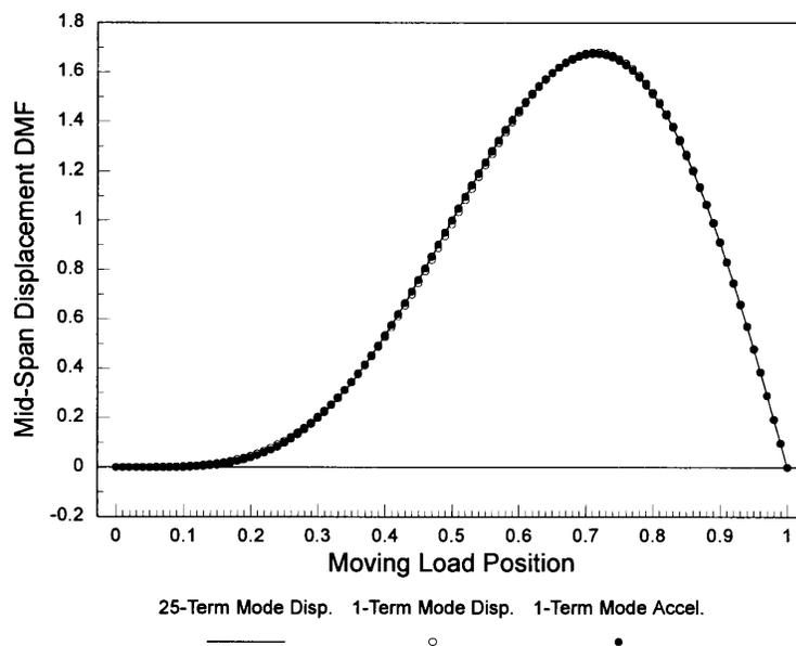
**Figure 8** Dynamic magnification factors for mid-span displacement based on 1- and 25-term mode-displacement and 1-term mode acceleration solutions ( $\gamma=0.5$ ).
