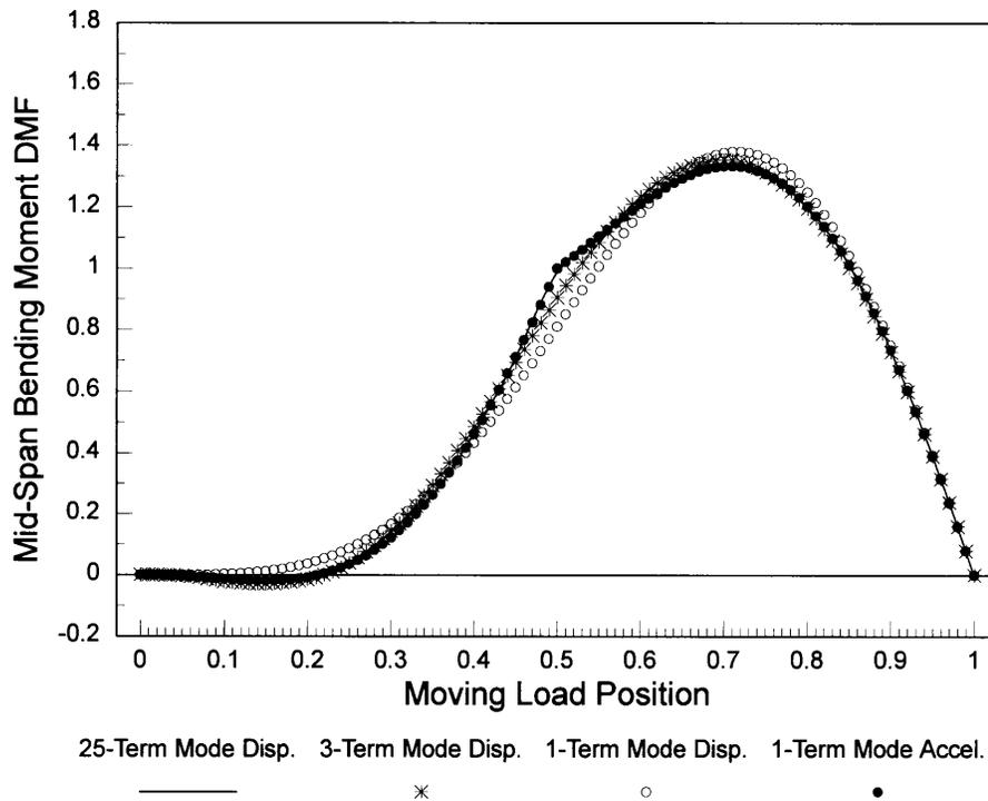
**Figure 11** Dynamic magnification factors for mid-span bending moment based on 1-, 3- and 25-term mode-displacement and 1-term mode-acceleration solutions ( $\gamma=0.5$ ).
