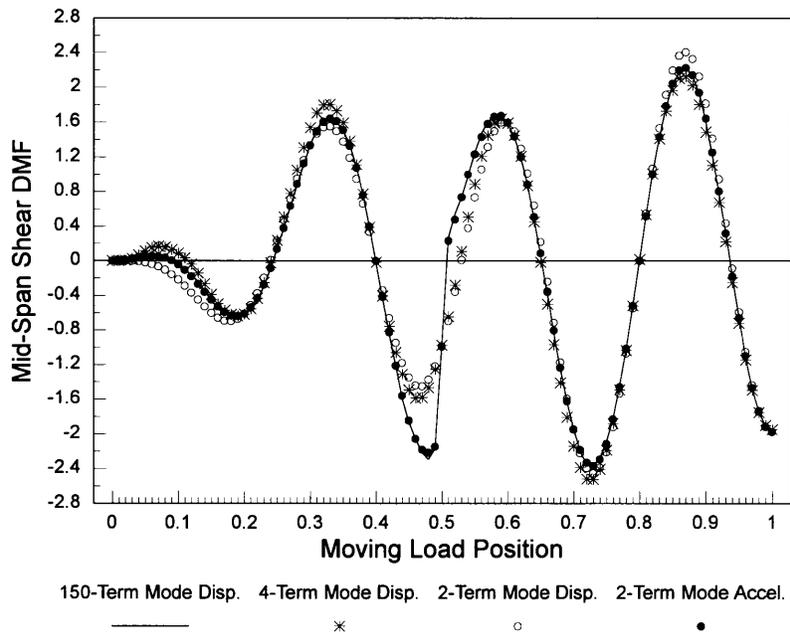
**Figure 15** Dynamic magnification factors for mid-span shear force based on 2-, 4- and 150-term mode-displacement and 2-term mode-acceleration solutions ( $\gamma=2.5$ ).
