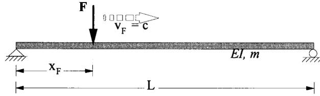
**Figure 1** Force moving across a uniform, simply-supported beam at a constant velocity,  $c$ .
