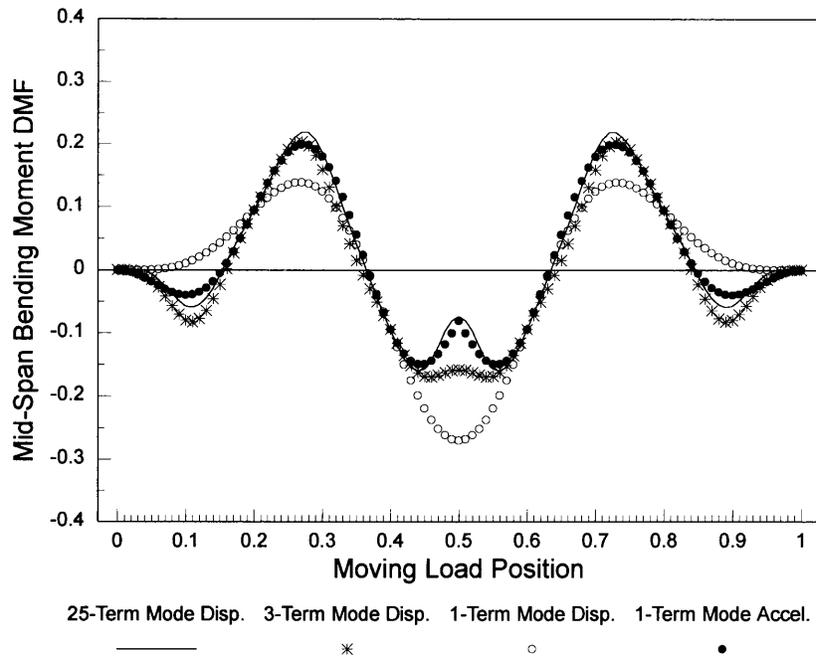
**Figure 12** Dynamic magnification factors for mid-span bending moment based on 1-, 3- and 25-term mode-displacement and 1-term mode-acceleration solutions ( $\gamma=2.5$ ).
