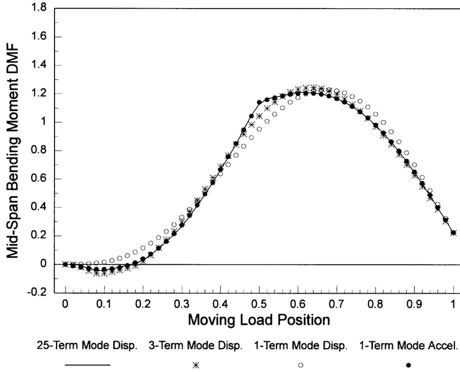
**Figure 6** Comparison of dynamic magnification factors for mid-span bending moment based on 1-term, 3-term, and 25-term mode-displacement and 1-term mode acceleration solutions.
