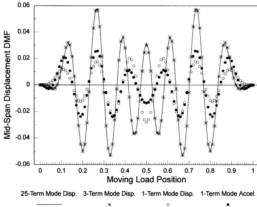
**Figure 10** Dynamic magnification factors for mid-span displacement based on 1-, 3- and 25-term mode-displacement and 1-term mode-acceleration solutions ( $\gamma=6.5$ ).
