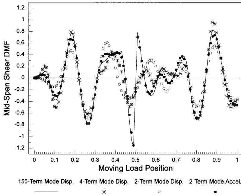
**Figure 16** Dynamic magnification factors for mid-span shear force based on 2-, 4- and 150-term mode-displacement and 2-term mode-acceleration solutions ( $\gamma=6.5$ ).
