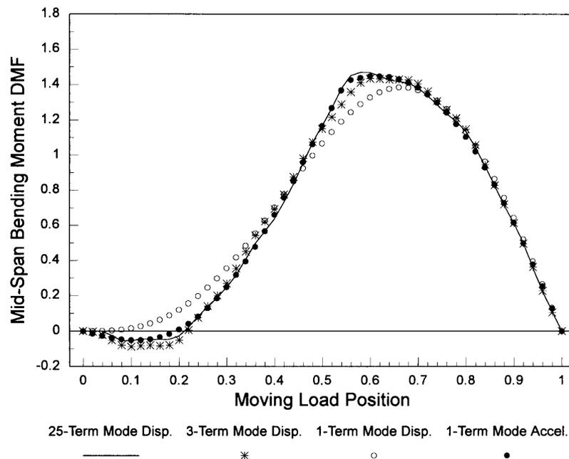
**Figure 3** Dynamic magnification factors for mid-span bending moment, 1, 3 and 25-term mode displacement & 1-term mode acceleration solutions.
