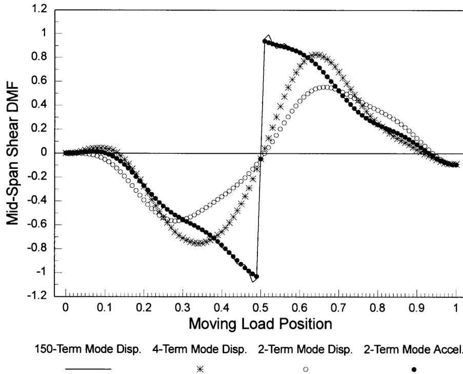
**Figure 14** Dynamic magnification factors for mid-span shear force based on 2-, 4- and 150-term mode-displacement and 2-term mode-acceleration solutions ( $\gamma=0.5$ ).
