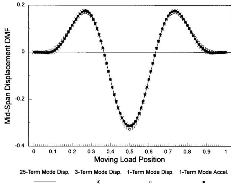
**Figure 9** Dynamic magnification factors for mid-span displacement based on 1-, 3- and 25-term mode-displacement and 1-term mode-acceleration solutions ( $\gamma=2.5$ ).
