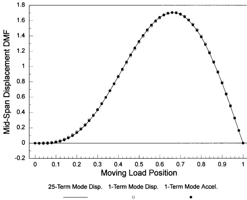
**Figure 2** Dynamic magnification factors for mid-span displacement based on 1-term and 25-term mode-displacement solutions and a 1-term mode-acceleration solution.
