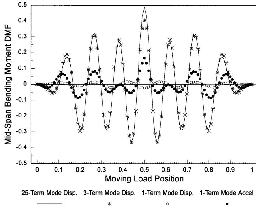
**Figure 13** Dynamic magnification factors for mid-span bending moment based on 1-, 3- and 25-term mode-displacement and 1-term mode-acceleration solutions ( $\gamma=6.5$ ).
