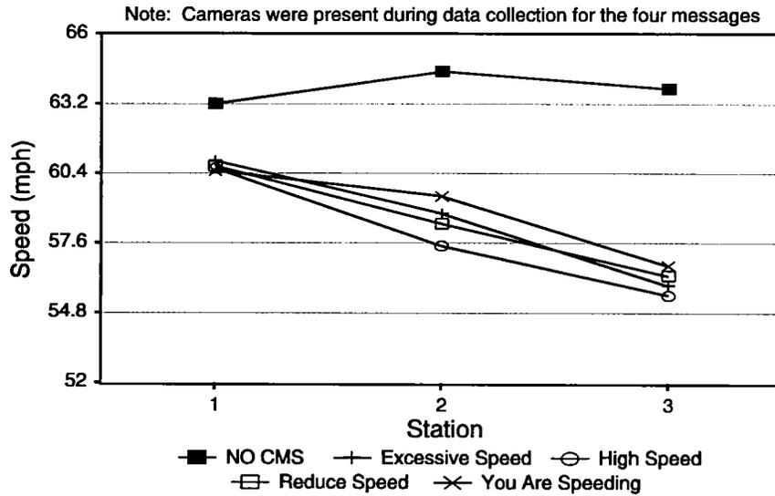
Figure 13. 85th percentile speeds (mph) -- whole population data (I-64 East Short Pump). Threshold speed limit 58 mph; posted speed limit 55 mph.
