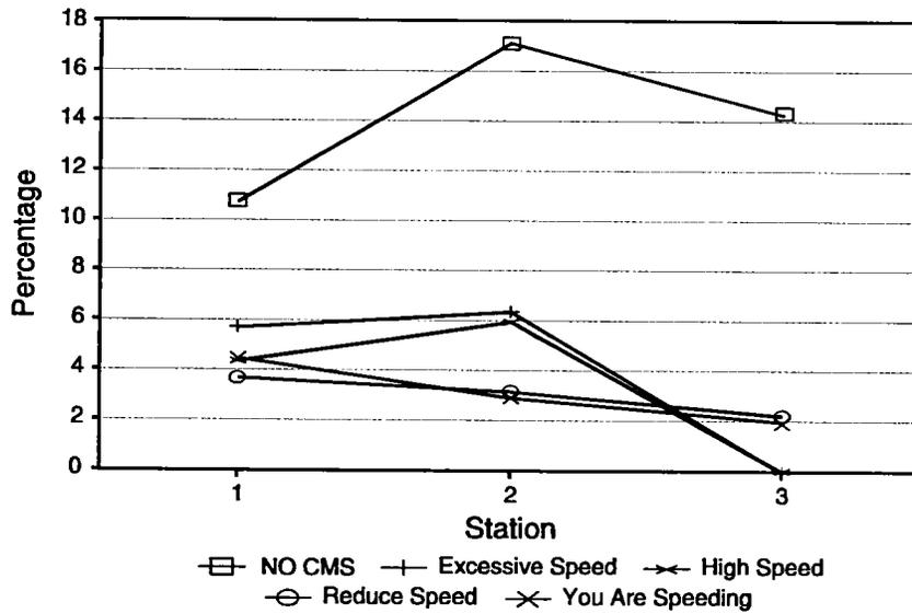
Figure 16. Percent speeding by 10 mph or more -- whole population data (I-64 East Short Pump Threshold speed limit 58 mph; posted speed limit 55 mph).
