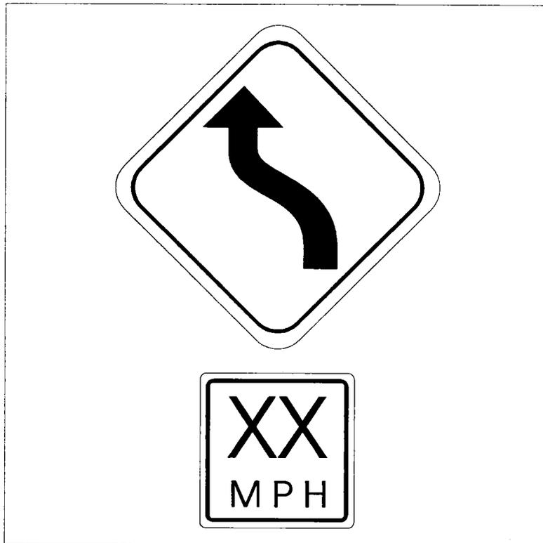
Figure 3. Advisory speed plate (W13-1) with warning sign for construction zones.
