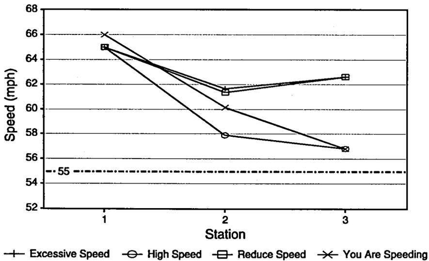
Figure 11. 85th percentile speeds (mph) -- camera data (I-64 East Shadwell). Threshold speed limit 58 mph; posted speed limit 55 mph.
