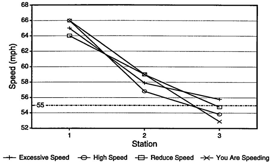
Figure 10. 85th percentile speeds (mph) -- camera data (I-81 South Buffalo Gap). Threshold speed limit 58 mph; posted speed limit 55 mph.
