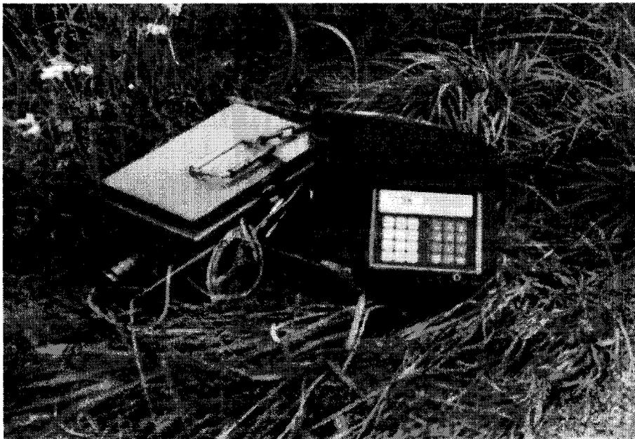
Figure 4. Traffic counter (left) with T240 programmer.
