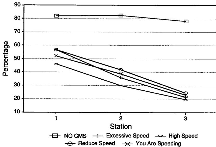
Figure 14. Percent speeding by any amount -- whole population data (I-64 East Short Pump). Threshold speed limit 58 mph; posted speed limit 55 mph.
