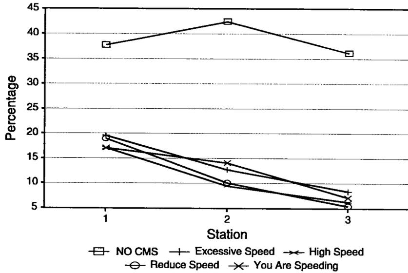
Figure 15. Percent speeding by 5 mph or more -- whole population data (I-64 East Short Pump Threshold speed limit 58 mph; posted speed limit 55 mph).
