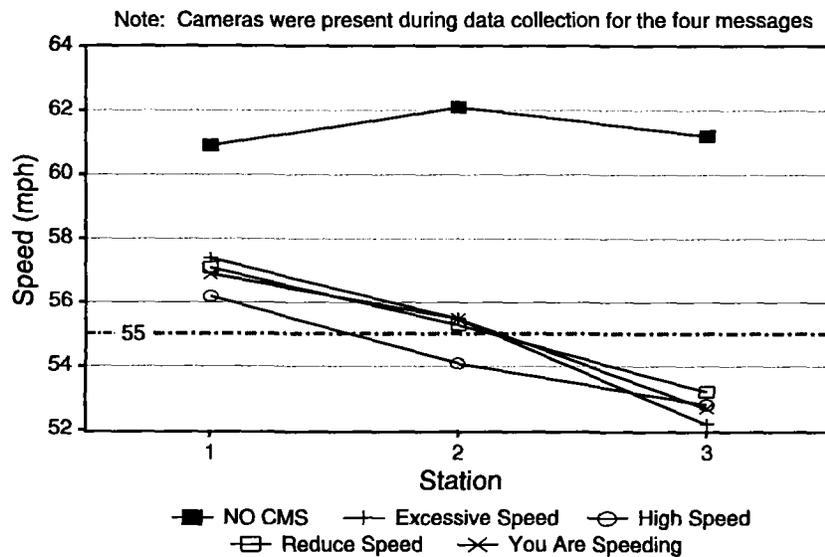
Figure 12. Average speeds (mph) -- whole population data (I-64 East Short Pump). Threshold speed limit 58 mph; posted speed limit 55 mph.
