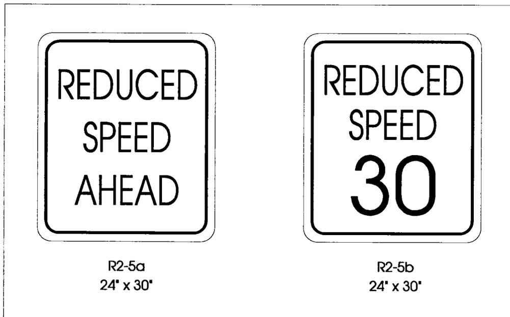
Figure 2. Standard speed limit reduction signs. (Source: MUTCD)
