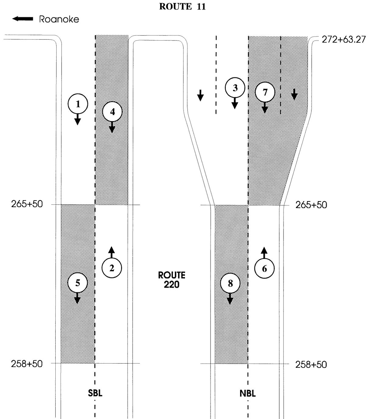
Figure 3. Paving sequence.
