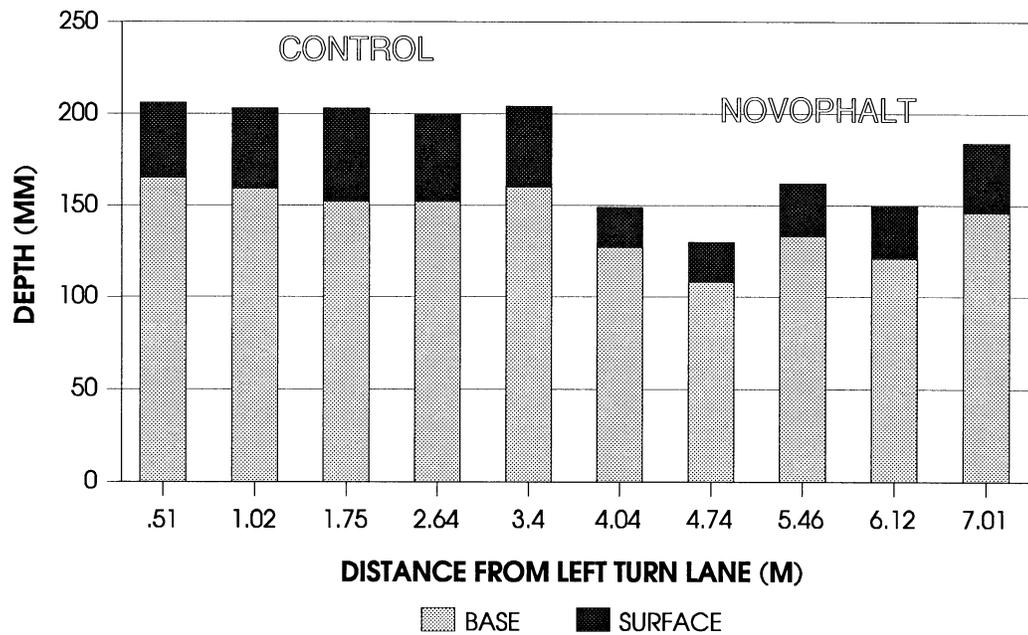
Figure 5. Thickness of cores removed in February of 1991.
