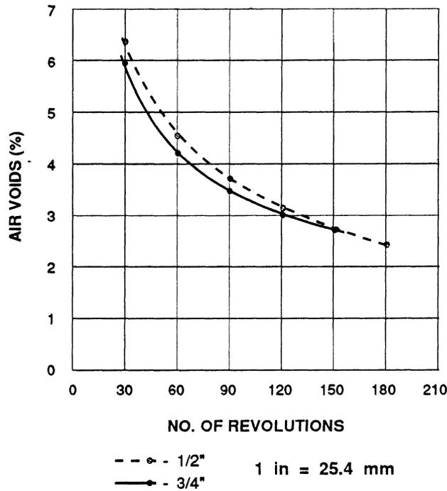
Figure 12. Air voids v. number of revolutions (quartzite,  $n = .4$ ).
