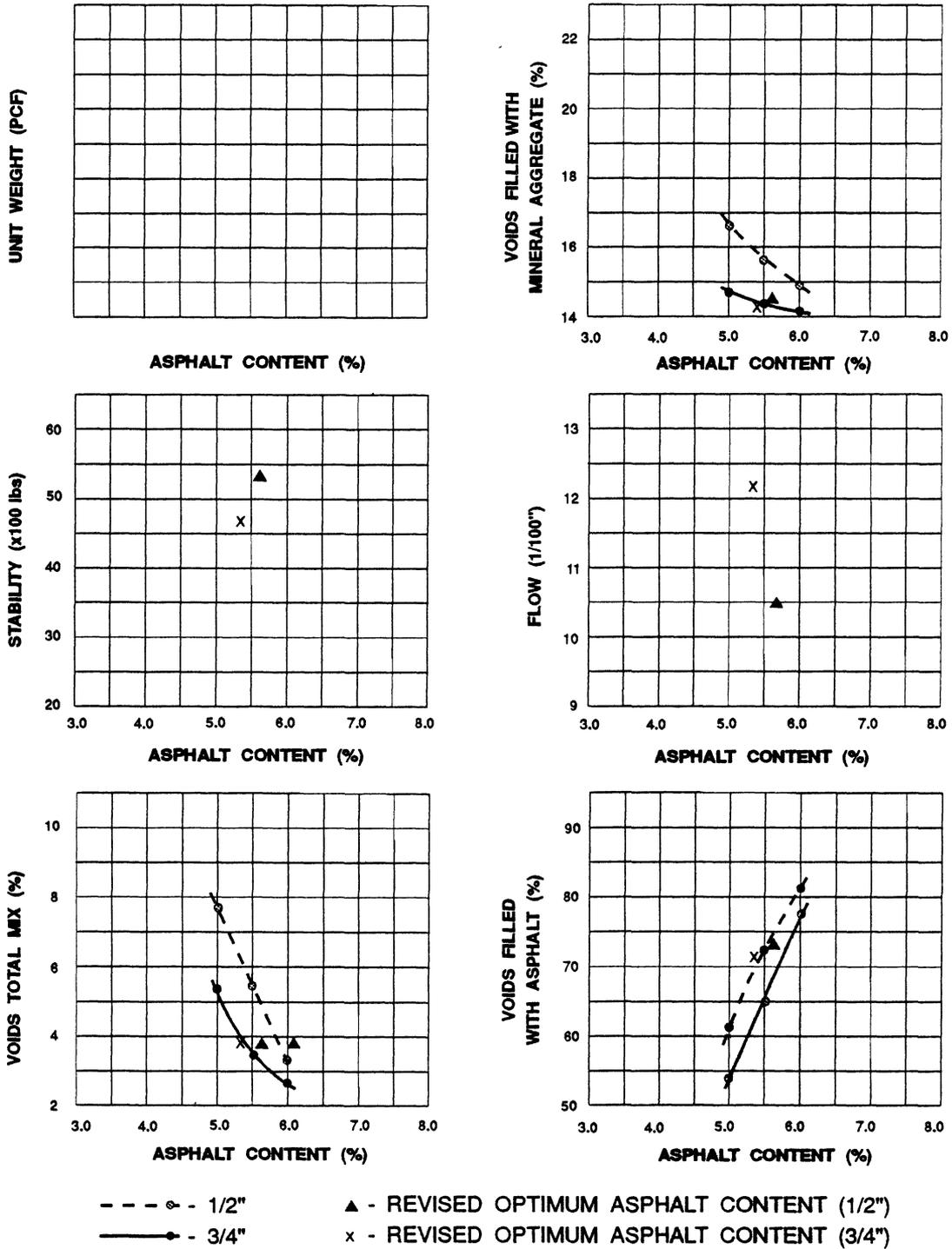
Figure 5. Mixture designs with quartzite ( $n = .4$ ).
