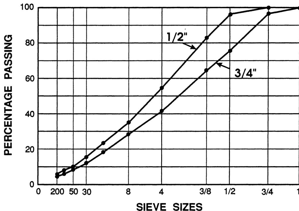
Figure 3. Gradations for  $n = .53$  (taken from ASTM) for 1/2-in (13-mm) and 3/4-in (19 mm) maximum size aggregates.
