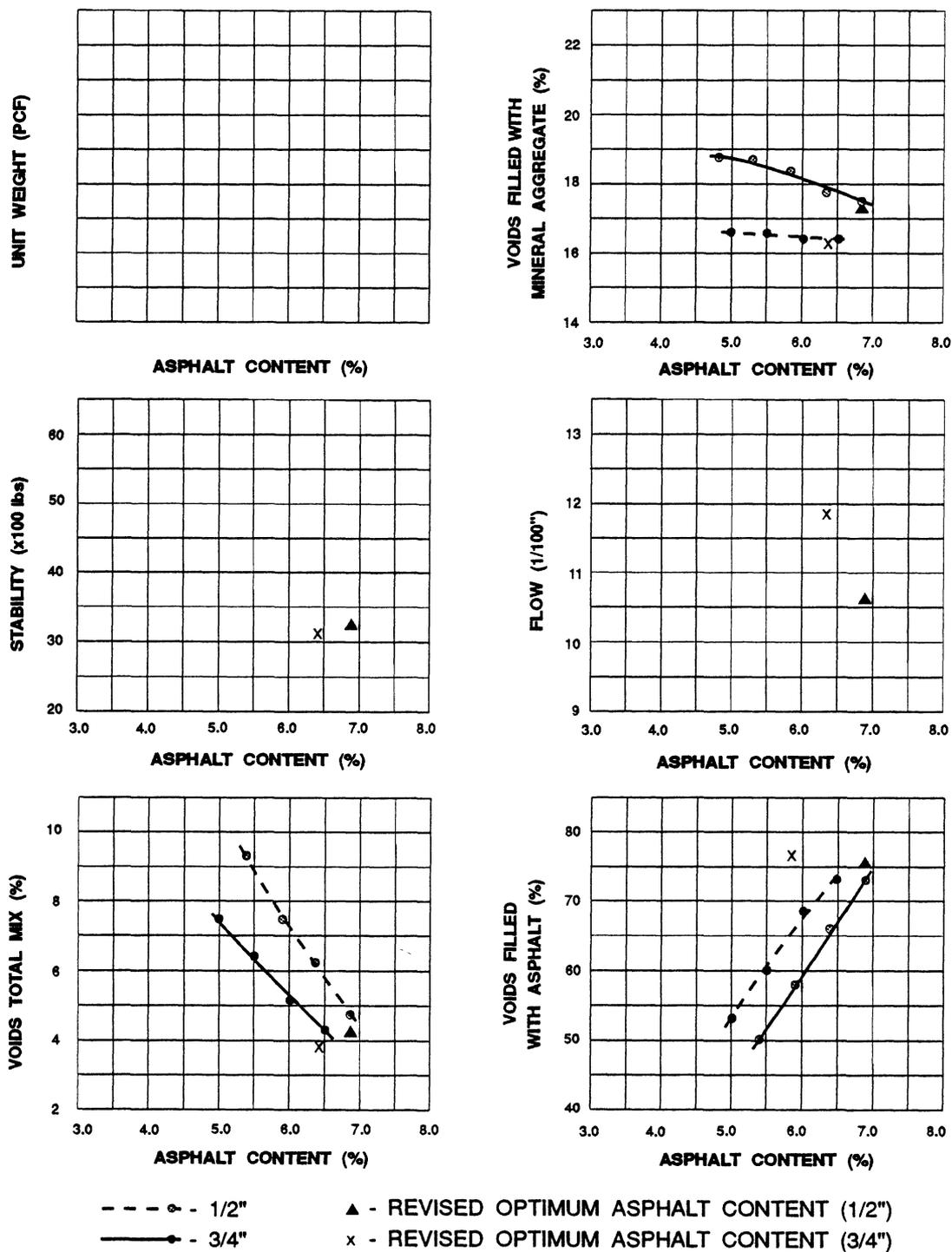
Figure 7. Mixture designs with quartzite ( $n = .6$ ).
