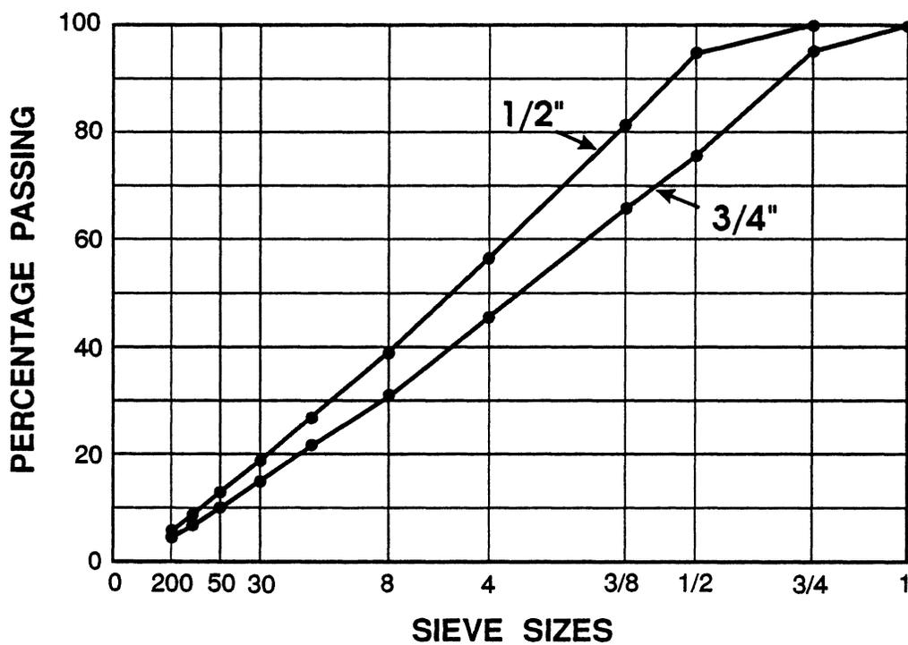
Figure 4. Gradations for  $n = .6$  for 1/2-in (13-mm) and 3/4-in (19mm) maximum size aggregates.
