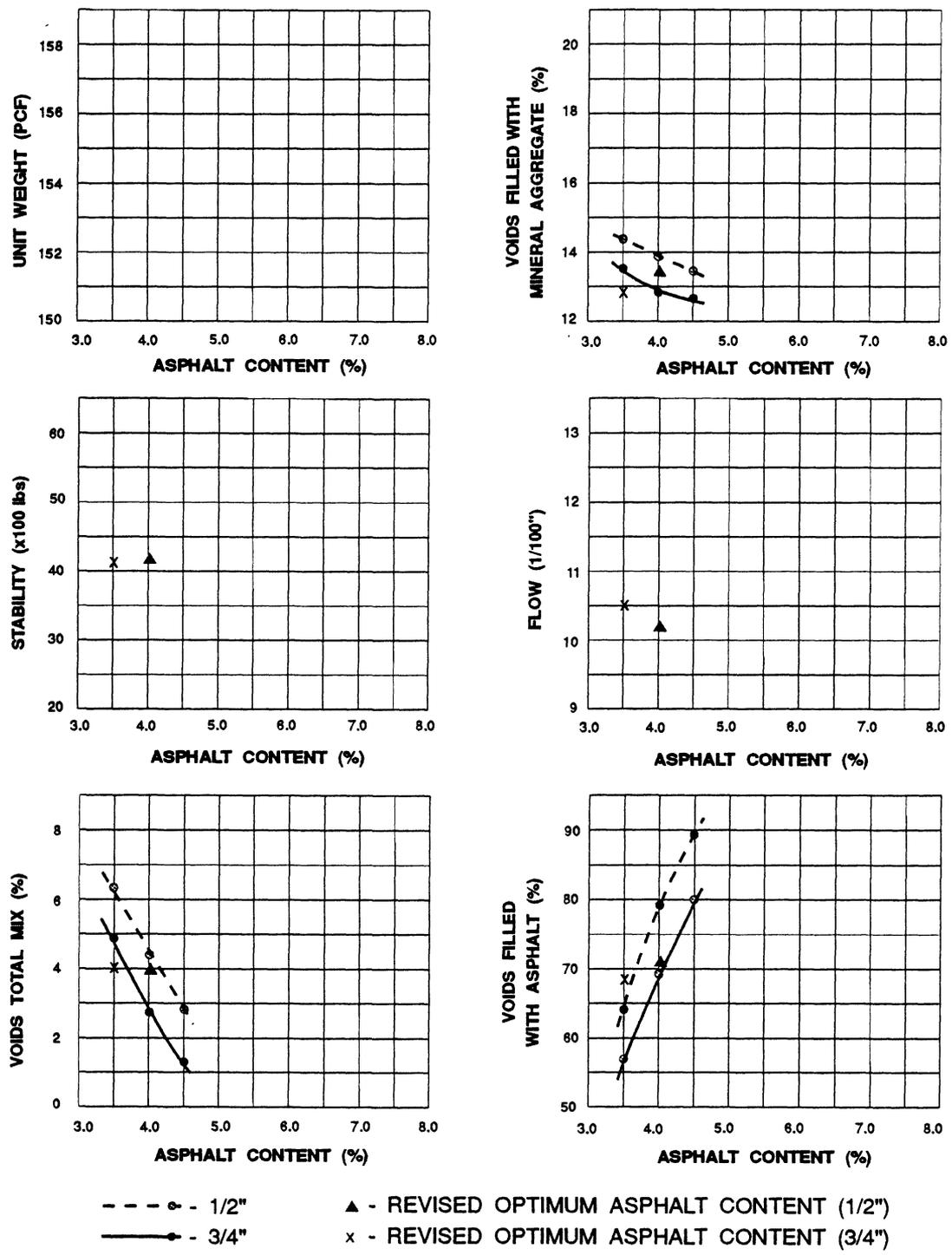
Figure 8. Mixture designs with granite (n = .4).
