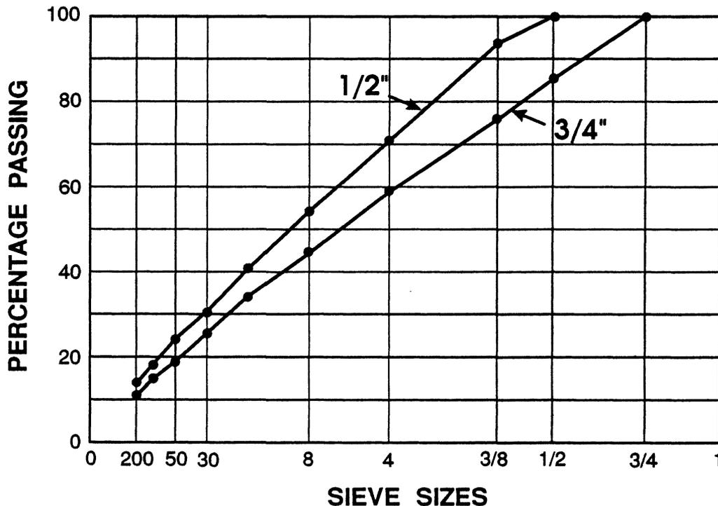
Figure 2. Gradations for  $n = .4$  for 1/2-in (13-mm) and 3/4-in (19 mm) maximum size aggregates.
