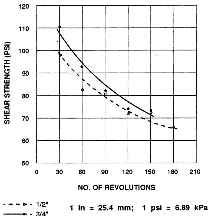
Figure 11. Shear strength v. number of revolutions (quartzite,  $n = .4$ ).
