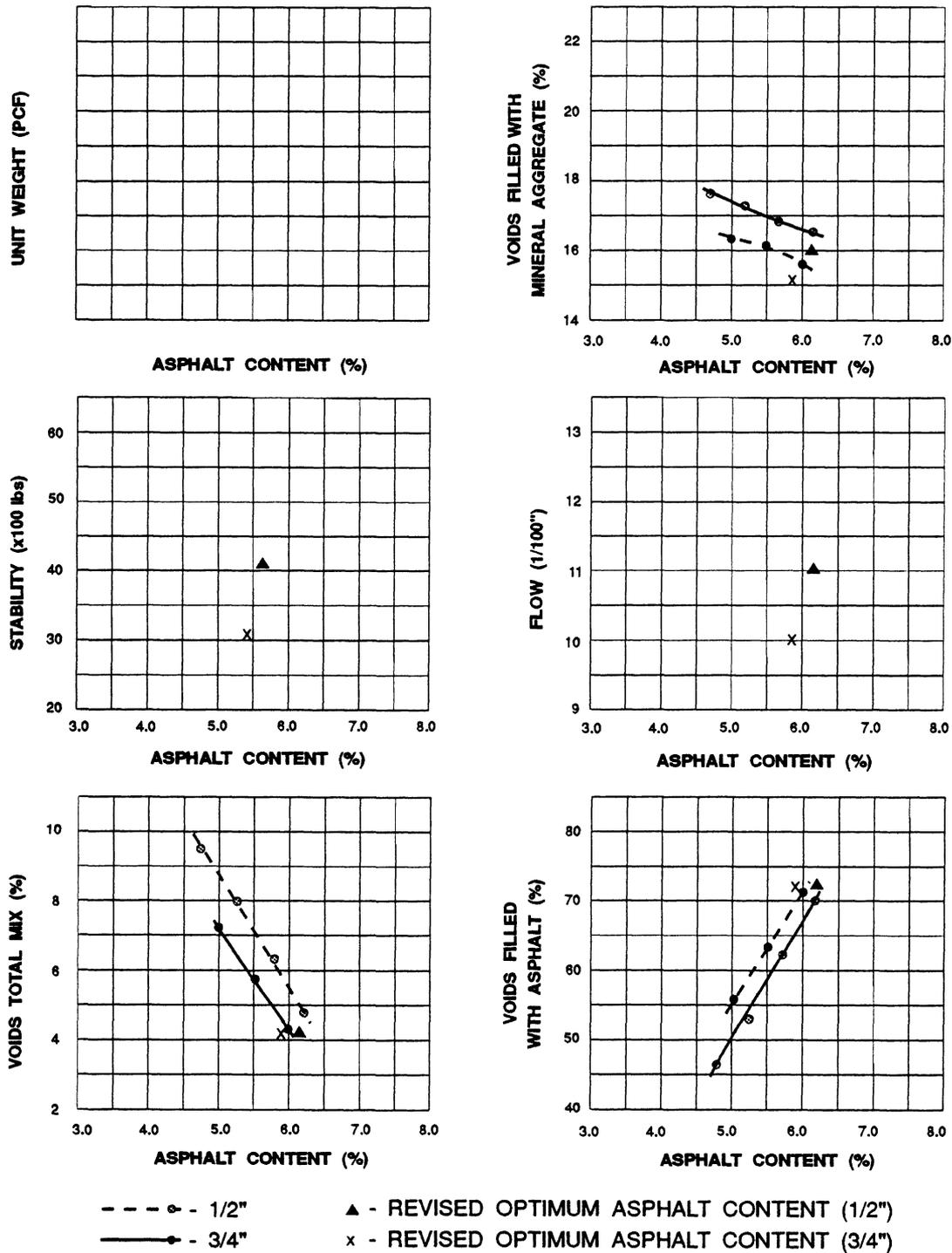
Figure 6. Mixture designs with quartzite ( $n = .53$ ).
