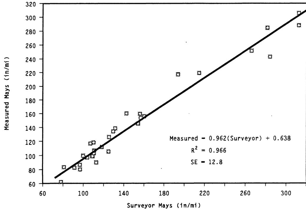
Figure 3. Mays Meter roughness v. Surveyor-predicted Mays roughness.
