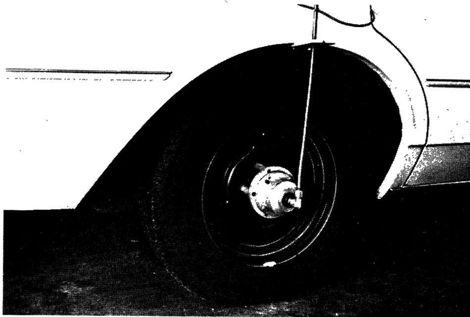
Figure 1. Distance-measuring instrumentation.
