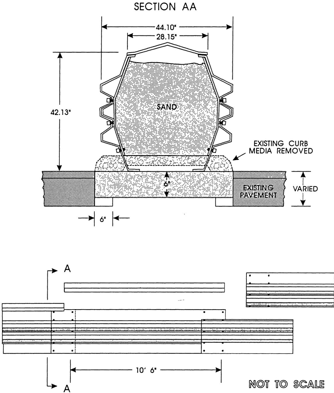
Figure 1. IBC Mark VII Median Barrier.
