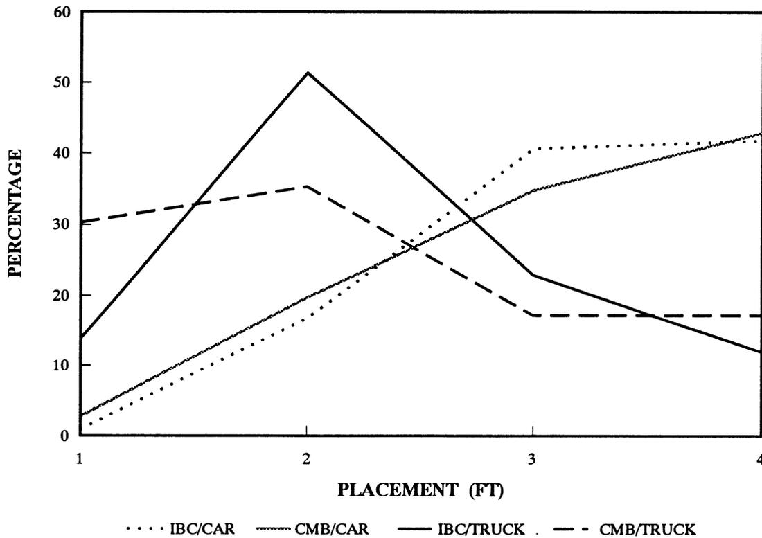
Figure 4. Lateral Placement of Uninfluenced Vehicles (NB and SB).
