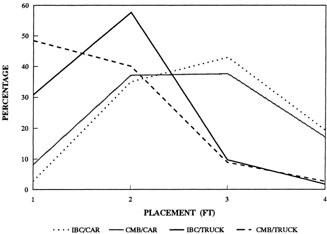
Figure 5. Lateral Placement of Influenced Vehicles (NB and SB).
