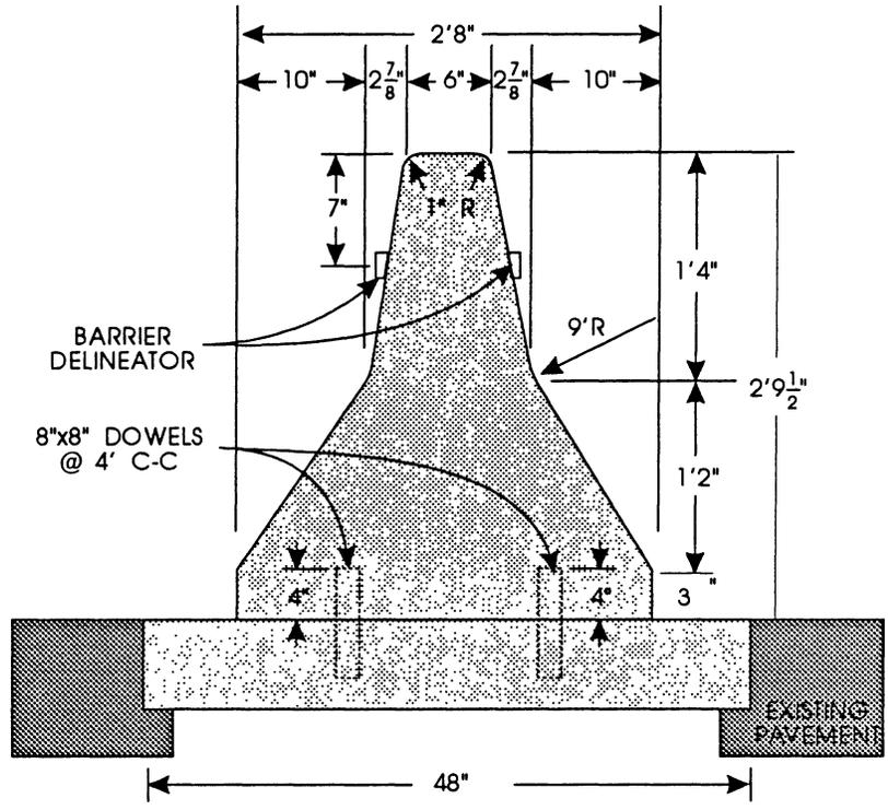
Figure 2. VDOT Standard Concrete Median Barrier (MB-7A).
