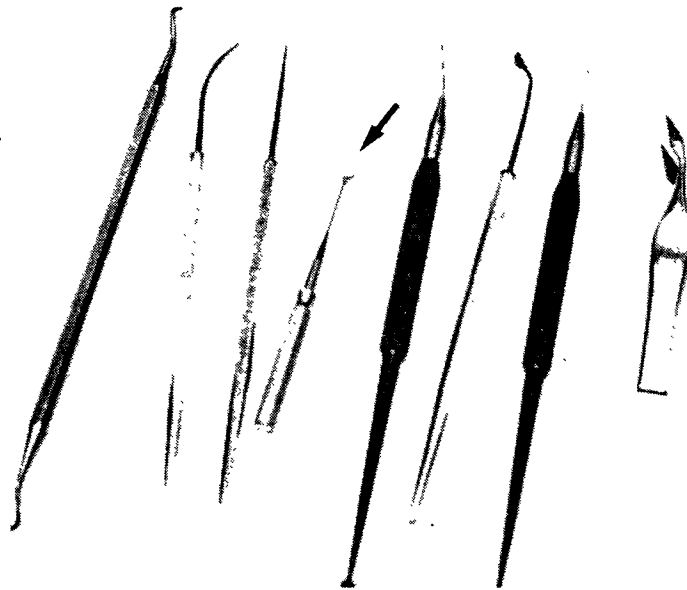
Figure 2-18 MICROTOOLS. These include needles, shovels, and scrapers small enough to be useful in the cracks and crevices of concrete and fit in the working distance under the stereomicroscope. The arrow indicates a small scale engraved on very thin, flexible metal attached to a thin rod that is attached to a handle. The scale has 5 mm marked into tenths of a millimeter on one side and 1 tenth of an inch marked into 5 thousandths of an inch on the other.
