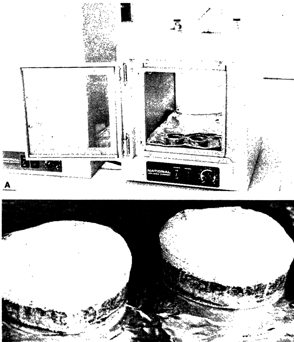
Figure 2-14 VACUUM OVEN. A. With thin-section stock in liquid dyed epoxy in a small disposable dish. Door will not stay shut without the vacuum. B. Close-up of bubbling of liquid epoxy as vacuum removes air and water from specimen.
