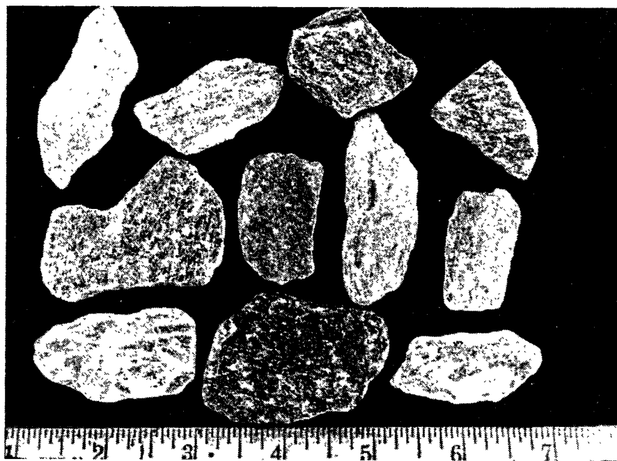
Figure E-2 AGGREGATE PARTICLES FROM FISSILE GNEISS. A particle shape such as this can cause a high water demand and popouts such as those shown in Figure E-1B.
