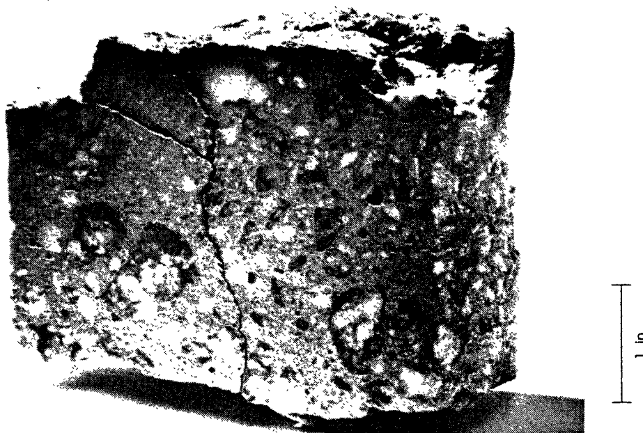
Figure 4-1 PLASTIC SHRINKAGE CRACKING. Was covered up by mortar filling over it in top of a 4-in. core. Mortar was worked into the top of this set of cracks before the concrete hardened. Later, the concrete cracked in the same area. Due to lack of interlock, the new crack follows the mortar boundaries. At the right side of the picture is a depression in the surface where a mortar plug was lost before the photograph was taken. (This specimen had to be glued together to enable the photograph to be made.)
