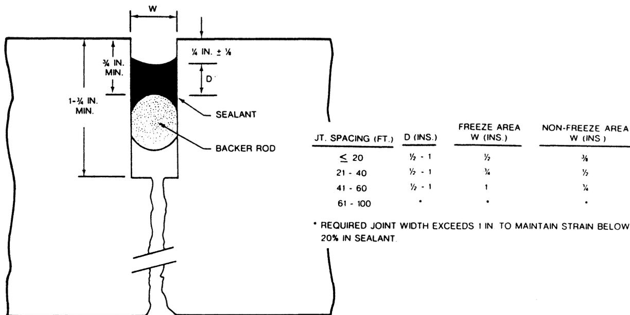
Figure 1. Recommended hot-poured sealant configurations.
