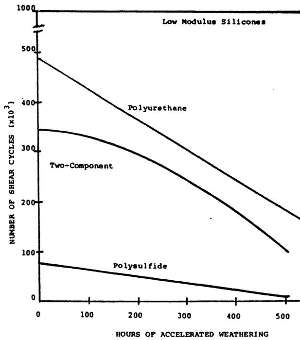
Figure 5. Effects of accelerated weathering on shear cycles.
