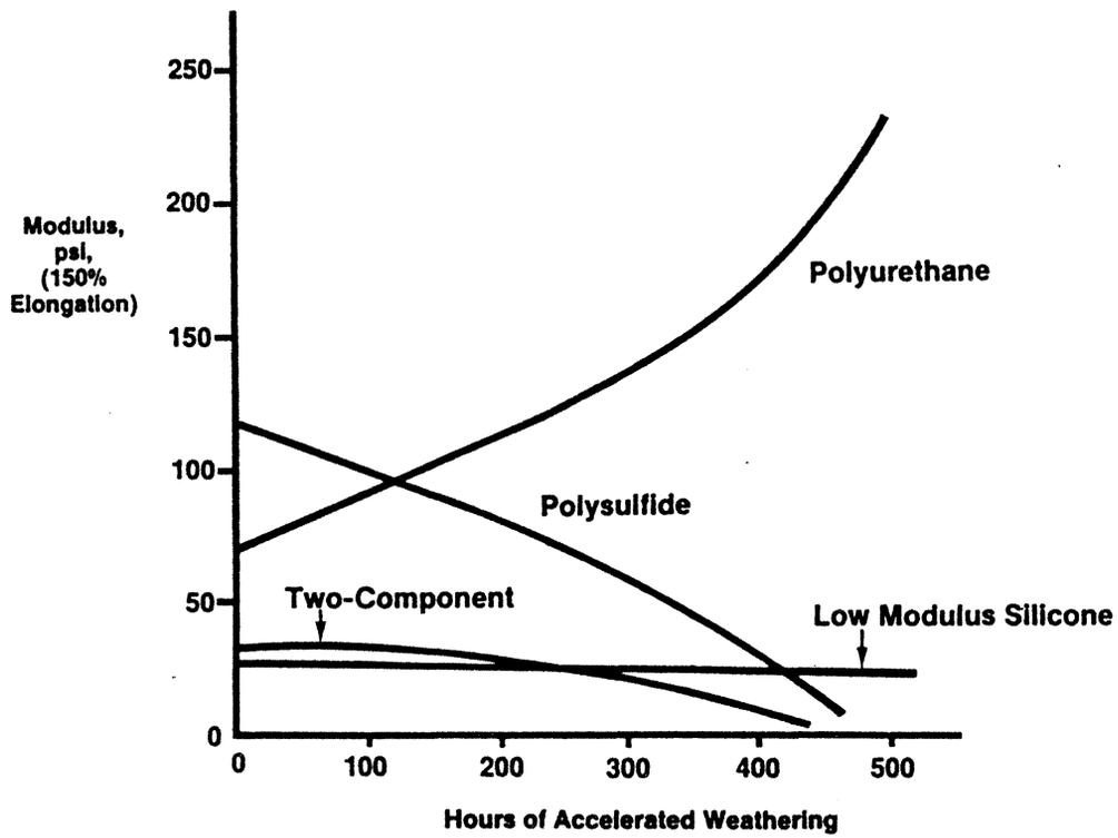
Figure 4. Effects of accelerated weathering on elastomeric properties.
