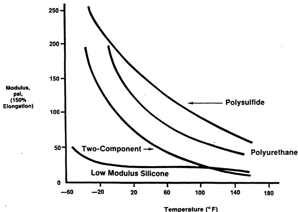
Figure 3. Effect of temperature on initial elastomeric properties.
