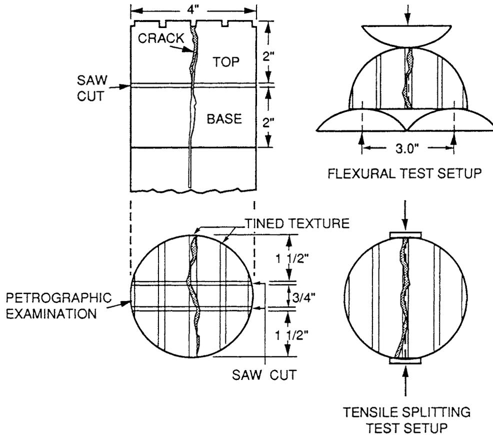
Figure 4. Sketch of test specimens obtained from cores.
