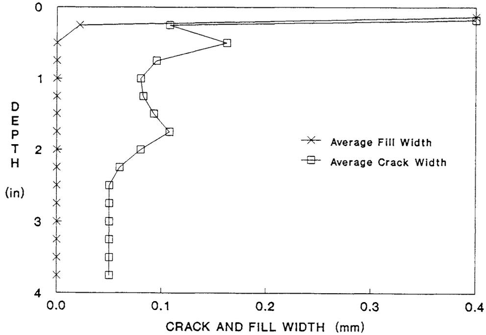
Figure 5. Average crack width and crack width filled vs. depth. Longitudinal cracks, spans 6 and 7 (T70X). At the surface, the average fill width = 0.86 mm and the average crack width = 1.15 mm.
