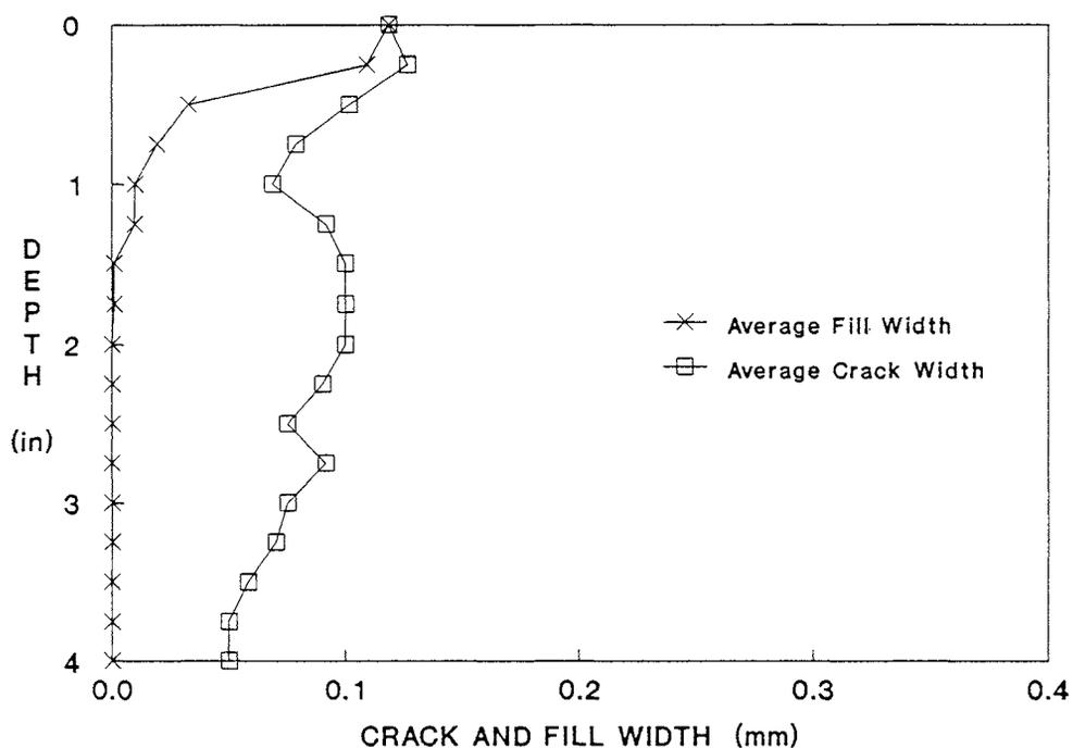
Figure 8. Average crack width and crack width filled vs. depth. All cracks, spans 8 and 9 (T70M). At the surface, the average fill width = 0.12 mm and the average crack width = 0.12 mm.
