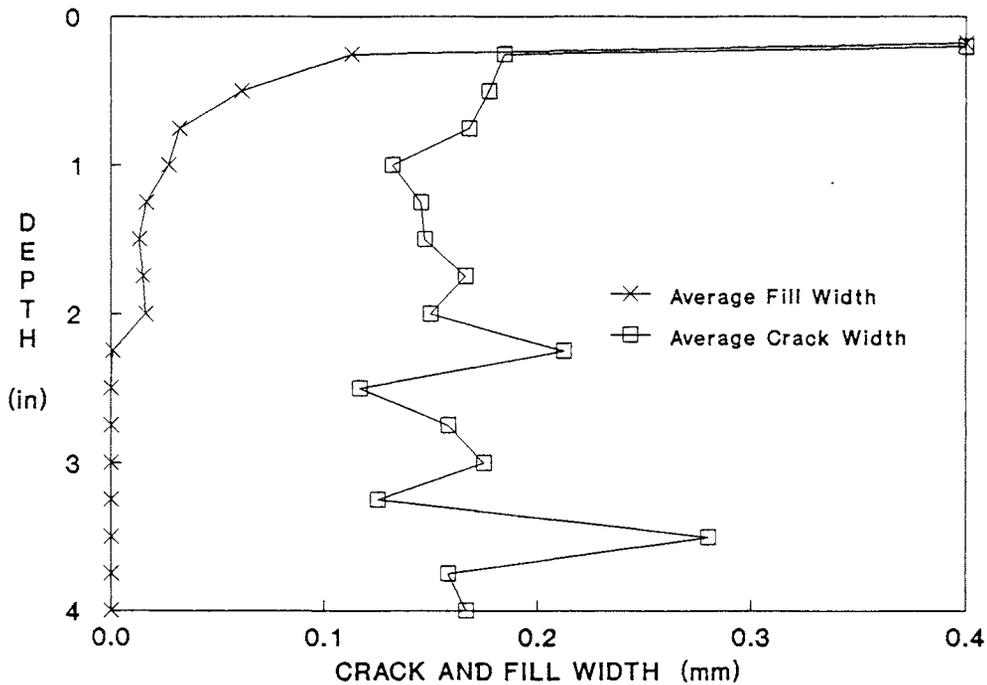
Figure 6. Average crack width and crack width filled vs. depth. All cracks, spans 6 and 7 (T70X). At the surface, the average fill width = 1.09 mm and the average crack width = 1.26 mm.
