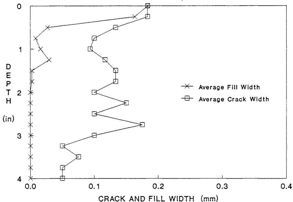
Figure 7. Average crack width and crack width filled vs. depth. Transverse cracks, span 8 (T70M). At the surface, the average fill width = 0.18 mm and the average crack width = 0.18 mm.
