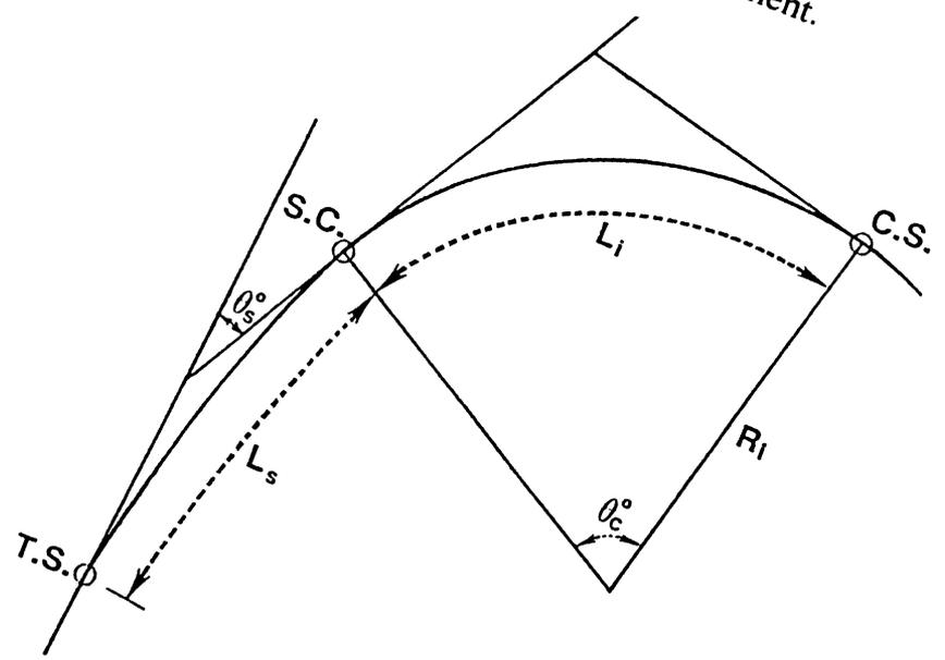
Figure 2. Components of highway horizontal alignment.
