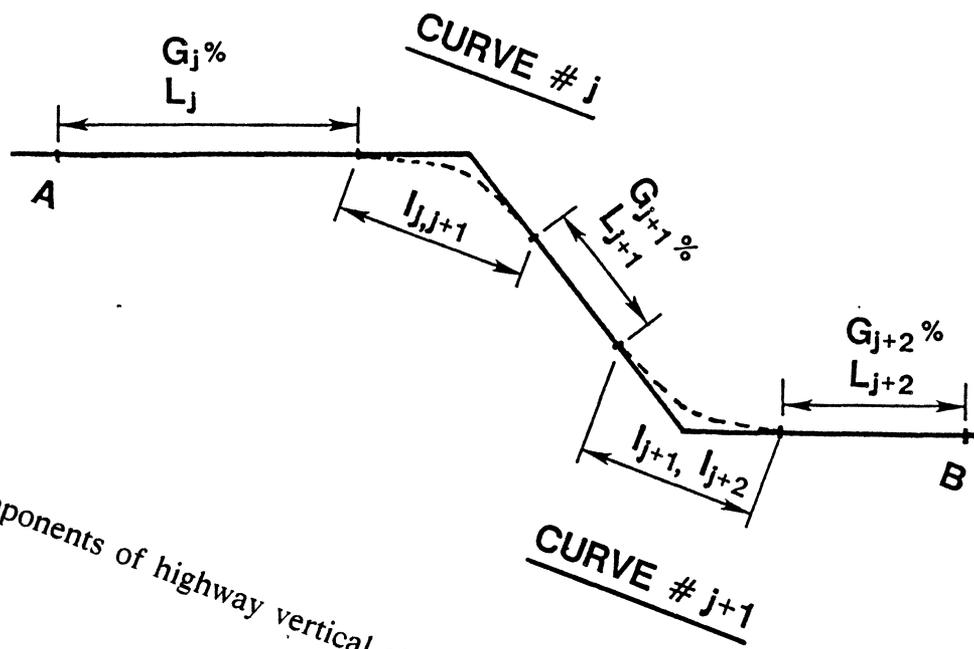
Figure 1. Components of highway vertical alignment.
