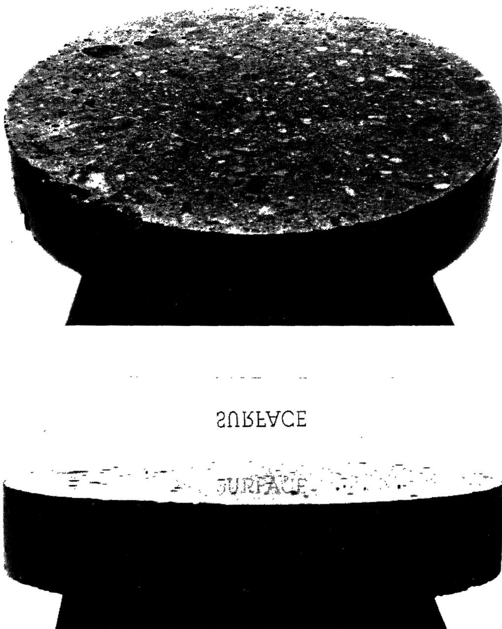
Figure 3. These photographs of the same well-prepared surface illustrate the quality of the surfaces required for microscopical examination and analyses. *A.* The surface viewed in ordinary illumination. *B.* The surface viewed at a very low angle toward a source of illumination. The quality of the reflection of a distant object (here, the quality of the reflection of the reversed word "SURFACE" on the screen) indicates the flatness of the lapped surface.
