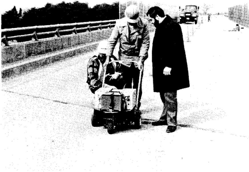
Figure 5. A delamect can be rolled over the deck surface to produce a strip chart that can be examined to identify delaminated areas.
