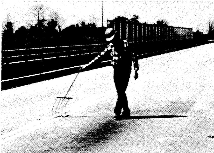
Figure 4. Several chains hanging from a pipe (chain drag) can be dragged over the deck surface to locate delaminated and very unsound concrete. The chain produces a hollow sound when it passes over delaminated concrete.
