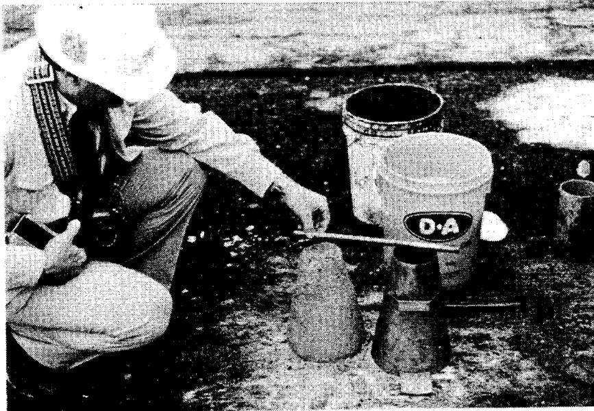
Figure 29. A slump test (ASTM C143) can provide an indication of the workability of hydraulic cement concrete. The temperature and the air content of the concrete should also be measured and recorded.
