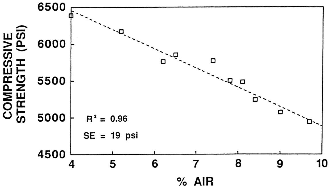
Figure 4. Relationship between the air content measured by a Type A pressure meter and the 28-day compressive strength.
