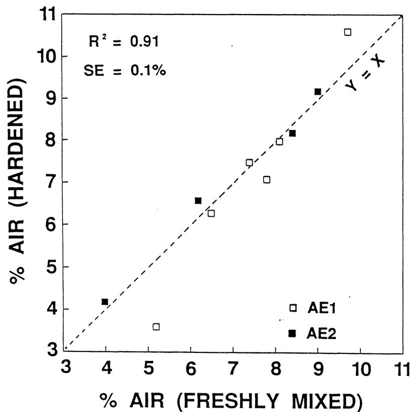
Figure 2. Comparison of the air content of laboratory concretes determined with a Type A pressure meter in the fresh stage with that determined microscopically in the hardened stage.
