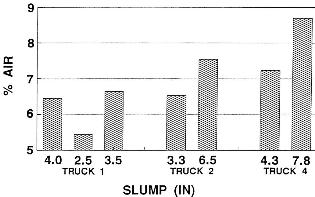
Figure 6. Air content and slump after the addition of water.
