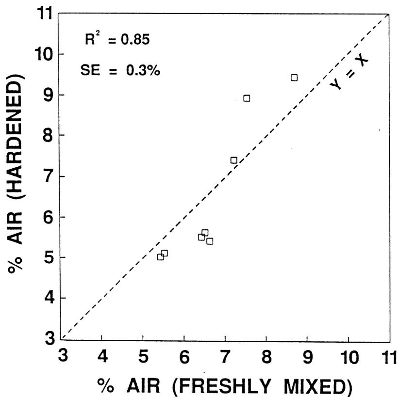
Figure 5. Comparison of air content of concretes from Plant 1 determined with a Type A pressure meter in the fresh stage with that determined microscopically in the hardened stage.
