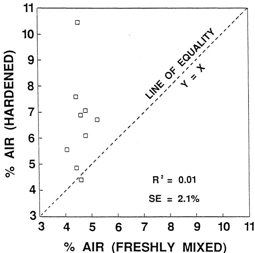
Figure 1. Comparison of the air content of field concretes determined with pressure meters in the fresh stage and determined microscopically in the hardened stage.
