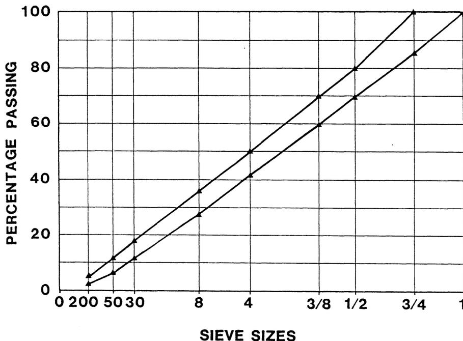
Figure 1. Master gradation band for experimental mixes.
