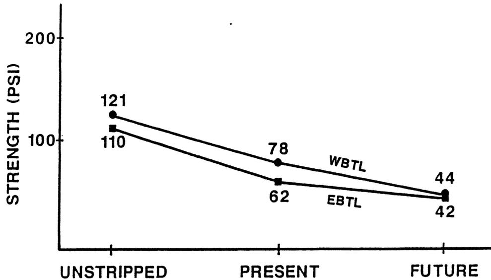
Figure 6. Deterioration curves for B-3 mix on I-64.
