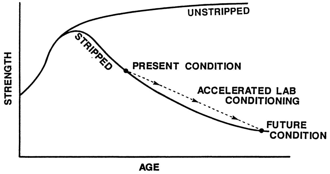
Figure 2b. Development of deterioration curve (present and future conditions).
