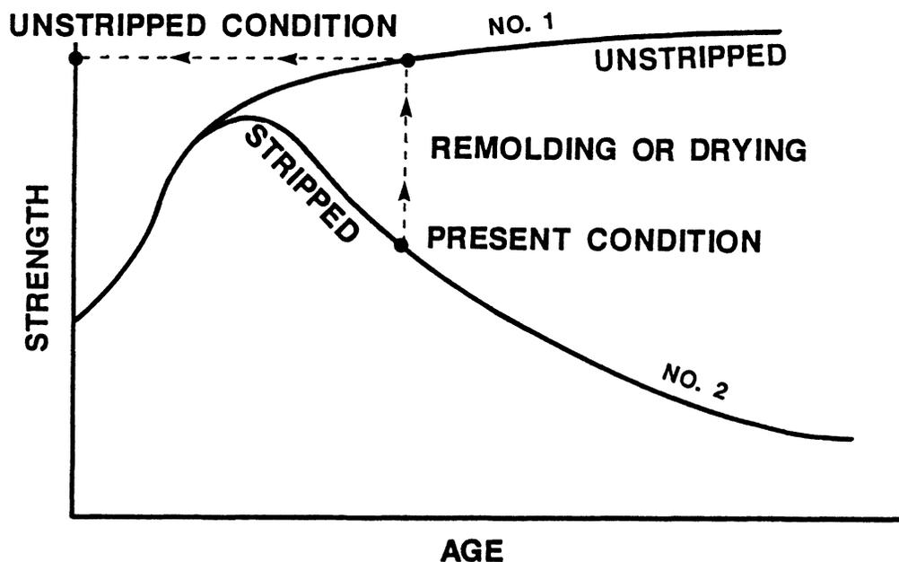
Figure 2a. Development of deterioration curve (present and unstripped conditions).
