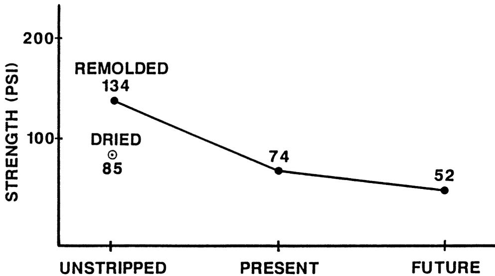
Figure 7. Deterioration curve for Greenwood Drive.
