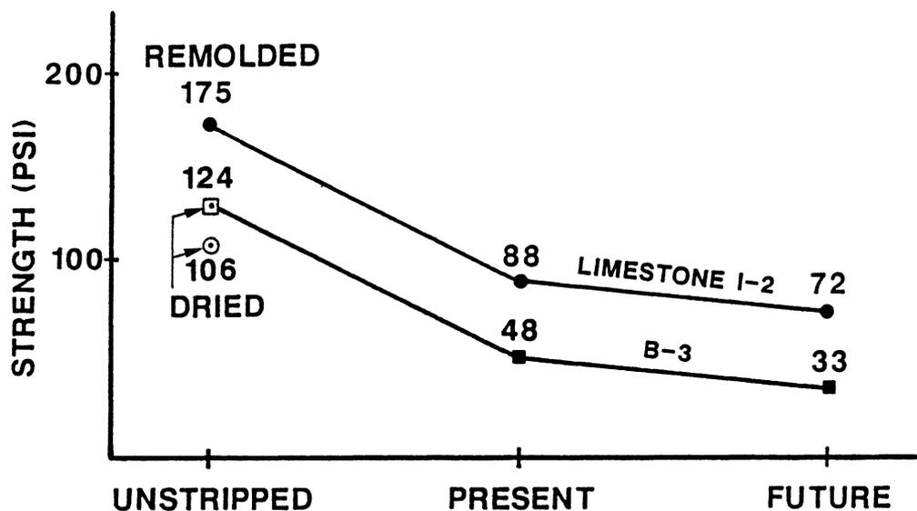
Figure 4. Deterioration curves for I-81.
