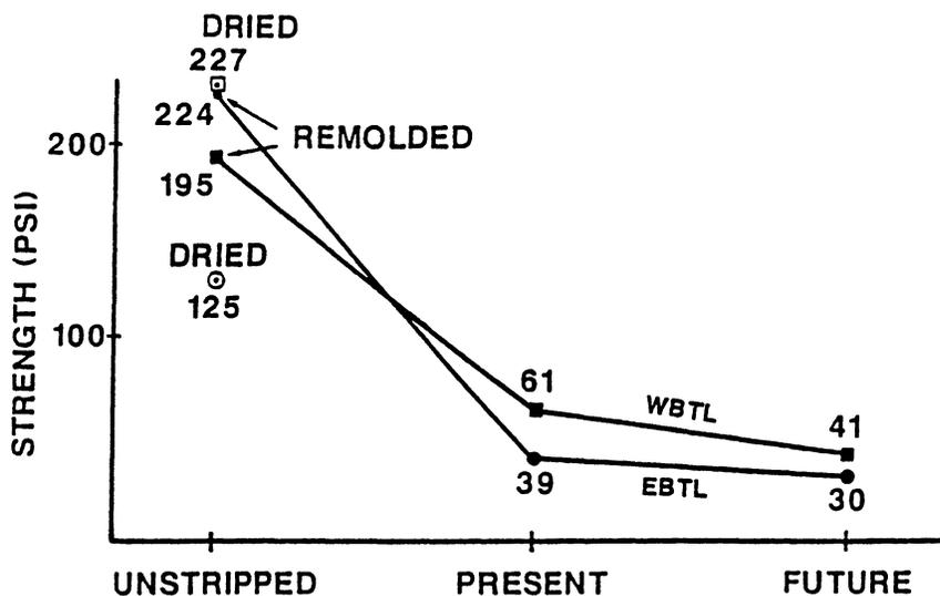
Figure 5. Deterioration curves for I-2 mix on I-64.
