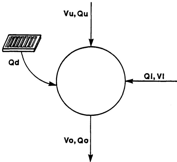
Figure 1. Flow at a manhole.
