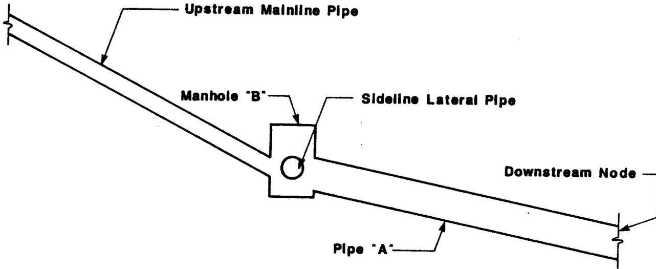
Figure 10. Schematic of computational pipe-node element in hydraulic gradeline computation.
