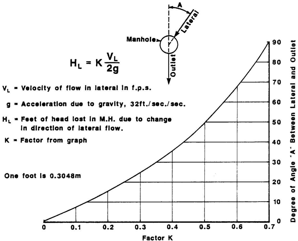
Figure 2. Loss coefficient due to change in direction of flow (after FHWA-TS-79-225),
