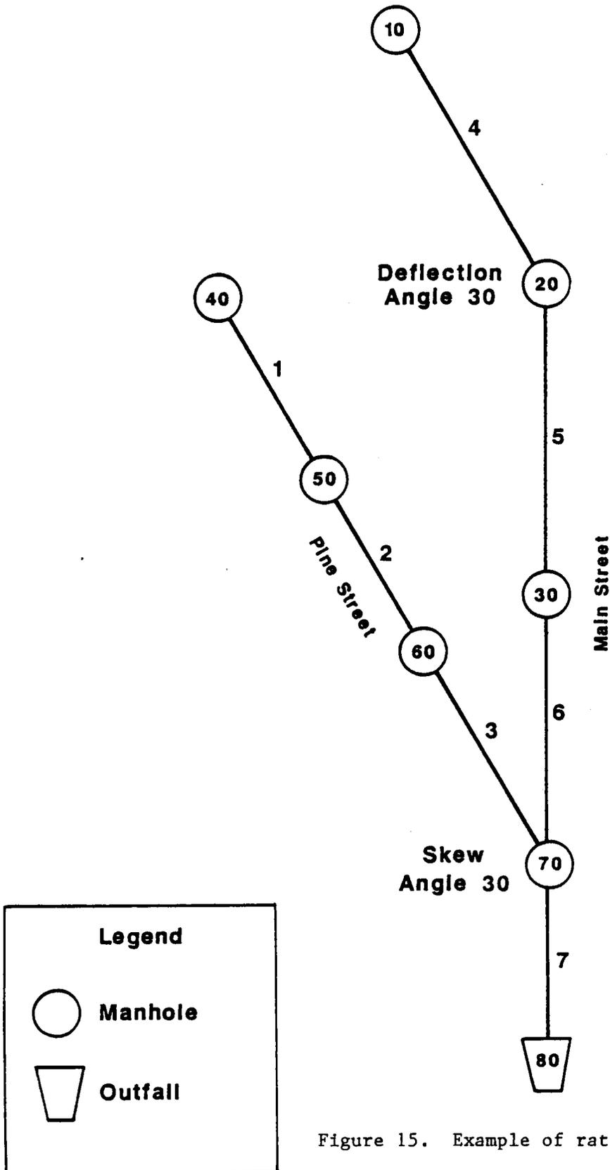
Figure 15. Example of rational method design.
