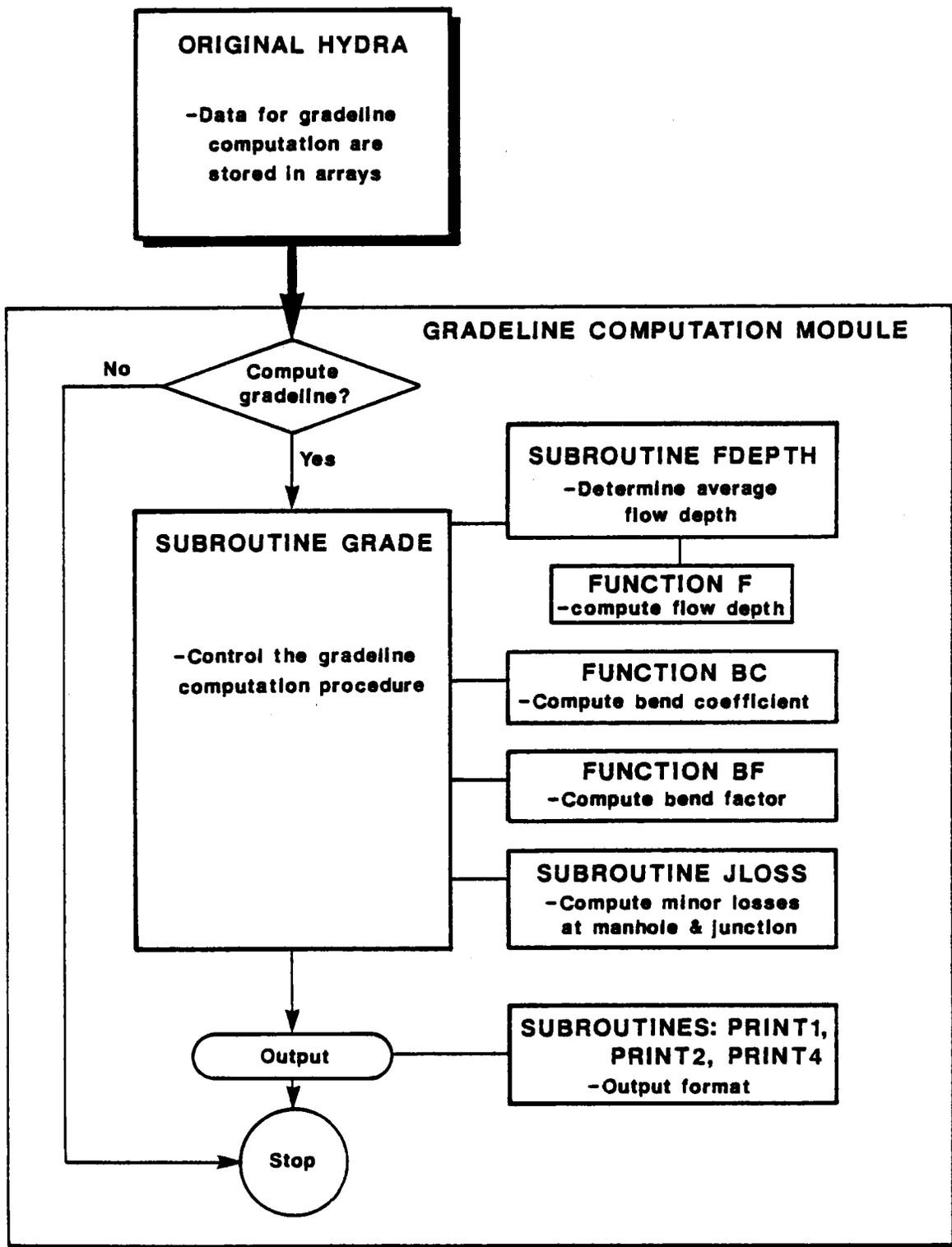
Figure 9. Flow chart of the modified HYDRA.
