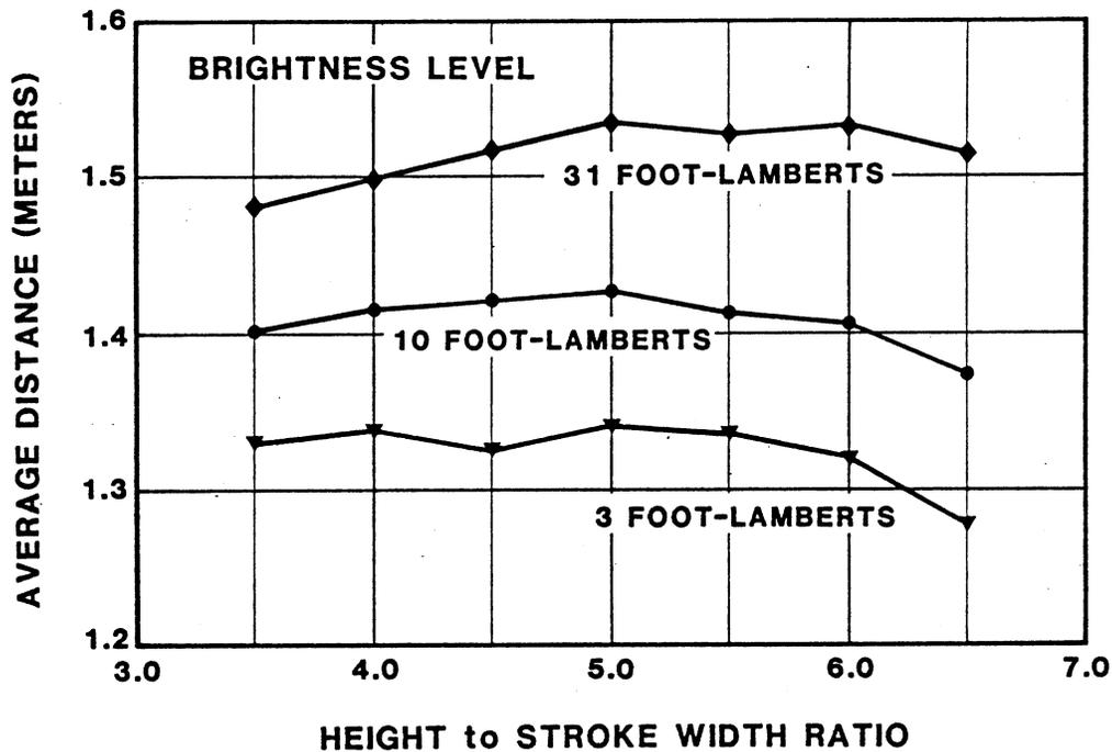
Figure 10. Average legibility distance for numerals as a function of height stroke-width ratio and brightness.
