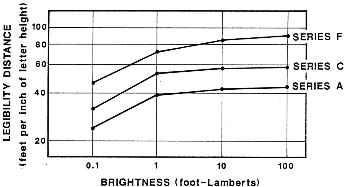
Figure 1. Brightness vs. legibility for different letter series.
