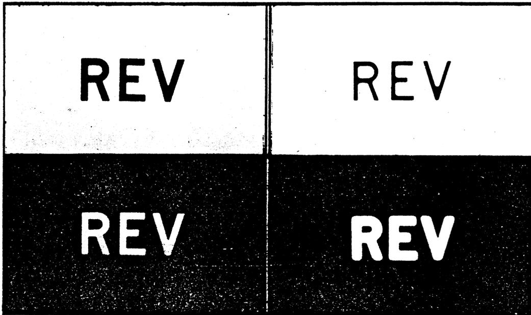
Figure 2. Appearance of signs of optimum and high brightness.
