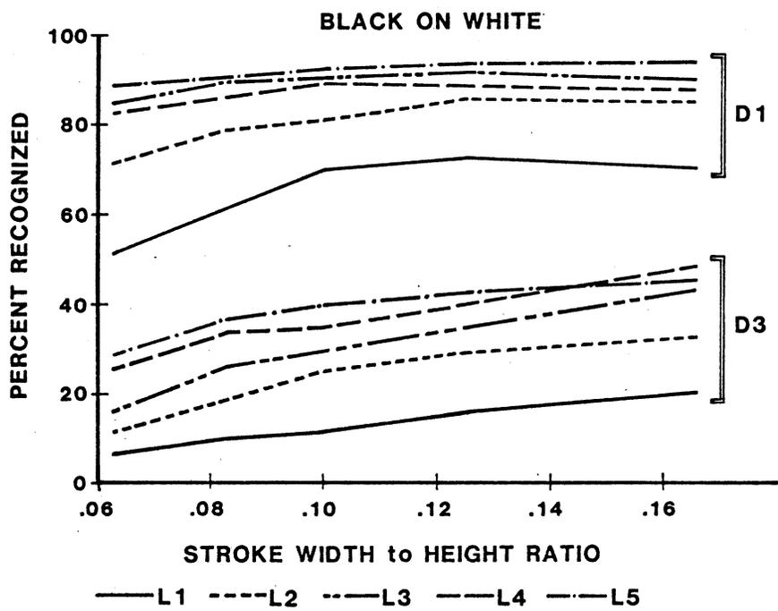
Figure 11. Illustration of the effects of distance, luminance and strobewidth/height ratio on recognition of black numerals.
