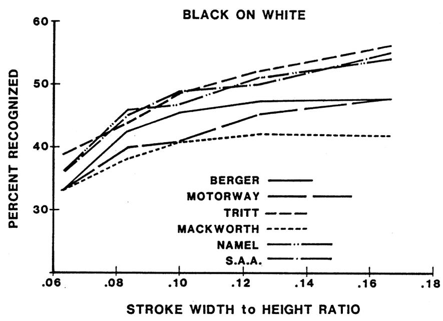
Figure 12. The effect of font and strobewidth/height ratio on the percentage of black numerals recognized.
