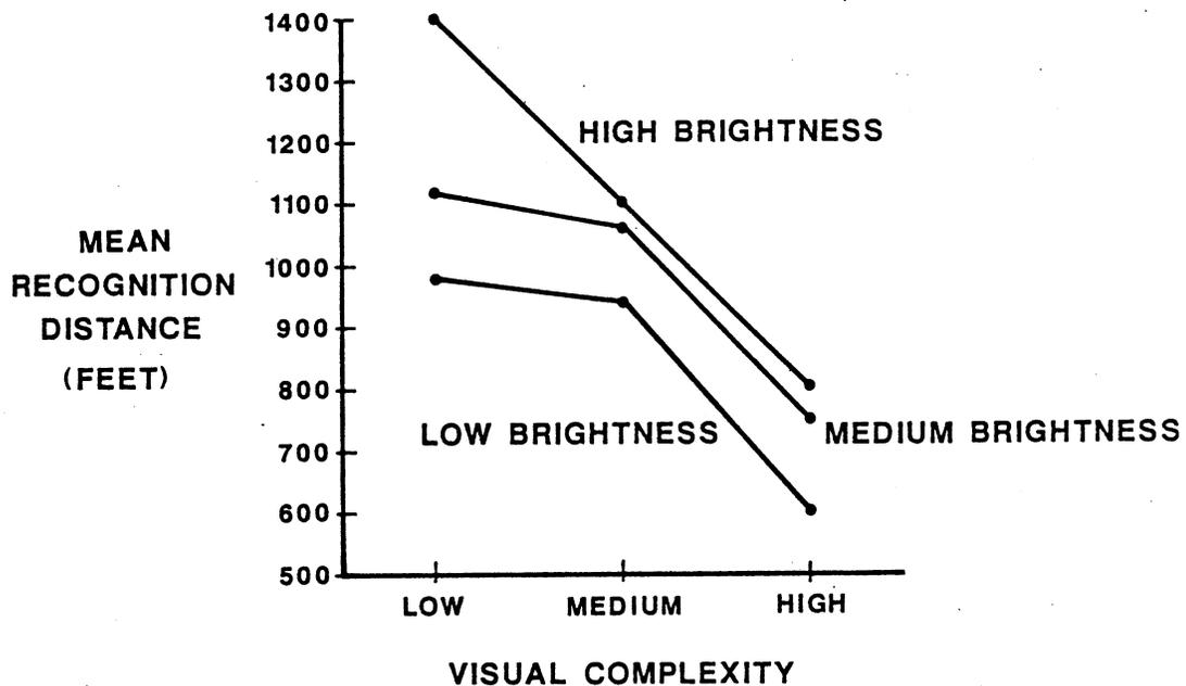
Figure 3. Recognition performance by visual complexity and sign brightness.
