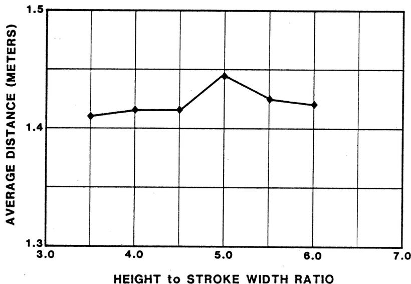
Figure 9. Average legibility distance for numerals as a function of height/stroke-width ratio and background.
