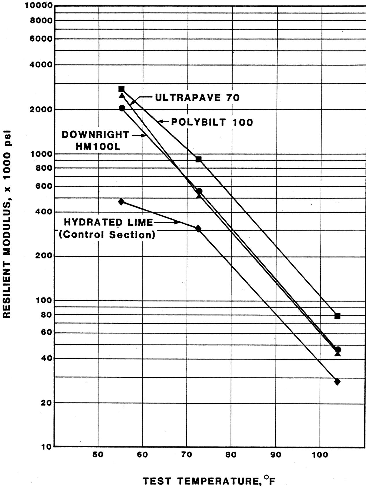
Figure 2b. Resilient modulus vs. test temperature.
