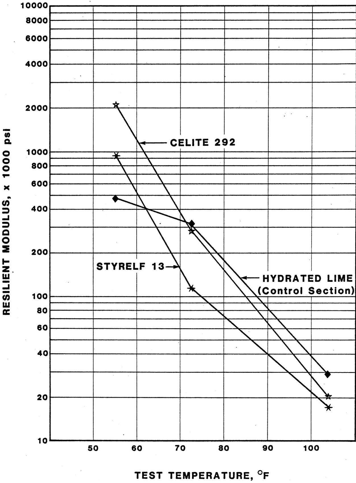
Figure 2a. Resilient modulus vs. test temperature.
