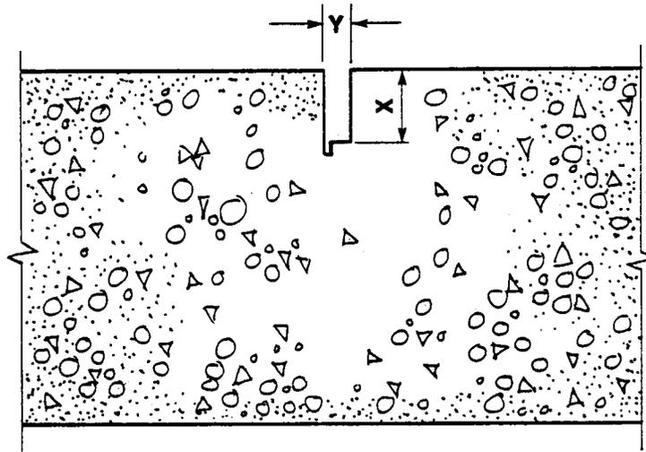
Figure 1. Shape of the sawed joint.
