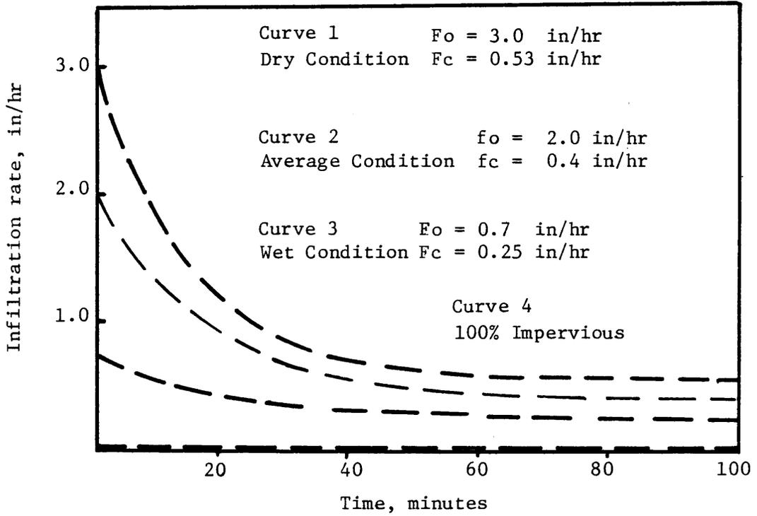
Figure 10. Infiltration capacity curves.
