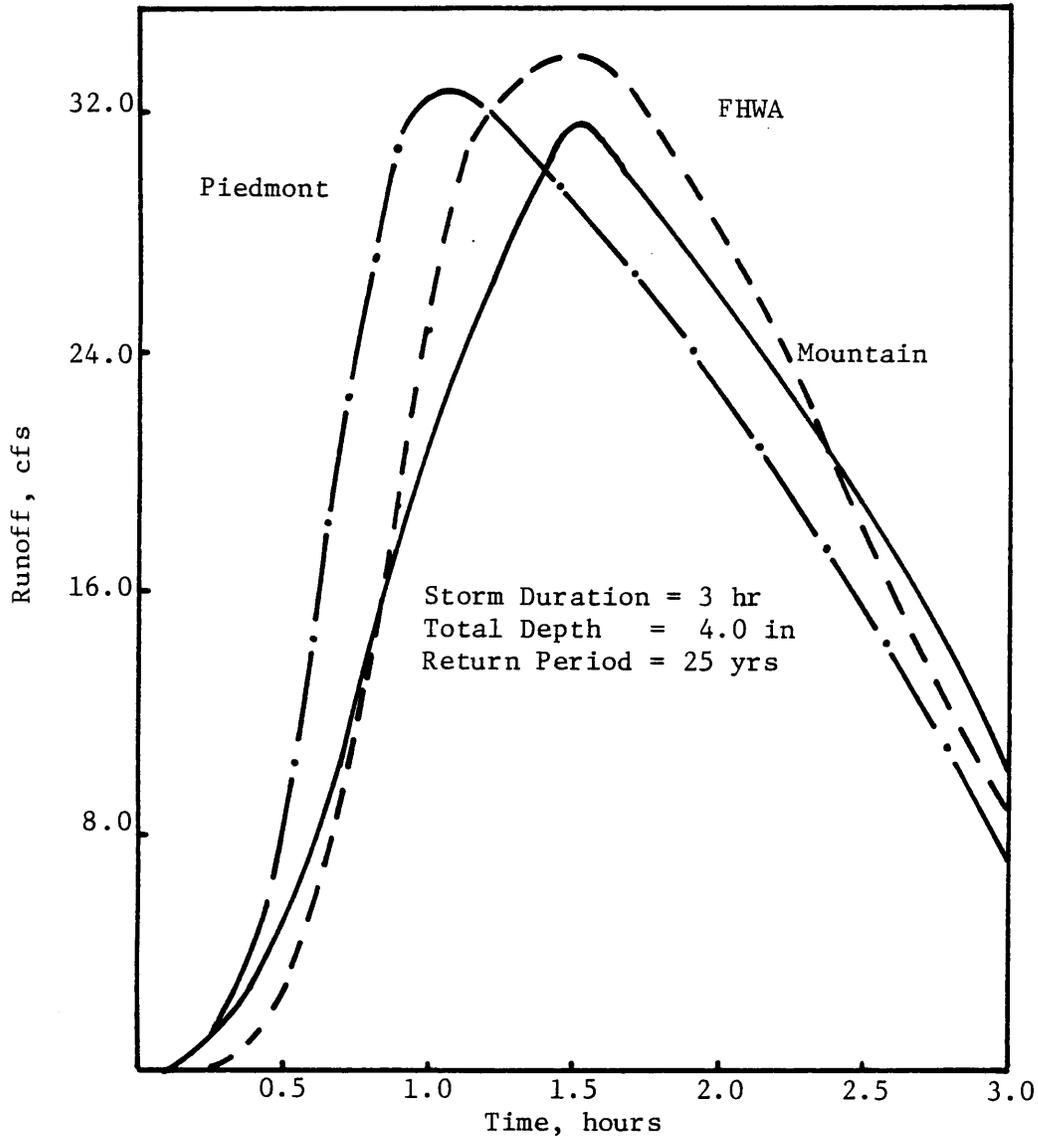
Figure 19. Hydrographs from the 3-hour storm duration with wet antecedent condition.
