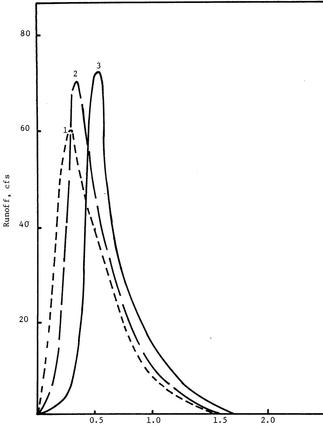
Figure 5. Hydrographs for storm of 30-min duration with normal antecedent soil moisture condition. Return period = 100 years.
