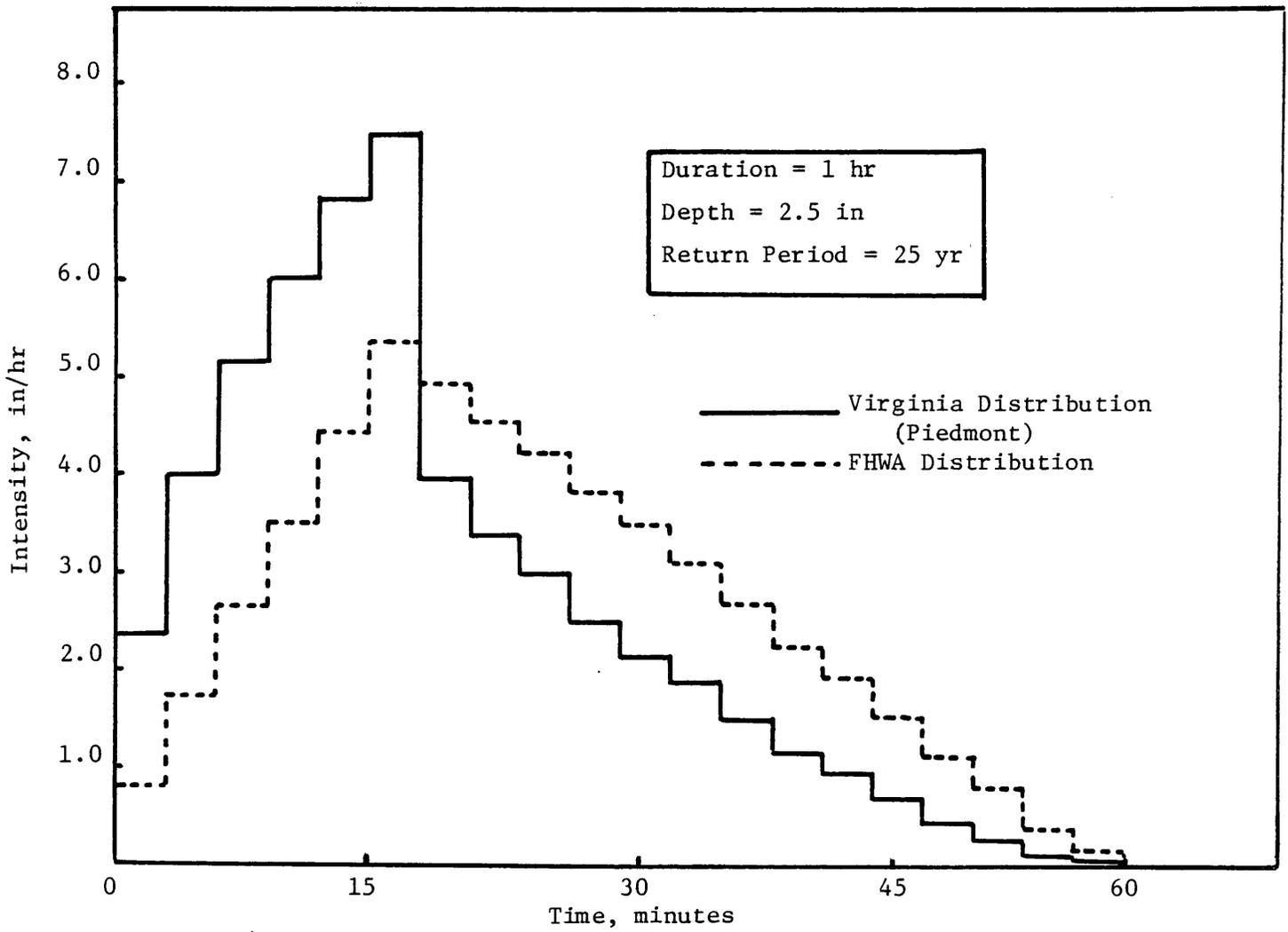
Figure 17. Hyetographs for the piedmont and FHWA distribution.
