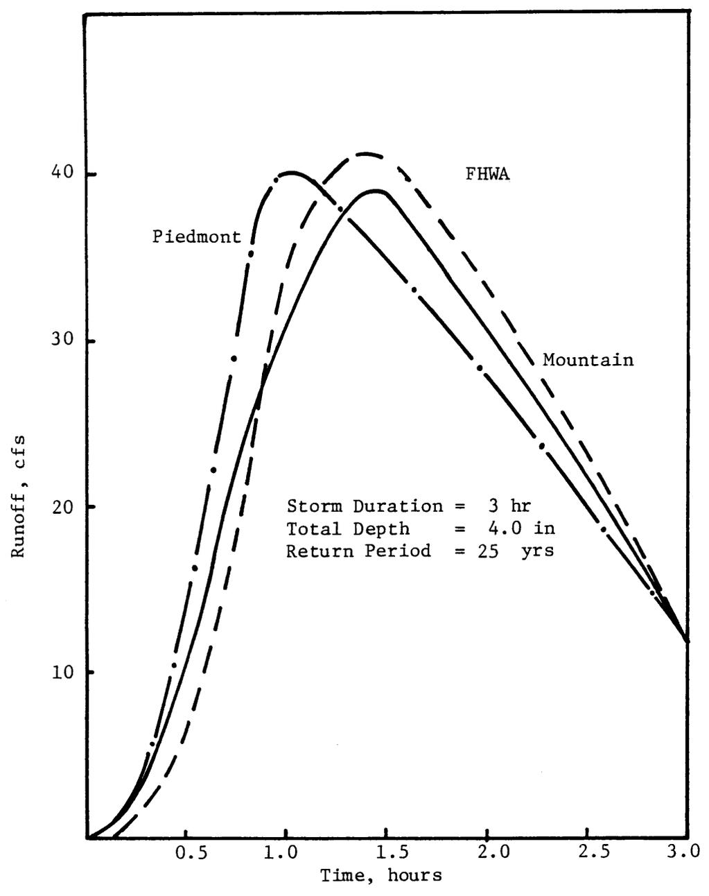
Figure 20. Hydrographs from the 3-hour storms. 100% impervious.
