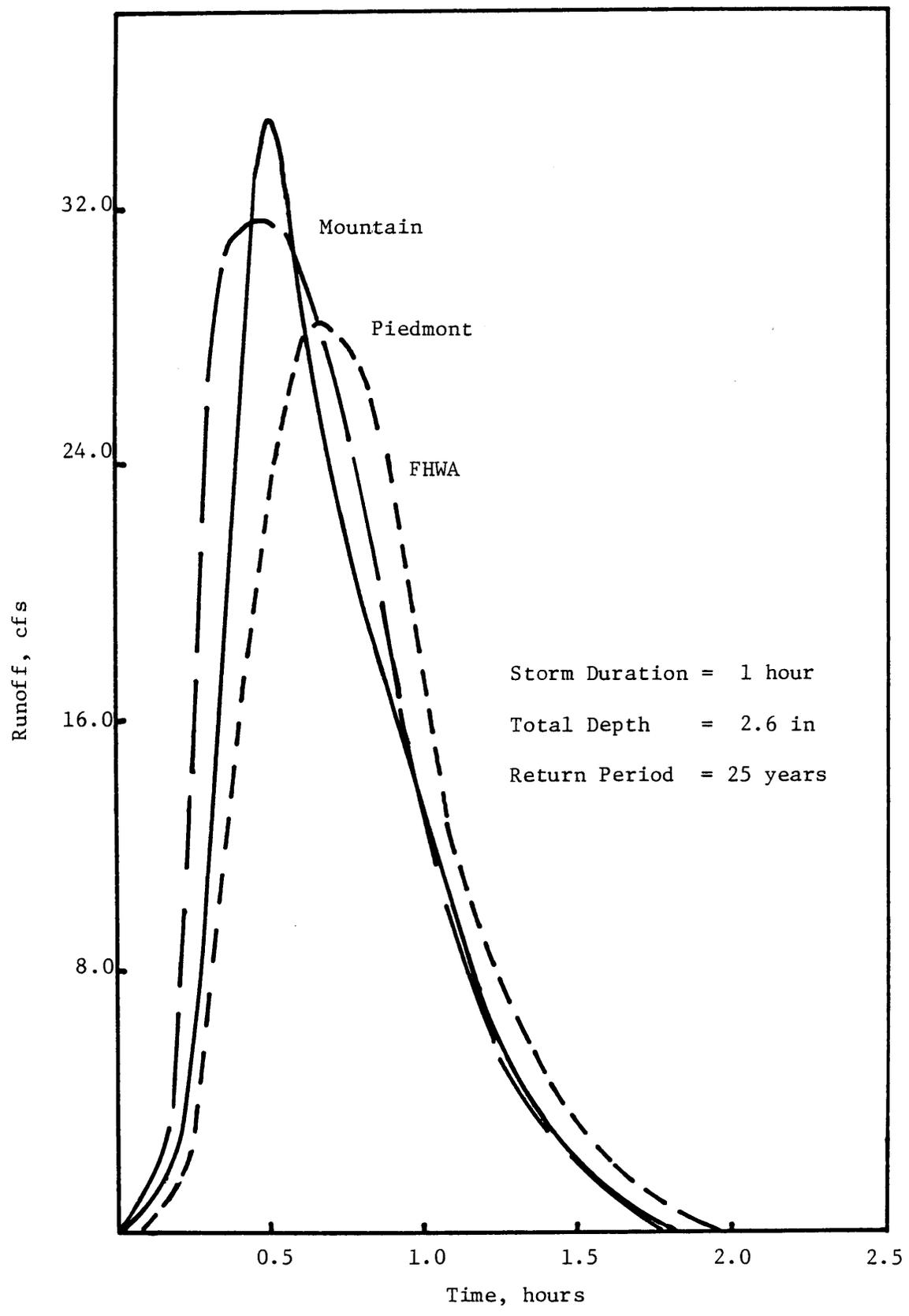
Figure 14. Hydrographs from the 1-hour storm with normal antecedent soil moisture condition.
