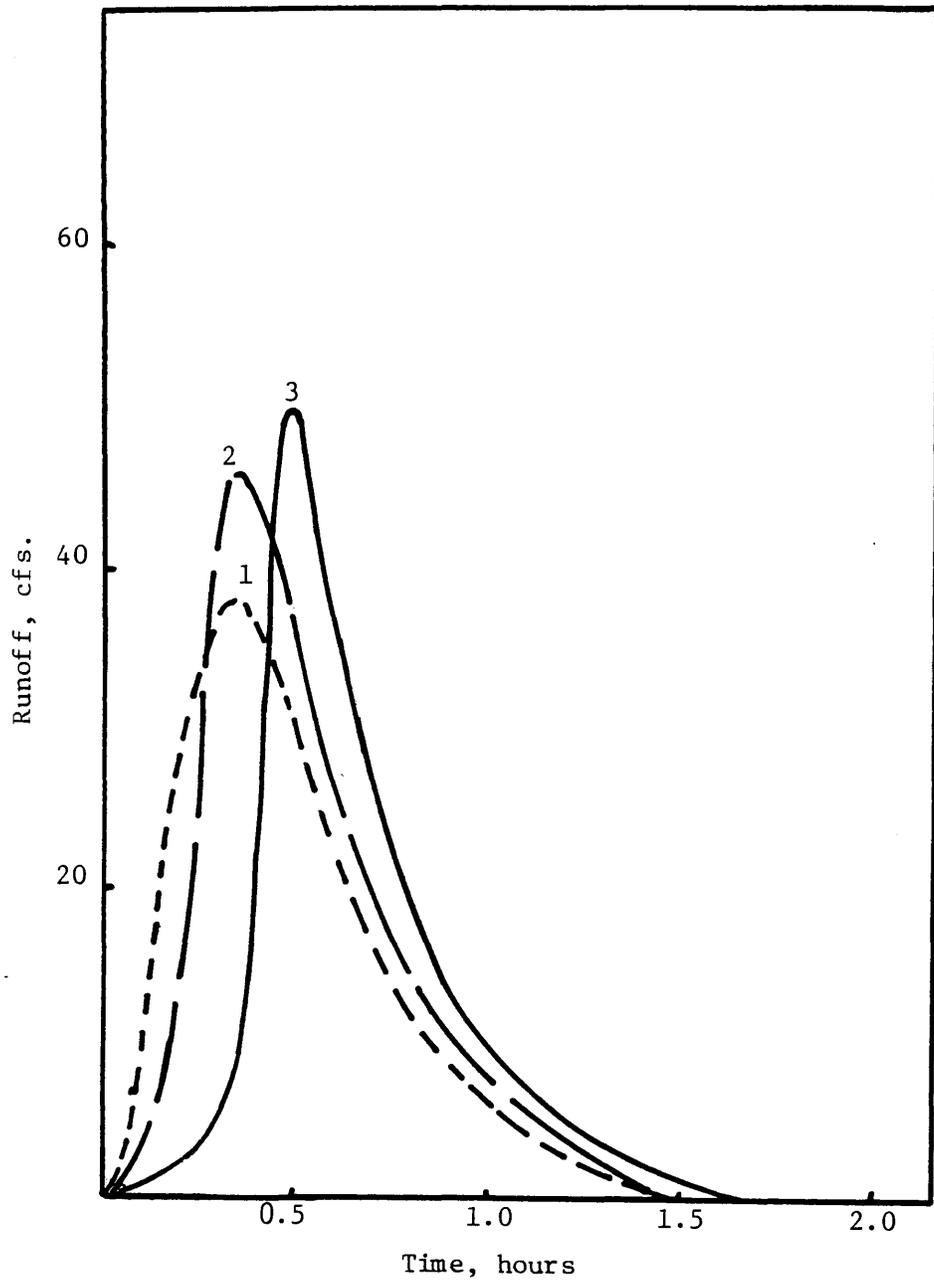
Figure 4. Hydrographs for storm of 30-min duration with normal antecedent soil moisture condition. Return period = 25 years.
