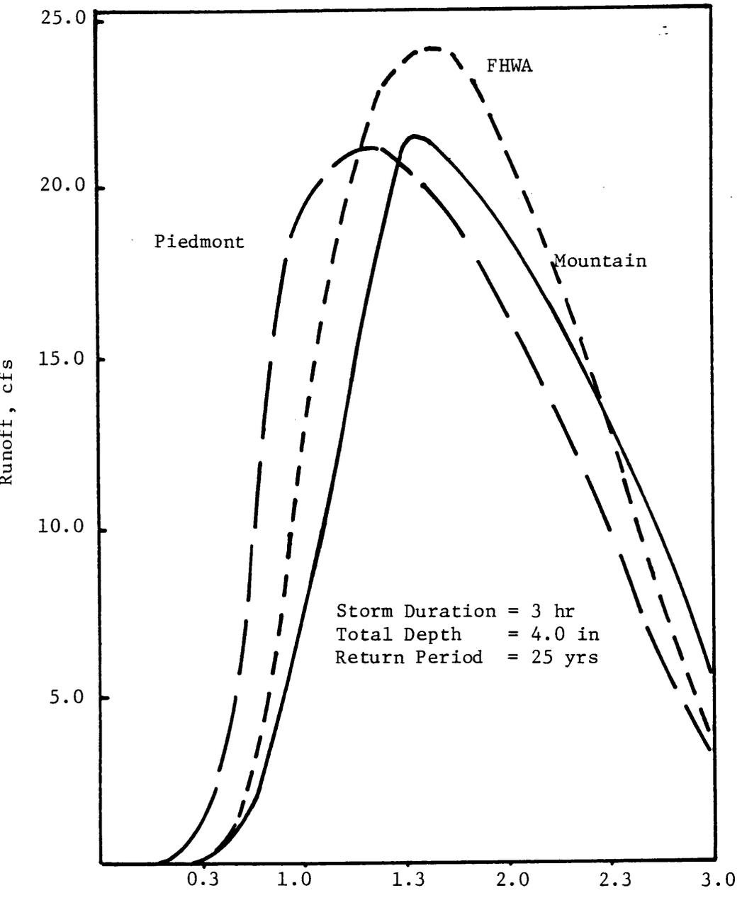
Figure 18. Hydrographs from the 3-hour storms during dry antecedent conditions.
