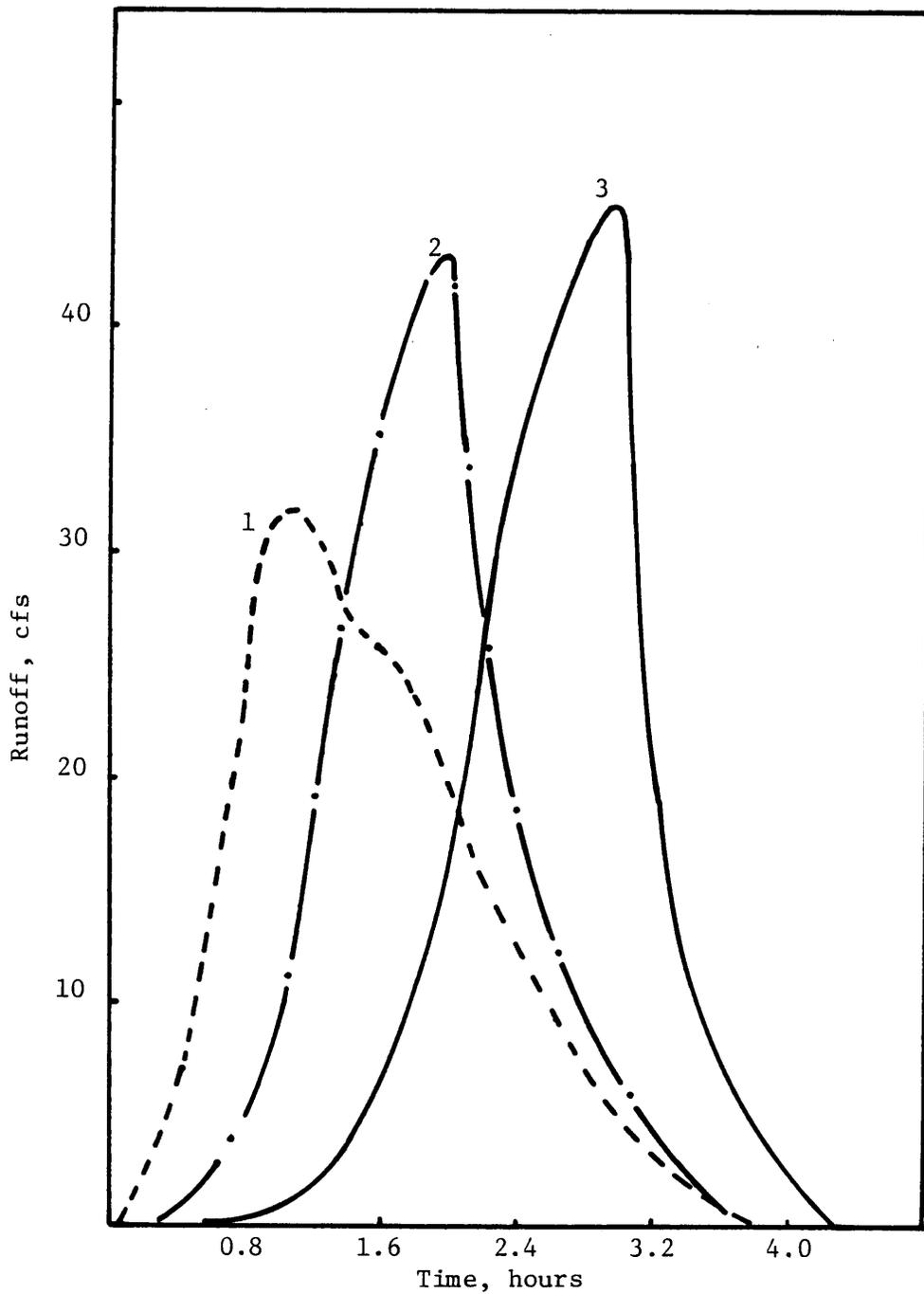
Figure 9. Hydrograph for storms of 3-hour duration with normal antecedent soil moisture condition. Return period = 100 years.
