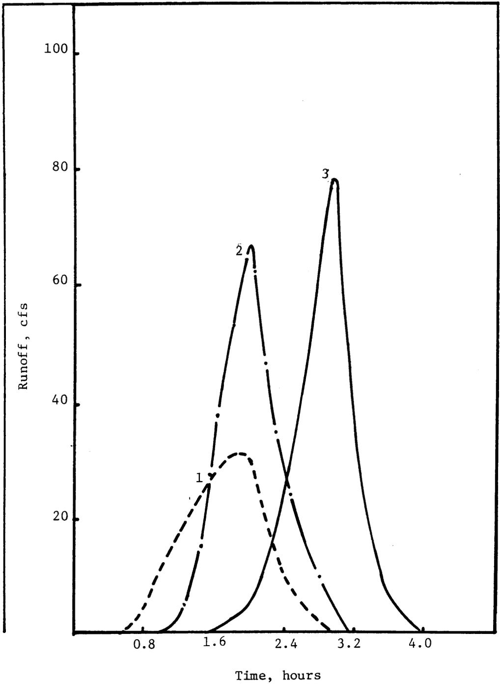
Figure 7. Hydrograph for storm of 3-hour duration with normal antecedent soil moisture condition. Return period = 2 years.
