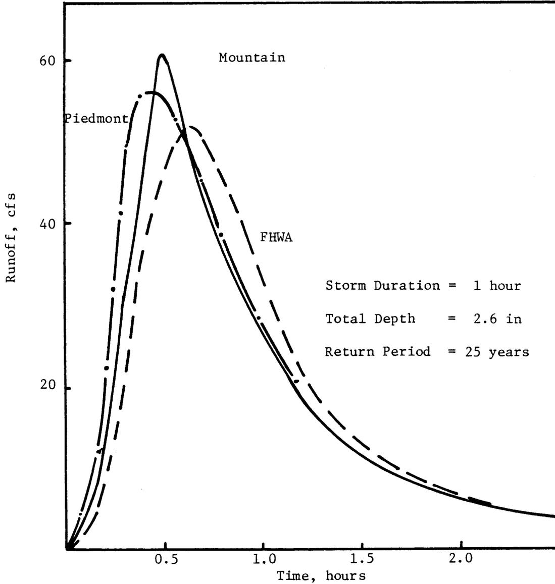
Figure 15. Hydrographs from the 1-hour storm with wet antecedent soil moisture condition.
