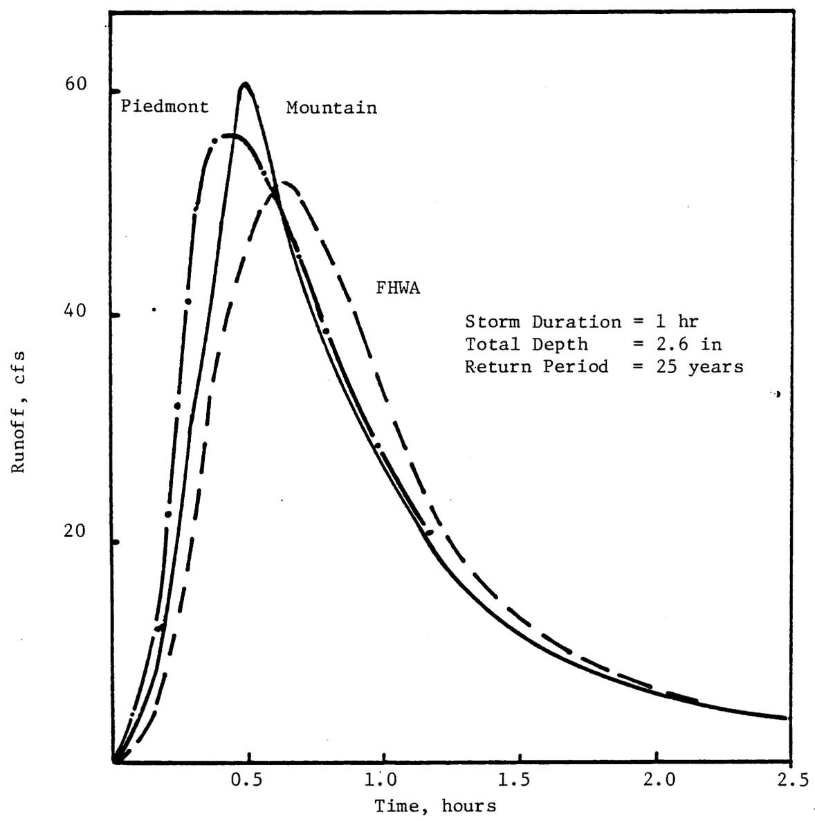
Figure 16. Hydrographs from the 1-hour storms. 100% impervious.
