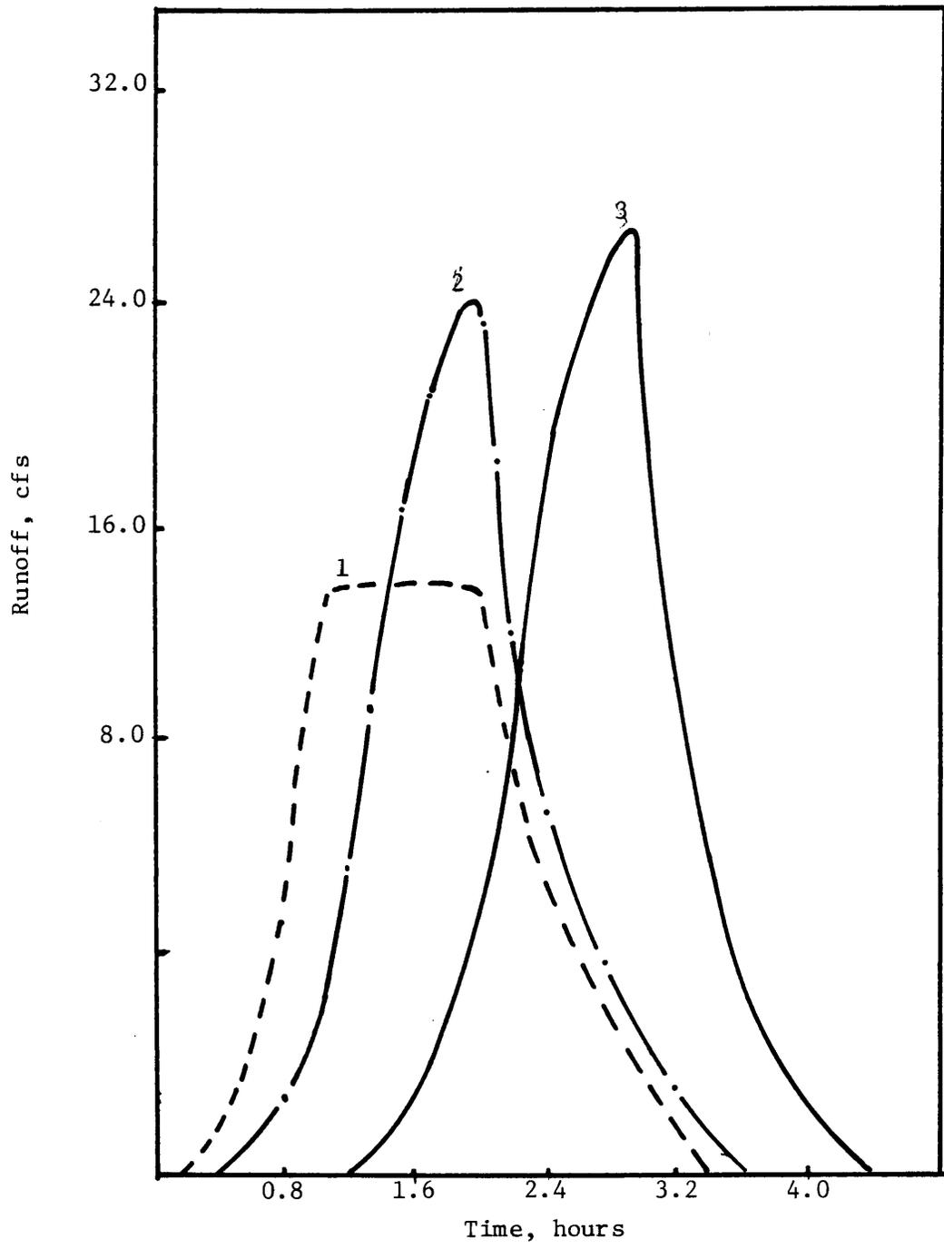
Figure 8. Hydrograph for storm of 3-hour duration with normal antecedent soil moisture condition. Return period = 25 years.
