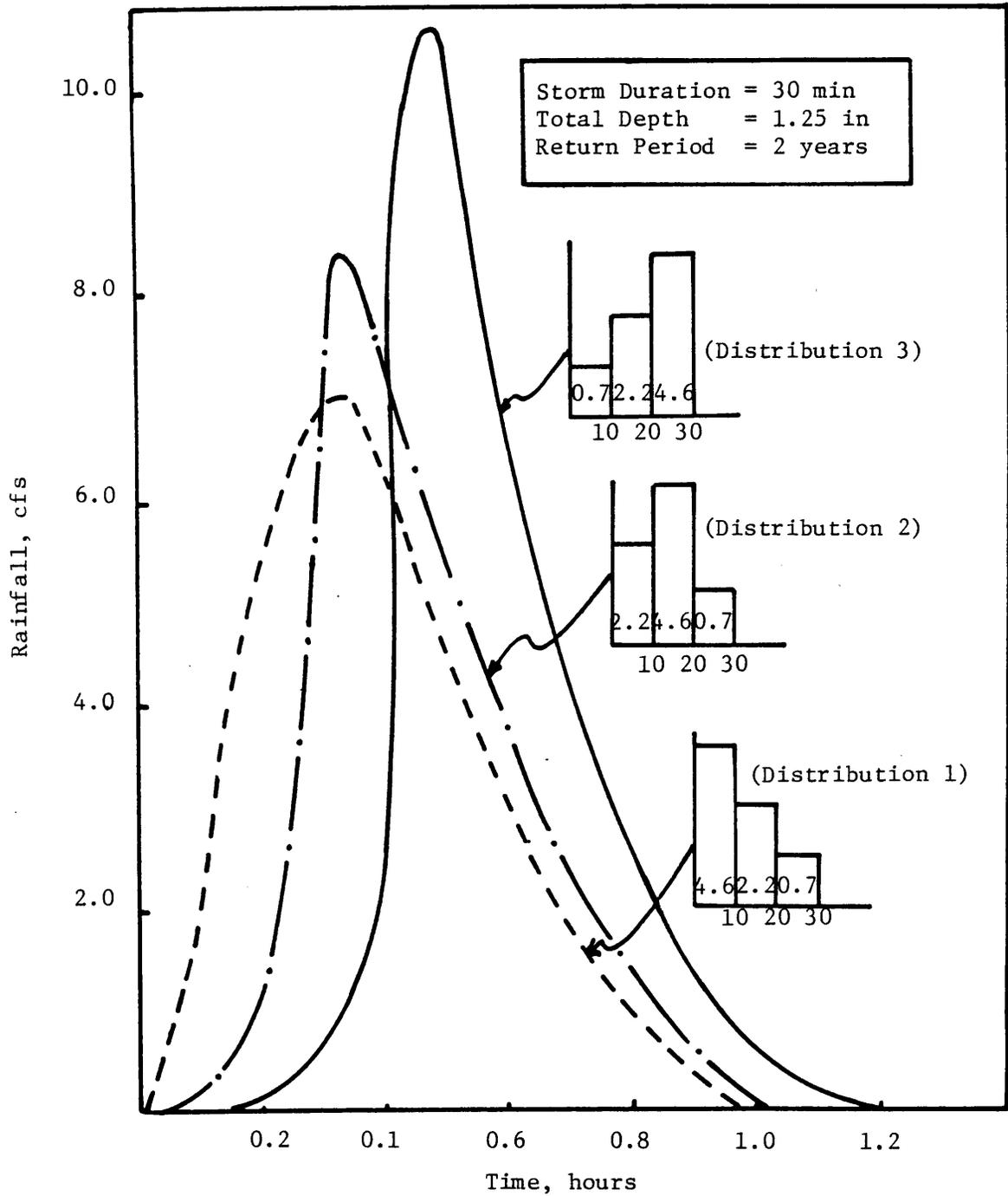
Figure 3. Hydrographs for storm of 30-minute duration with normal antecedent soil moisture condition. (Note: cfs is used for  $ft^2/s$  throughout this report.)
