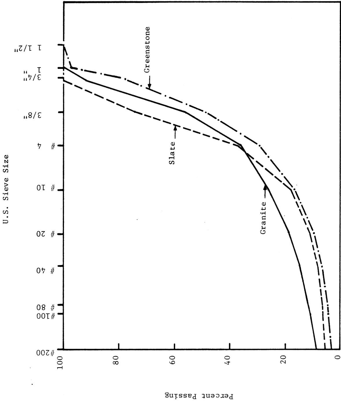
Figure 1. Gradations of aggregates as delivered, Rte. 660.
