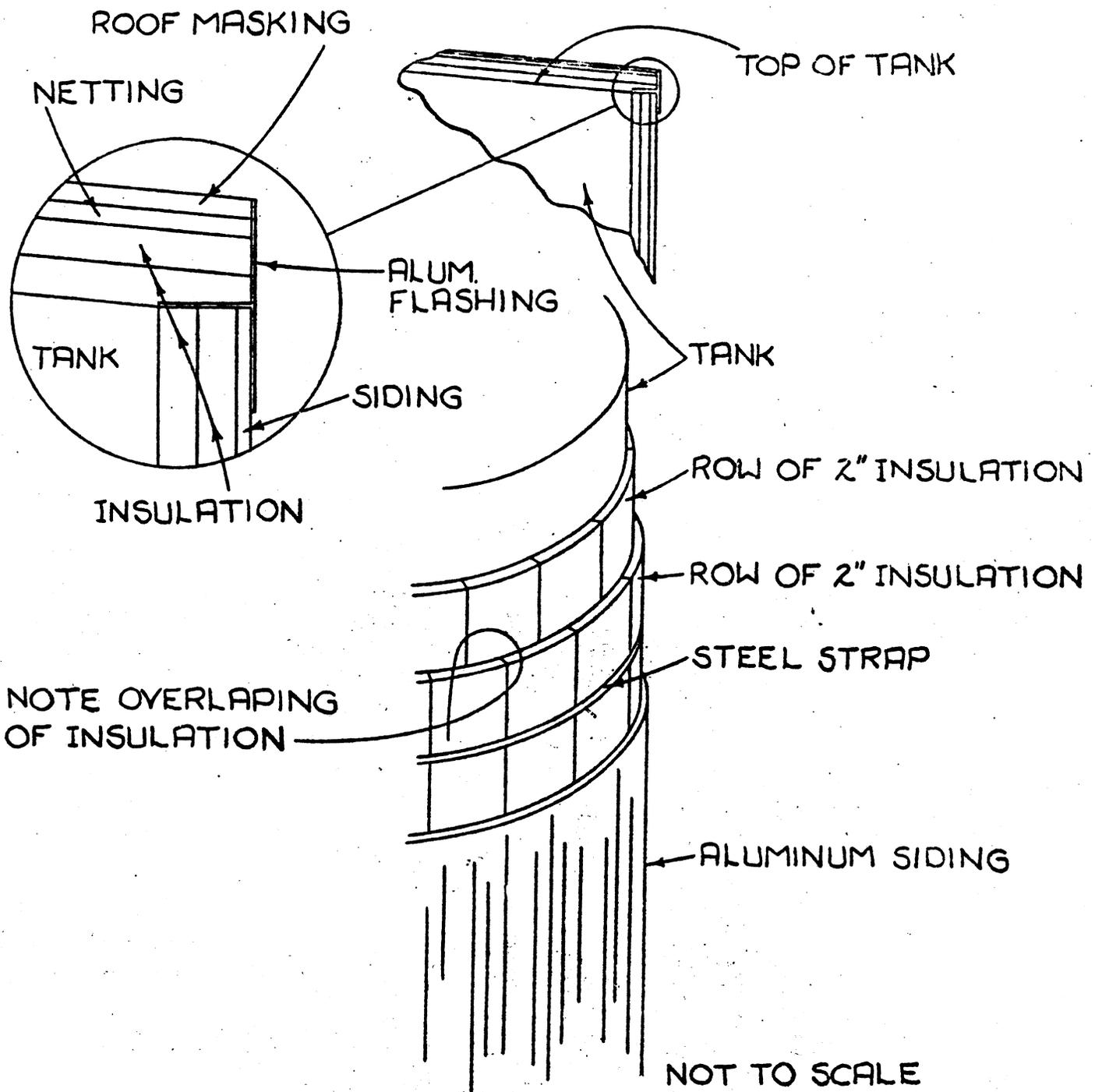
Figure A-4. Details for insulating the bituminous and hot water tanks.
