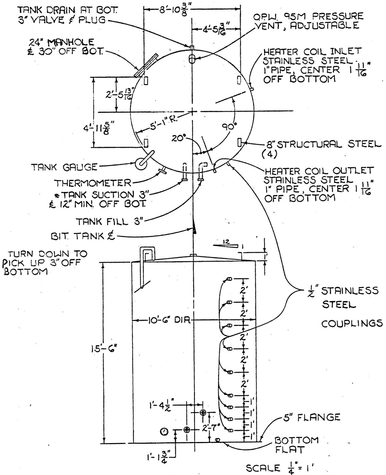
Figure A-1. Details of 10,000 gal. bituminous tank.
