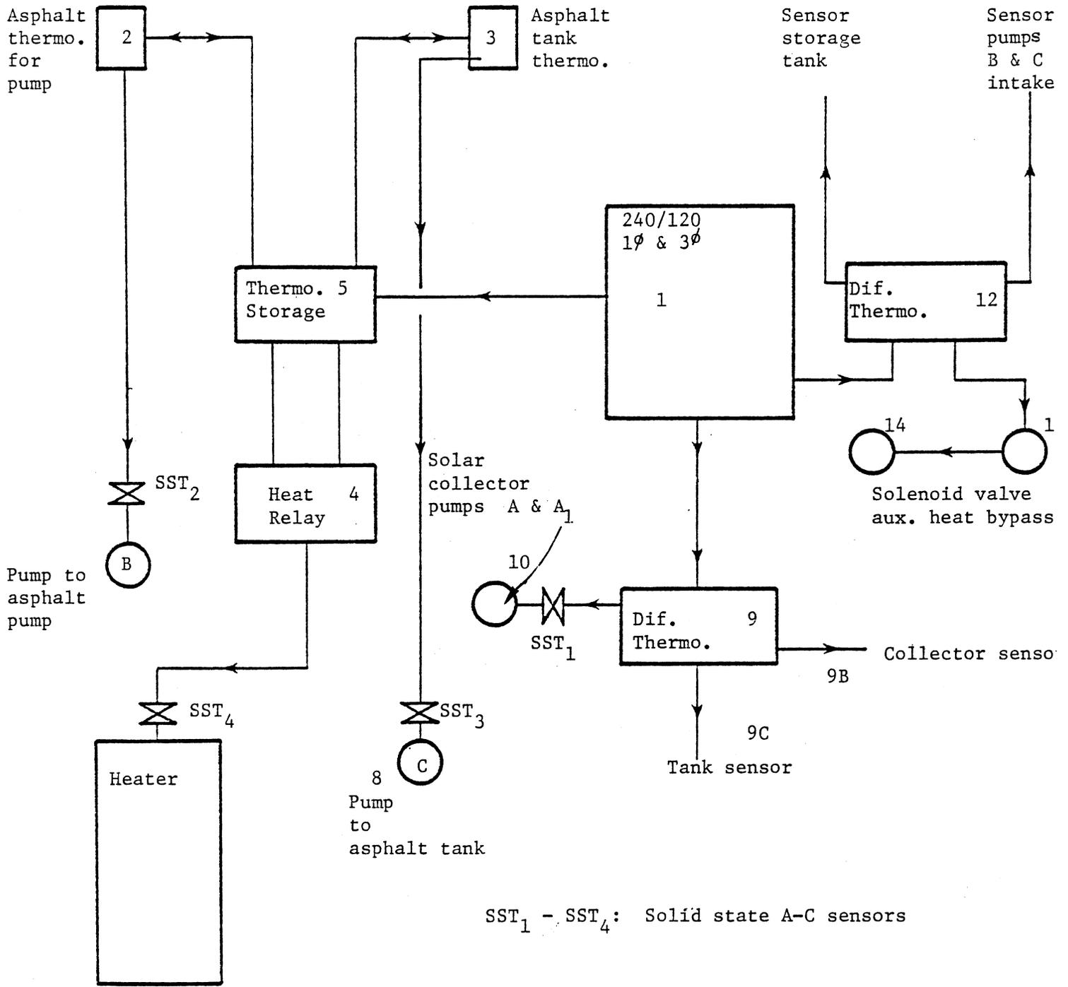
Figure 4. Electrical control layout for asphalt tank solar system.
