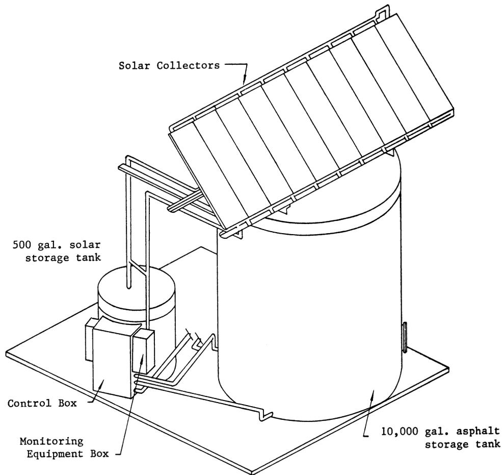
Figure 1. Schematic of the asphalt storage tank and solar heating system.
