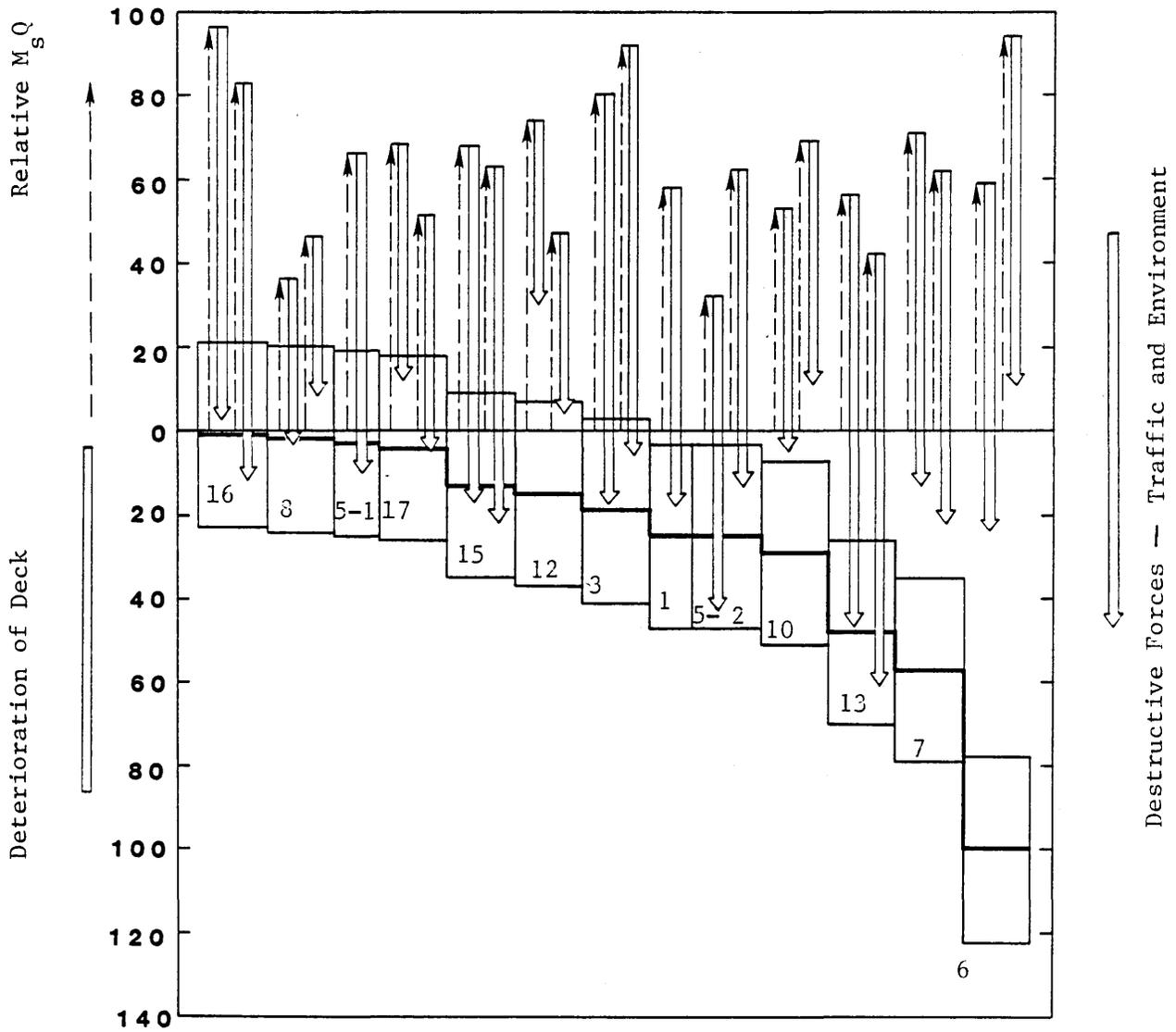
Figure 42. The balance between the quality of the concrete and the forces of deterioration.
