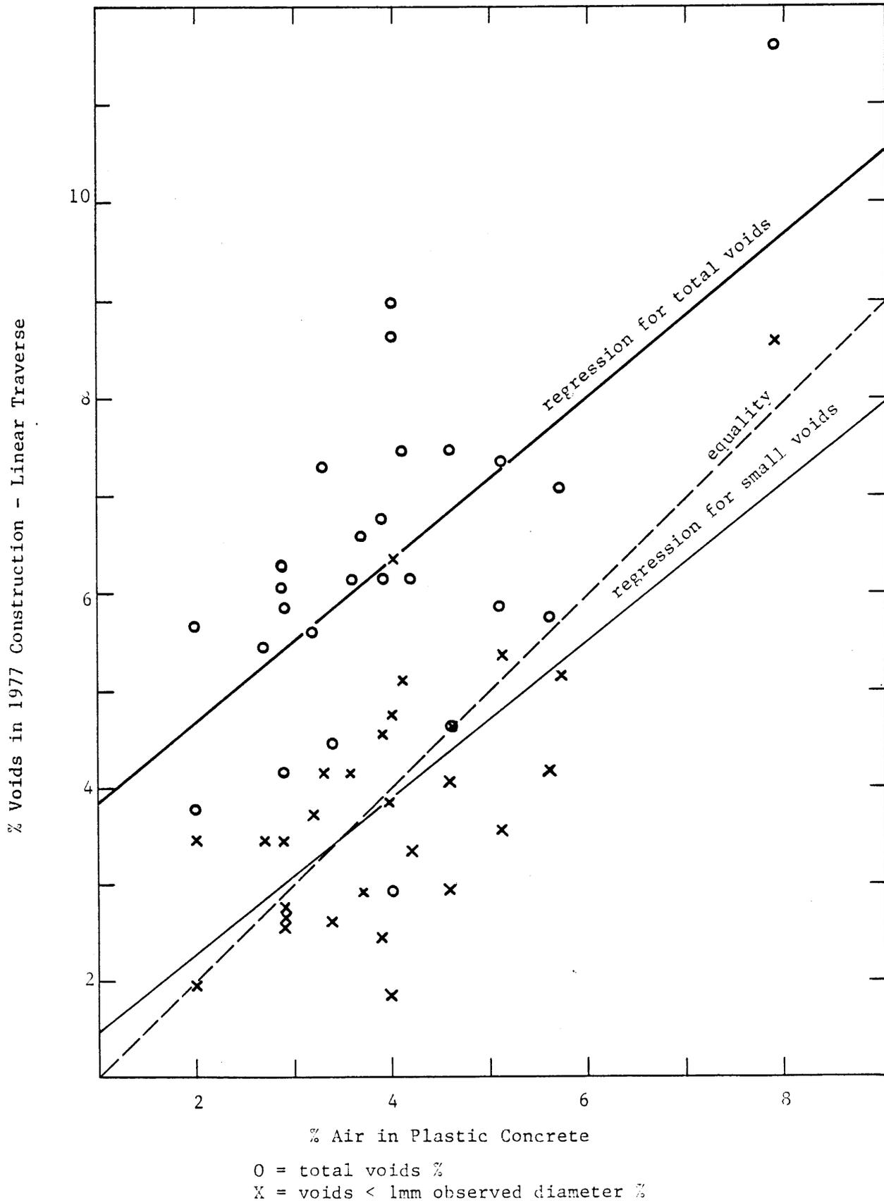
Figure 35. Void system of 1977 cores vs. air content of plastic concrete.
