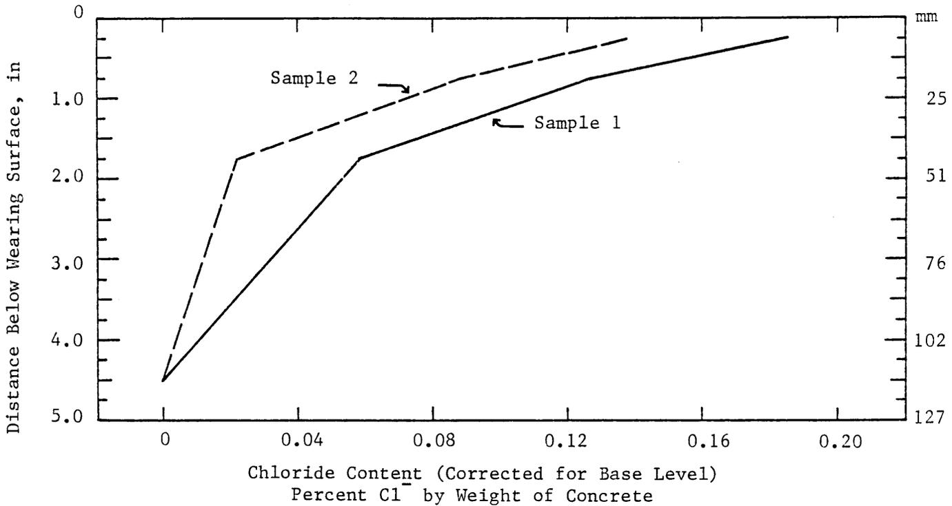
Figure 3. Chloride distribution in bridge #13. Relationship typical of bridges #3, #7, #8, #10 and #13.
