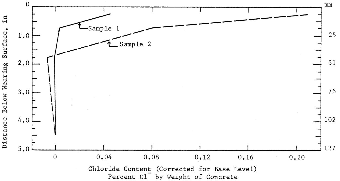
Figure 6. Chloride distribution in bridge #16.
