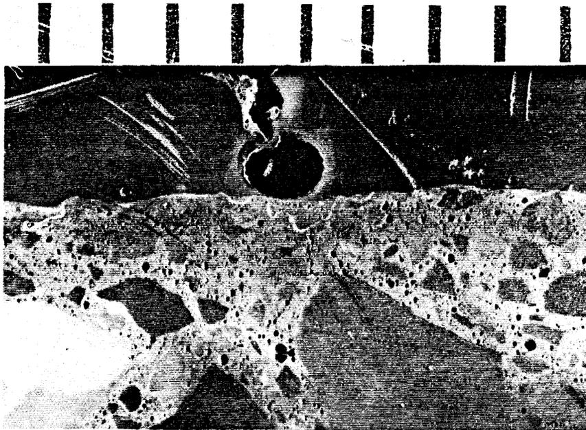
Figure 34. View of near surface of hardened concrete from sample 5-2. Note that fine cracking terminates at curing compound, which is intermixed with concrete. Large void at the top of the picture is in the epoxy mounting.
