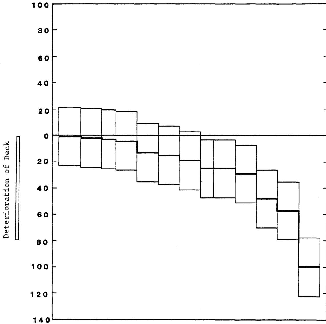
Figure 41. Non-overlaid bridges arranged in order of increasing deterioration. Relative amount of scaling and cracking shown by heavy black line plotted on scale of 0 to -100.
