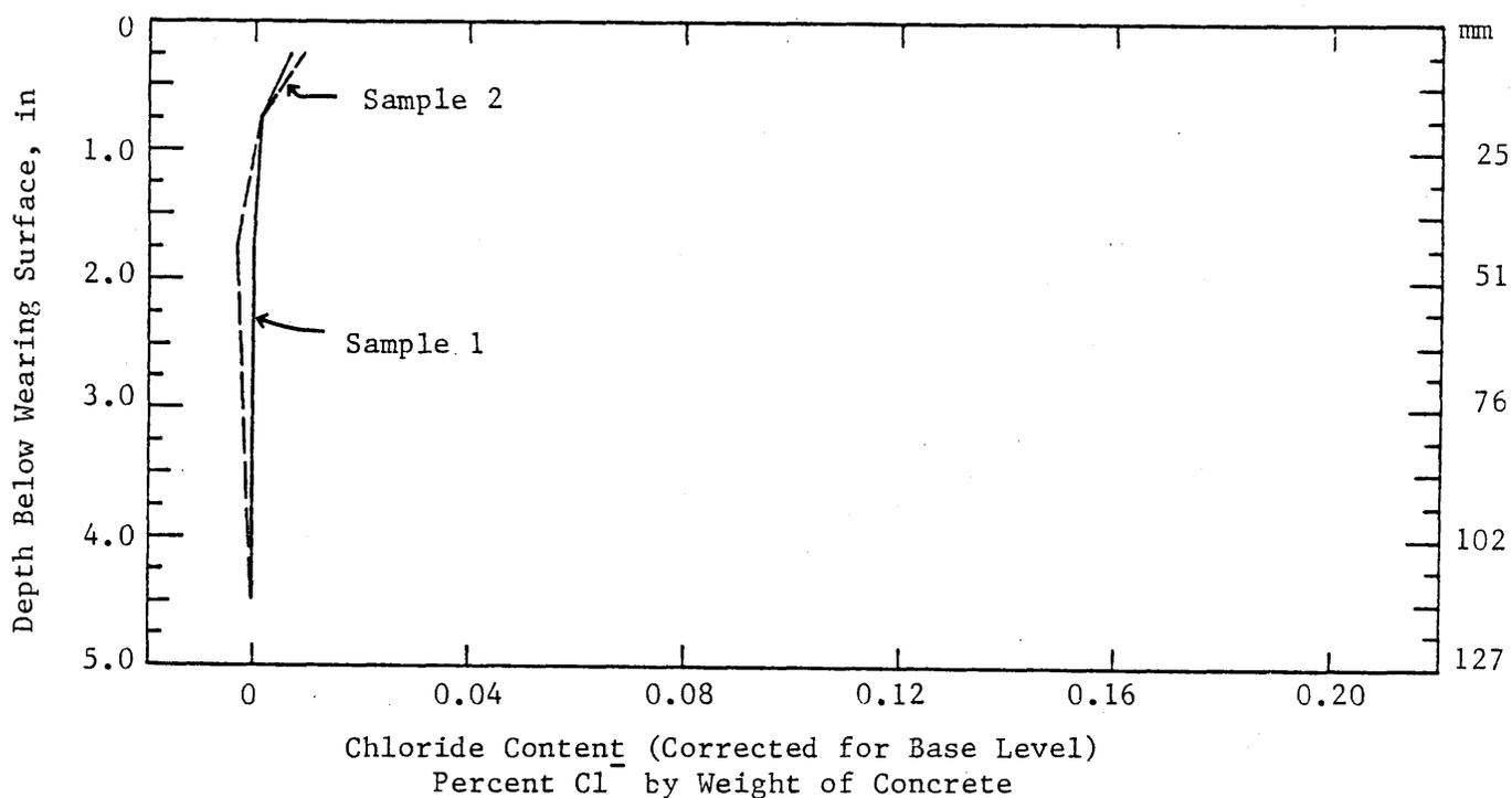
Figure 7. Chloride distribution for bridge #17 (typical for bridges #12 and #17).
