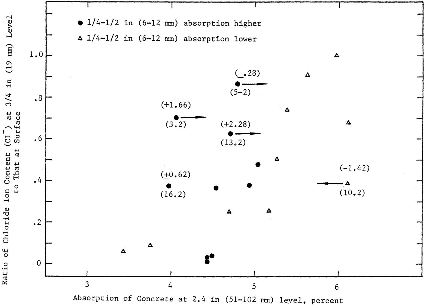
Figure 10. Relationship of chloride intrusion  $\frac{1}{4}$  -  $\frac{1}{2}$  in (6-13mm) absorption higher to a depth of  $\frac{3}{4}$  in (19mm) and  $\frac{1}{4}$  -  $\frac{1}{2}$  in (6-13mm) absorption lower.
