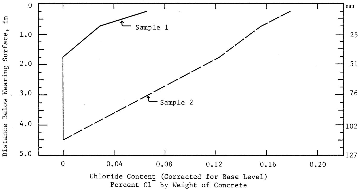
Figure 4. Chloride distribution in bridge #5 samples.
