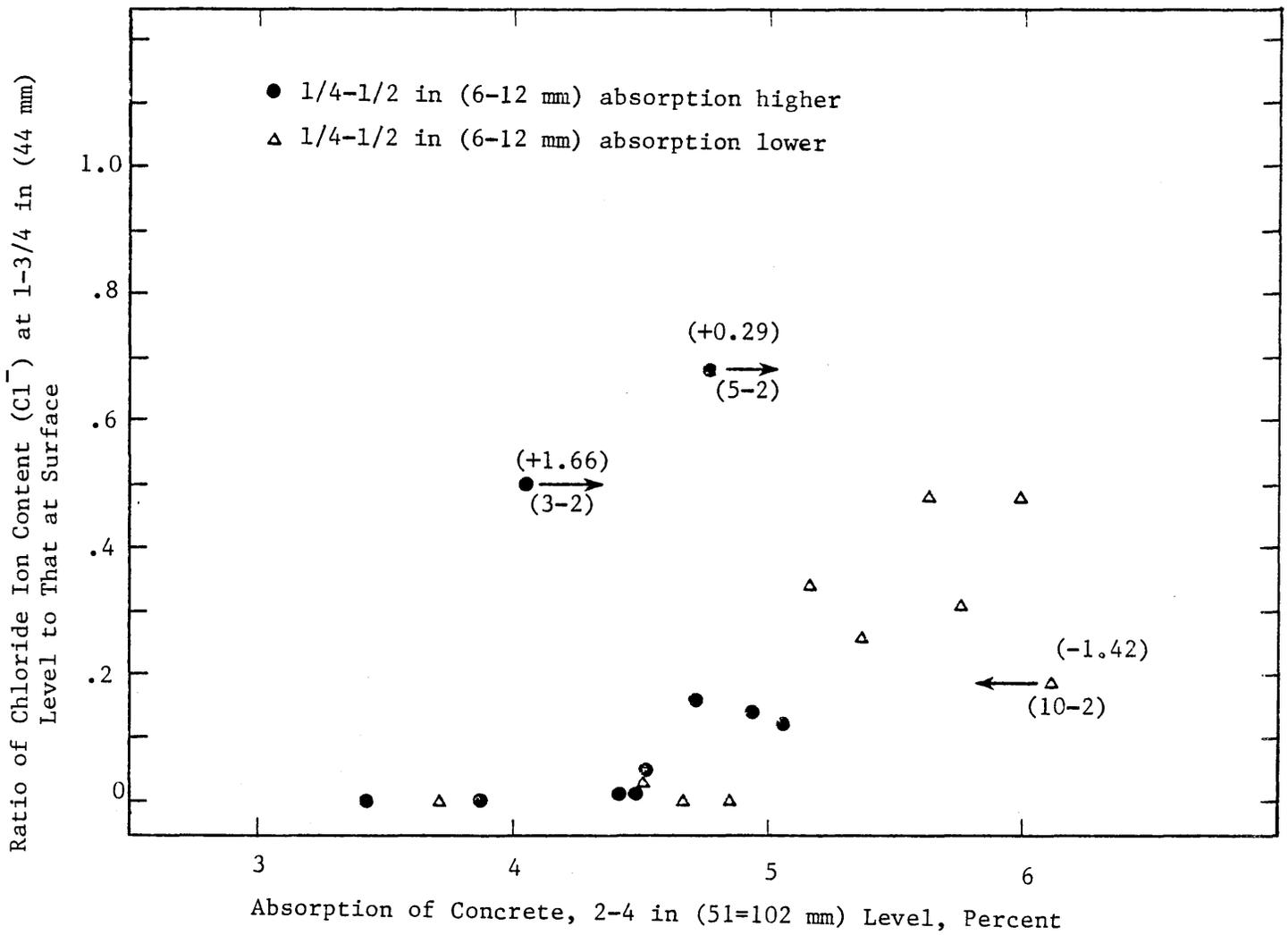
Figure 9. Relation of chloride intrusion to a depth of 1 3/4 in (44 mm) and absorption of the concrete.
