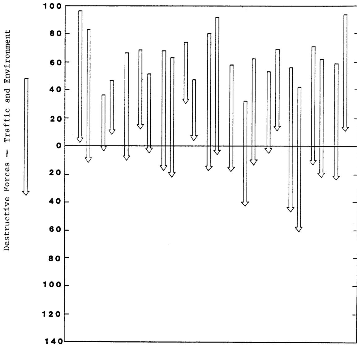
Figure 40. Non-overlaid bridges arranged in order of increasing deterioration. Sum of EO and TQ plotted downward from end points in Figure 39.
