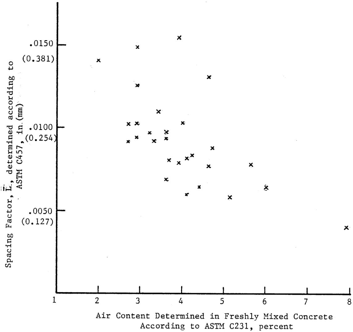
Figure 36. Relationship between Spacing Factor,  $\bar{L}$ , determined on hardened concrete and the air content measured by the pressure method at the time of placement.
