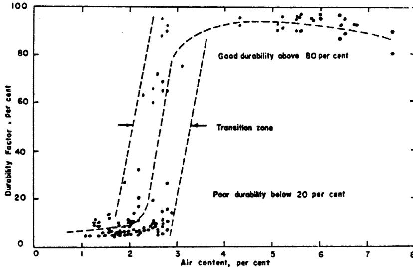
Figure 2. Durability of concrete containing various aggregates, cement contents, water-cement ratios, and air contents. (After Cordon and Merrill 1963.)
