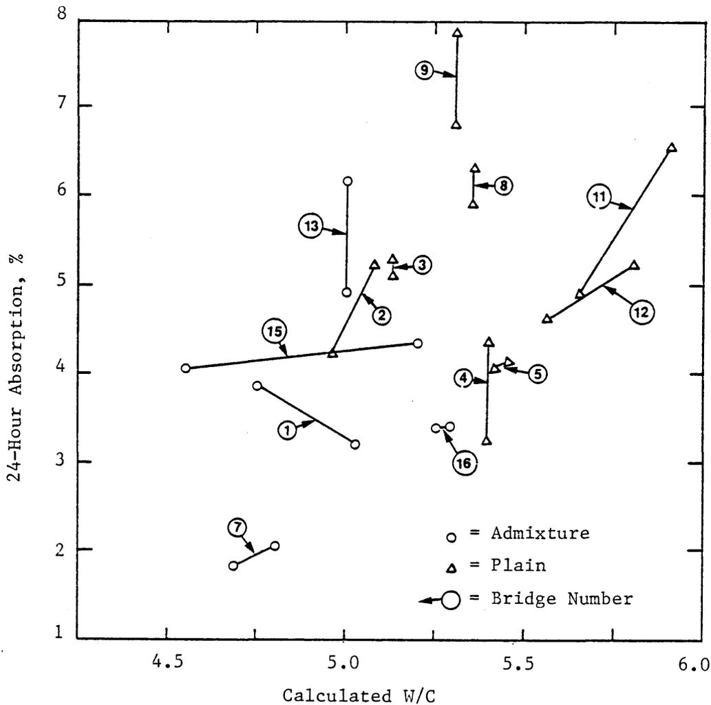
Figure 11. Relationship between measured absorption and calculated water-cement ratio. Data not available for bridges #6, #10, #14, and #17. (Reproduced from Newlon 1971.)
