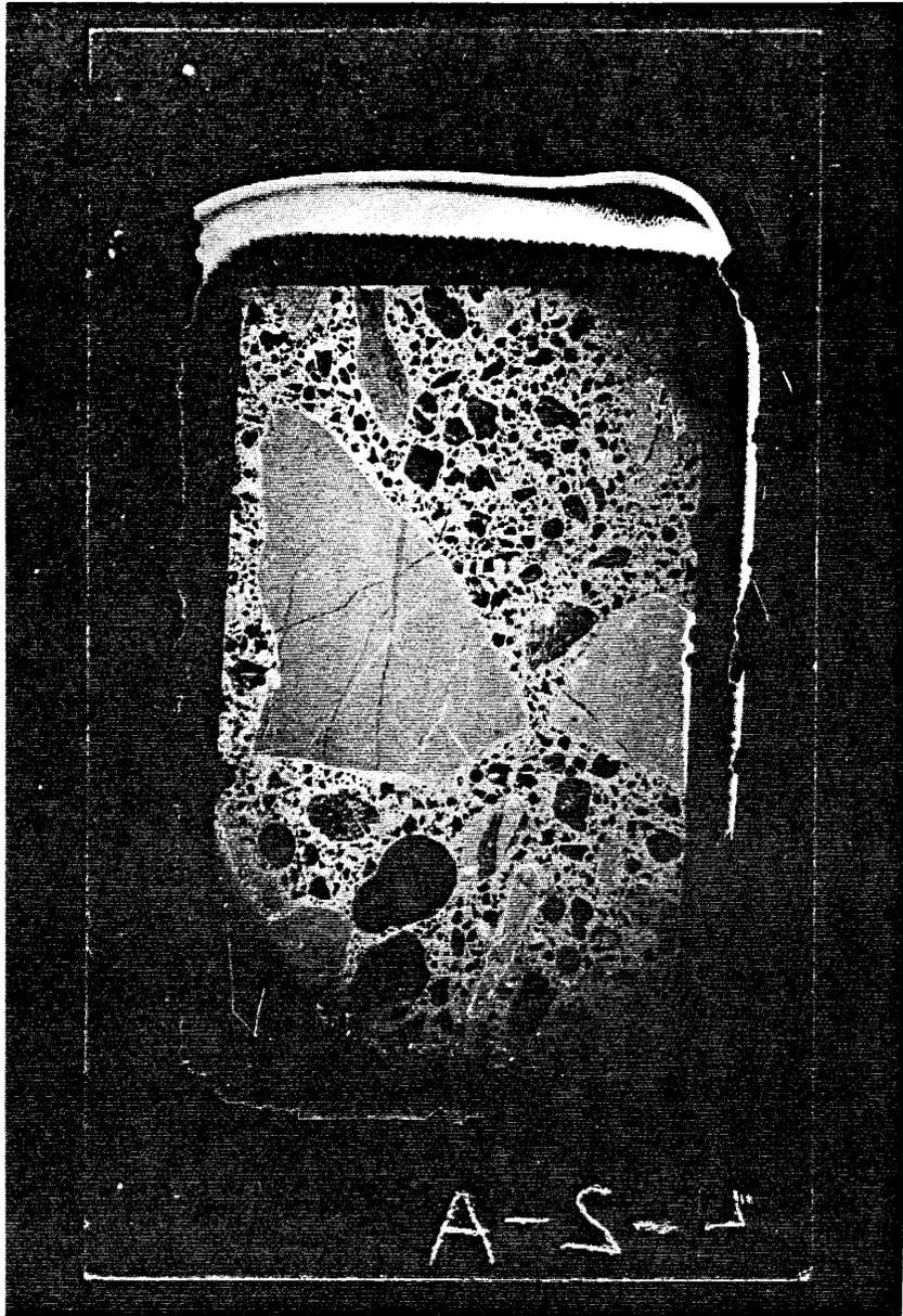
Figure 38. Thin section of concrete mounted on glass with epoxy. The section is 18  $\mu\text{m}$  thick. The work sheet for this section was shown in Figure 37.
