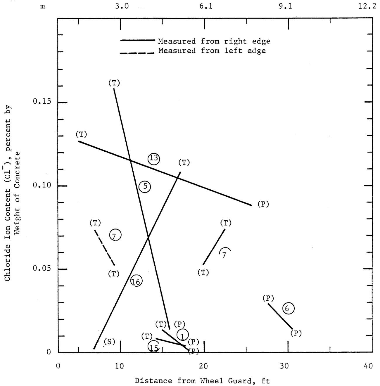
Figure 8. Chloride contents are related to location on the deck and traffic location.
