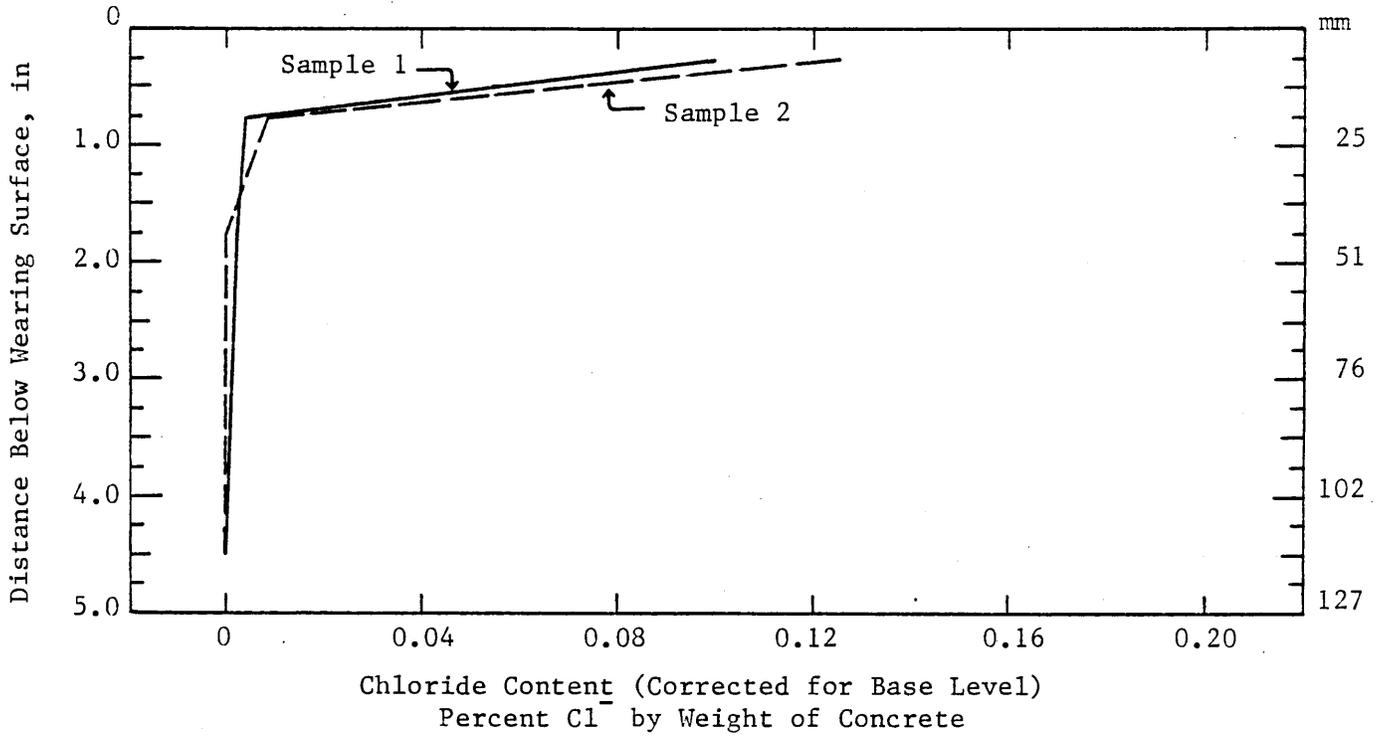
Figure 5. Chloride distribution in bridge #15. Relationship typical of bridges #1, #6 and #15.
