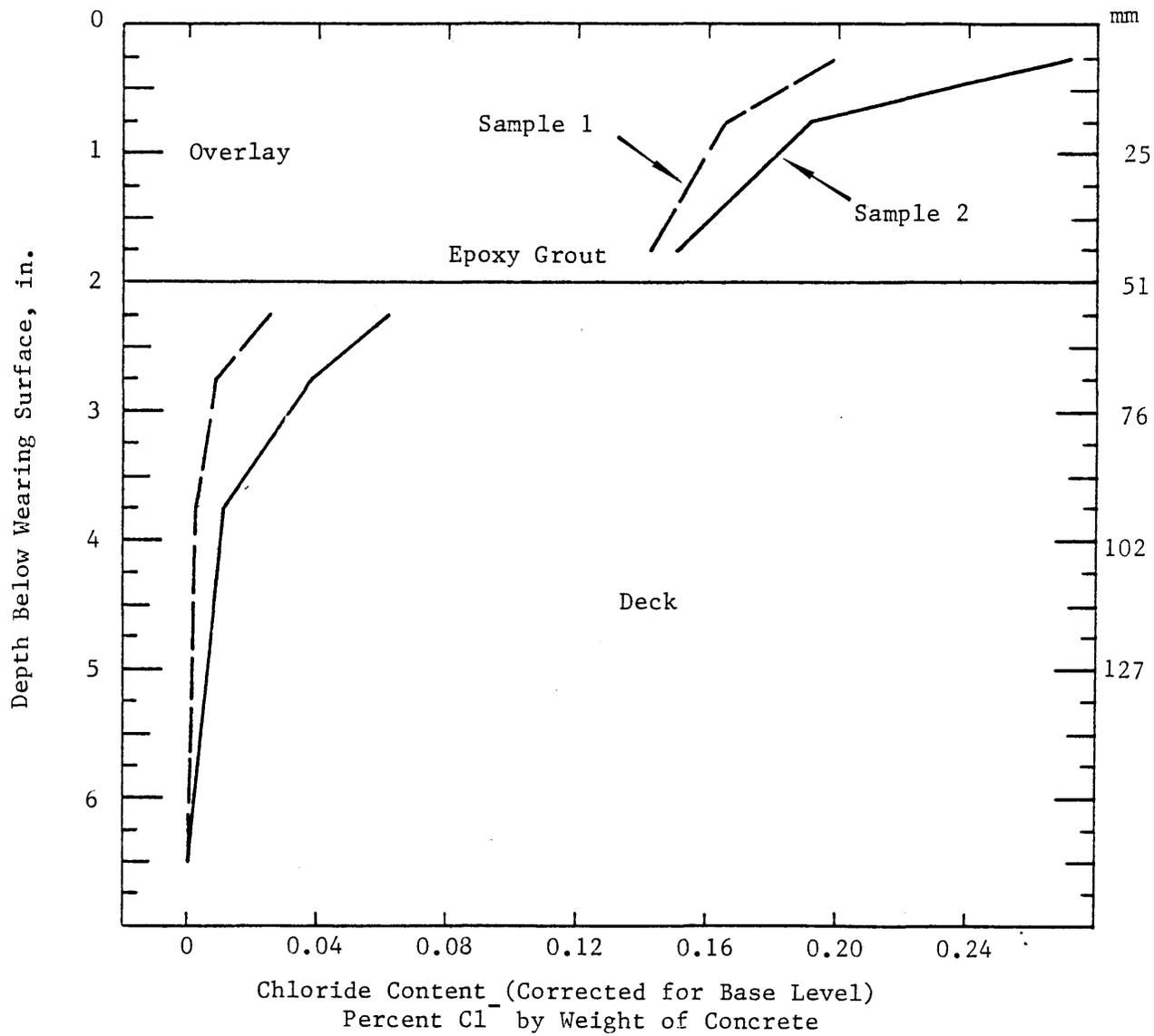
Figure 31. Chloride distribution in bridge #14, which was overlaid prior to traffic.
