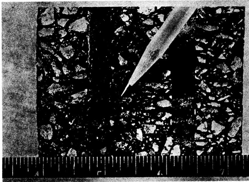
Figure 6. Example of sealant pulling away from side.
