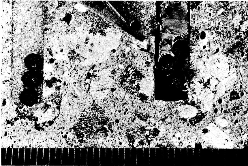
Figure 5. Example of cavity or void and of sealant pulling away from side.
