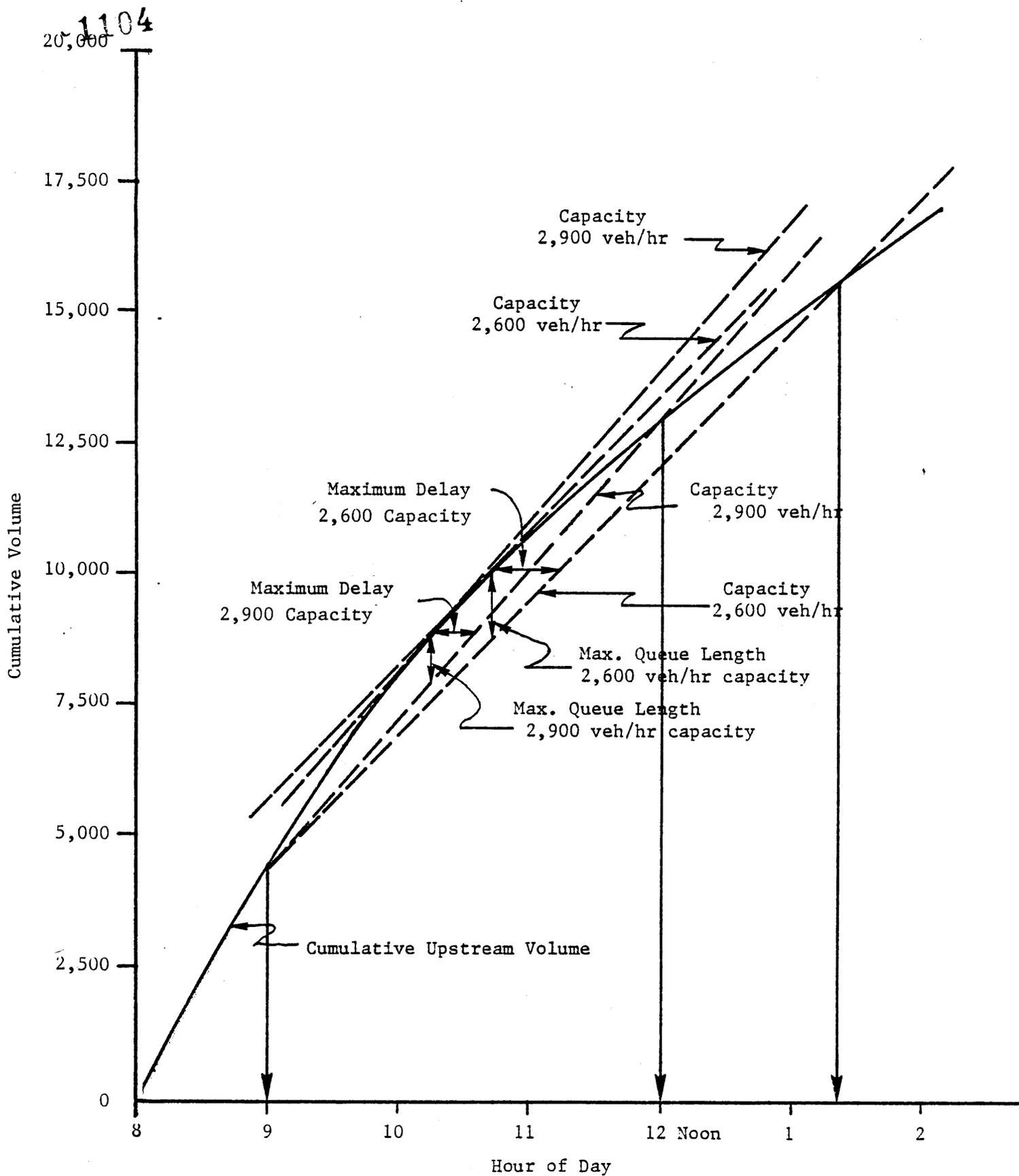
Figure 7. Cumulative demand volume between 8:00 a.m. and 2:00 p.m.
