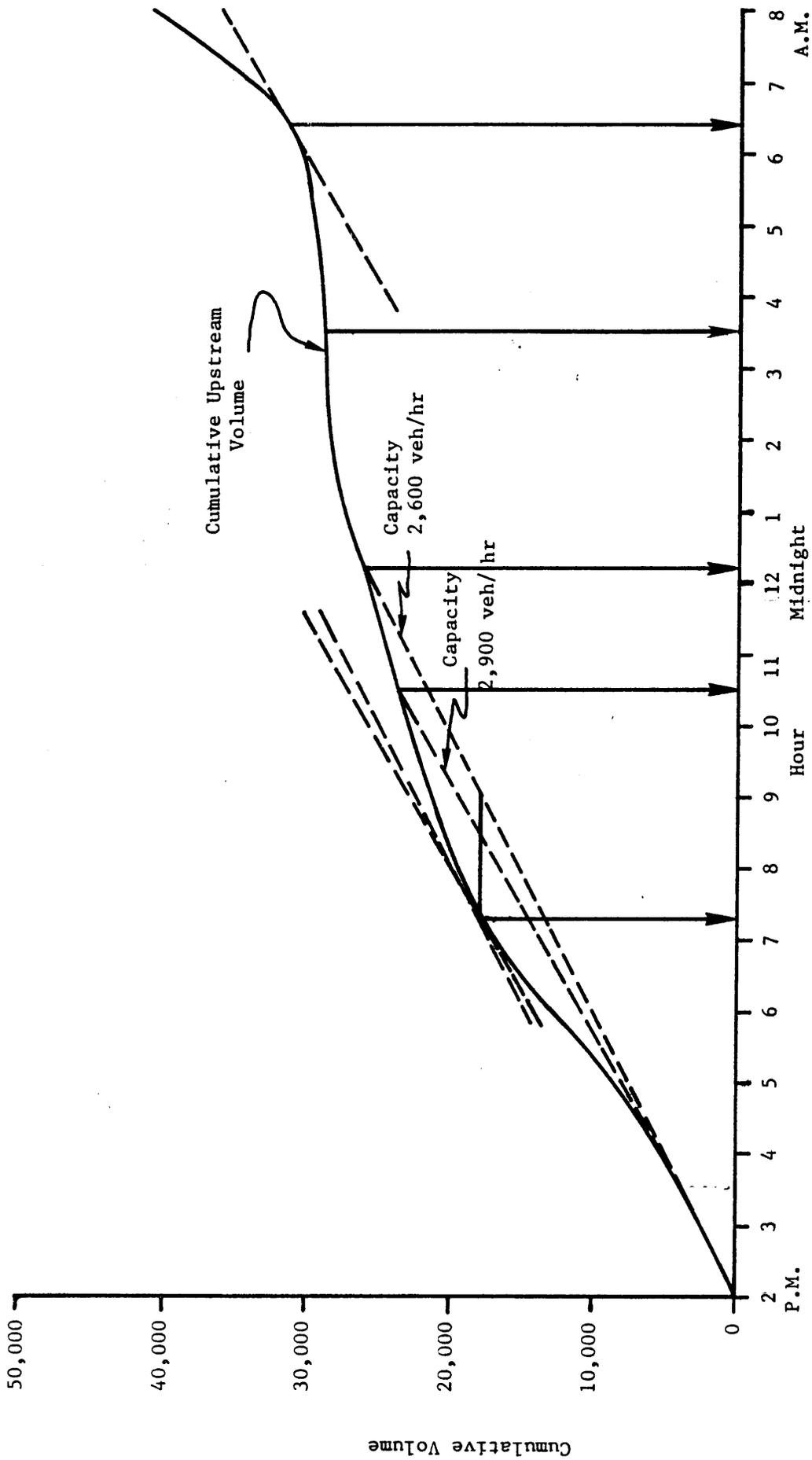
Figure 8. Cumulative demand volume between 2:00 p.m. and 8:00 a.m.
