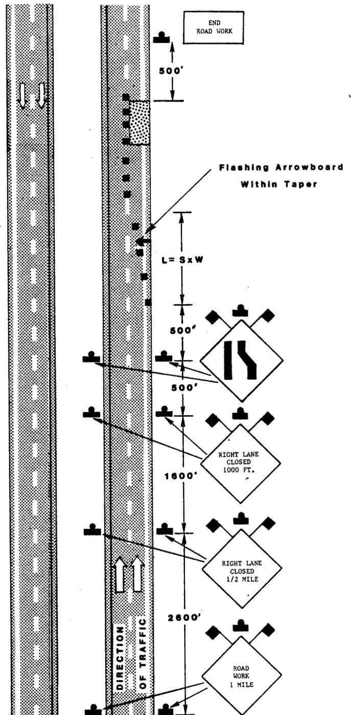
Figure 17. Typical layout for a single-lane closure.
