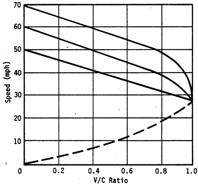
Figure 5. Estimates of vehicle speed. (From reference 6.)
