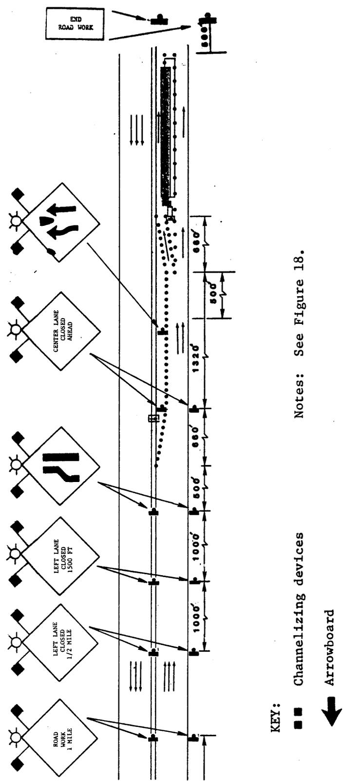
Figure 19. Typical layout for center-lane closure with split traffic.
