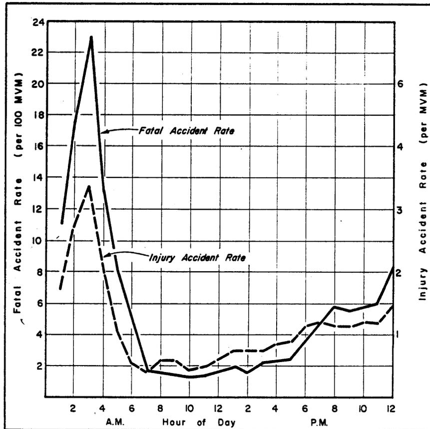
Figure 10. California fatal and injury accident rates expressed as functions of hours of the day. (From reference 12.)
