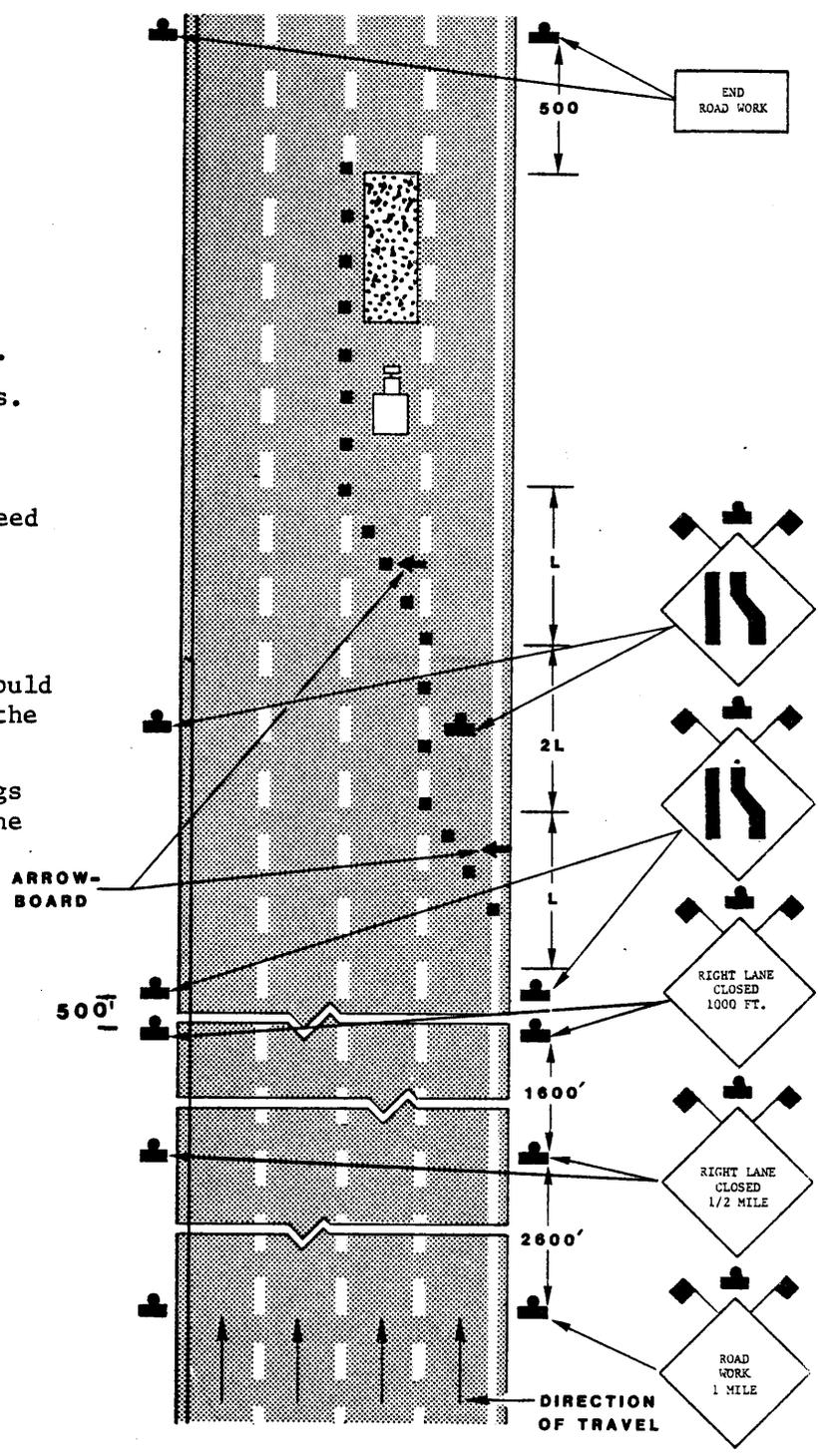
Figure 18. Typical layout for closing two (or more) lanes of a multilane highway.
