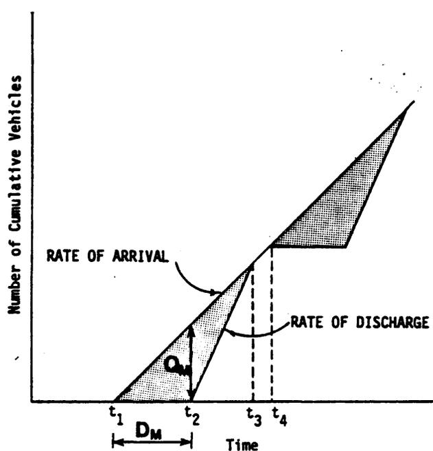
Figure 9. Volume/capacity relationship when traffic stream is temporarily stopped. (From reference 6.)
