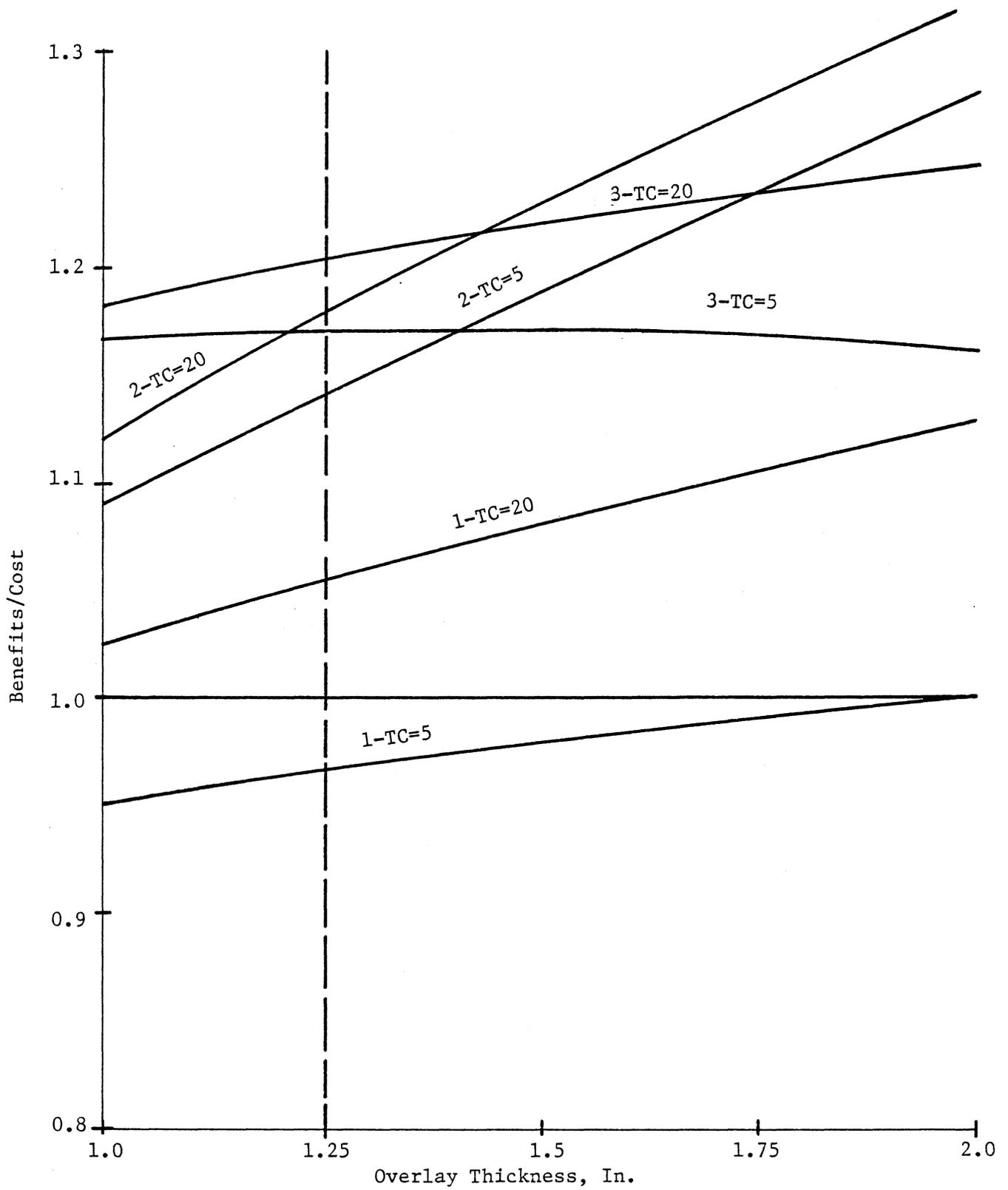
Figure 8. Benefit-to-cost ratio as a function of overlay thickness.
