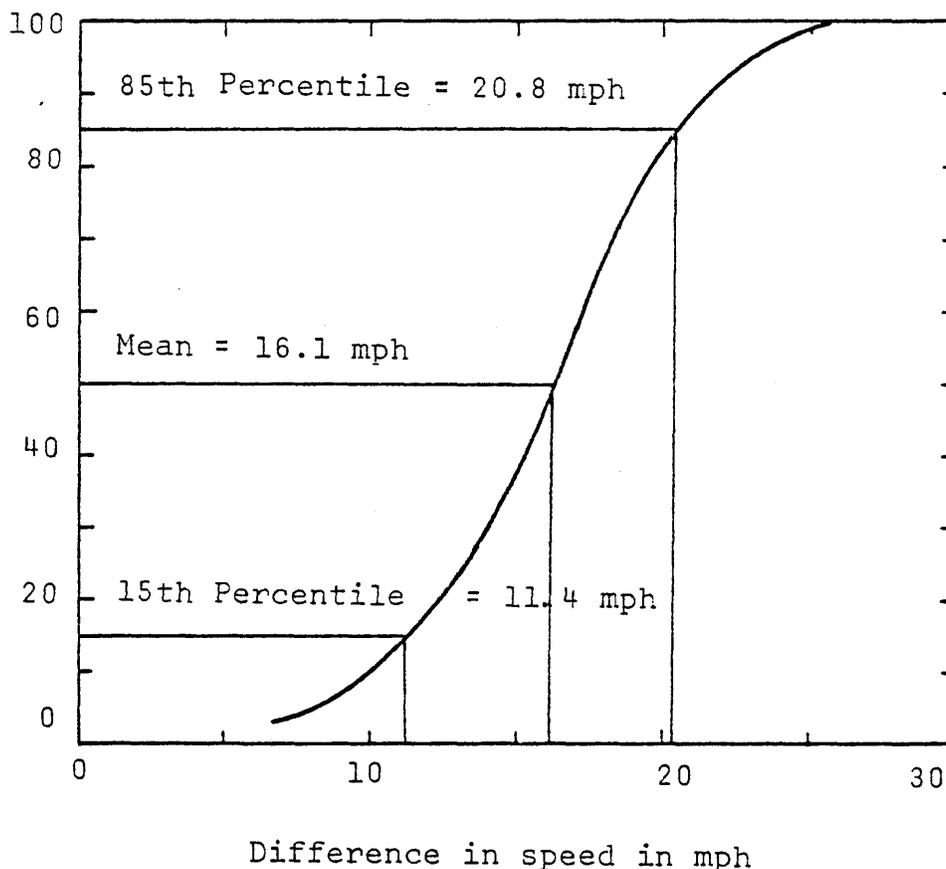
FIGURE 4. CUMULATIVE DISTRIBUTION OF SPEED DIFFERENCE BETWEEN PASSING VEHICLE AND IMPEDING VEHICLE.
