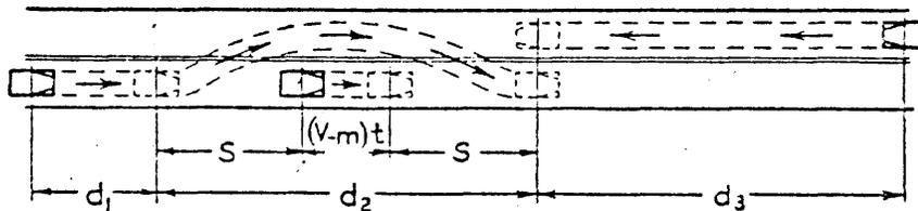
PASSING ONE VEHICLE AT 10 M.P.H. LESS THAN ASSUMED DESIGN SPEED, V. (m=10)
