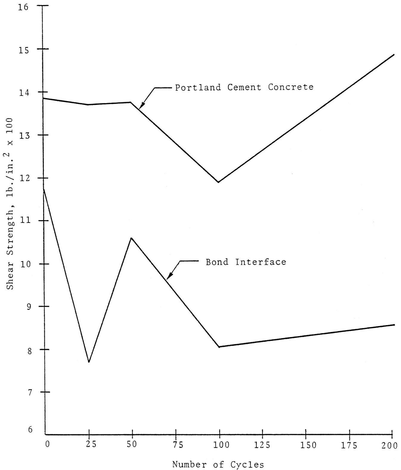
Figure 2. Shear strength as a function of number of thermal cycles. (6.89 kPa = 1 lb./in.<sup>2</sup>)
