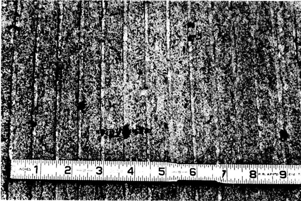
Figure 11            Striations produced by pan shown in Figure 10.
