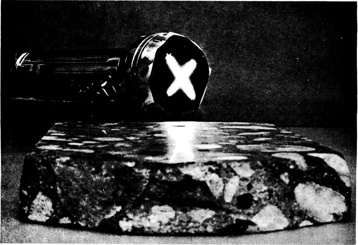
Figure 1. The ability to reflect a light image at a low angle indicates a sufficiently smooth surface.
