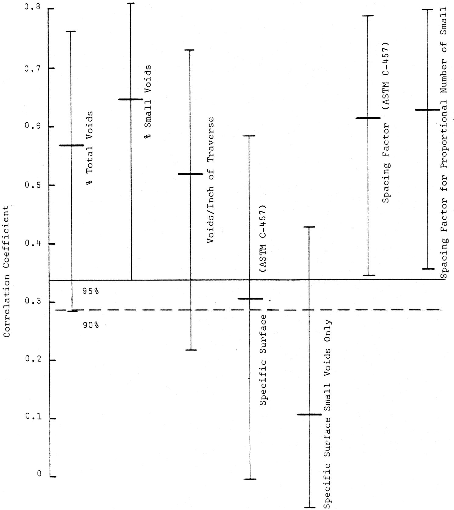
Figure 6. Correlation coefficient - durability factor versus parameters of air void system
