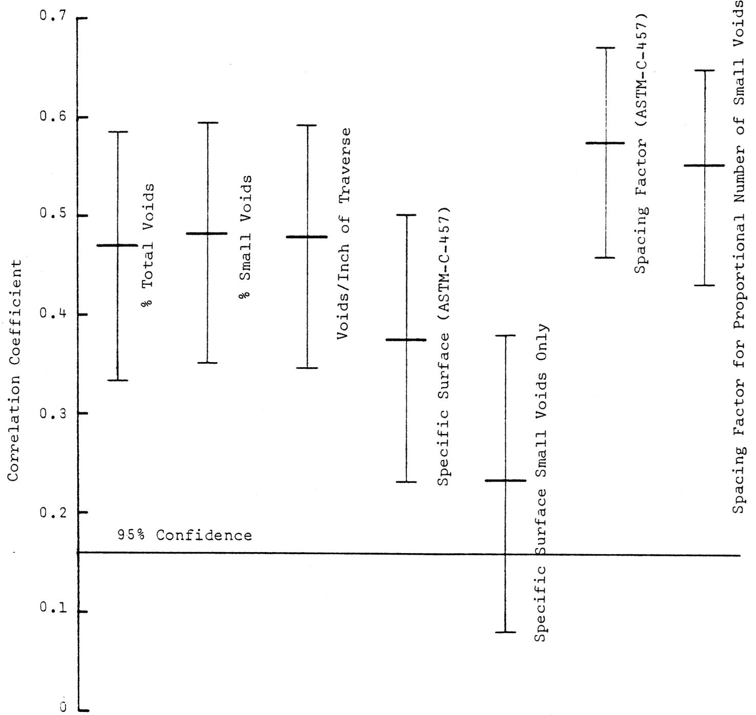
Figure 3. Correlation coefficient — durability factor versus parameters of air void system.
