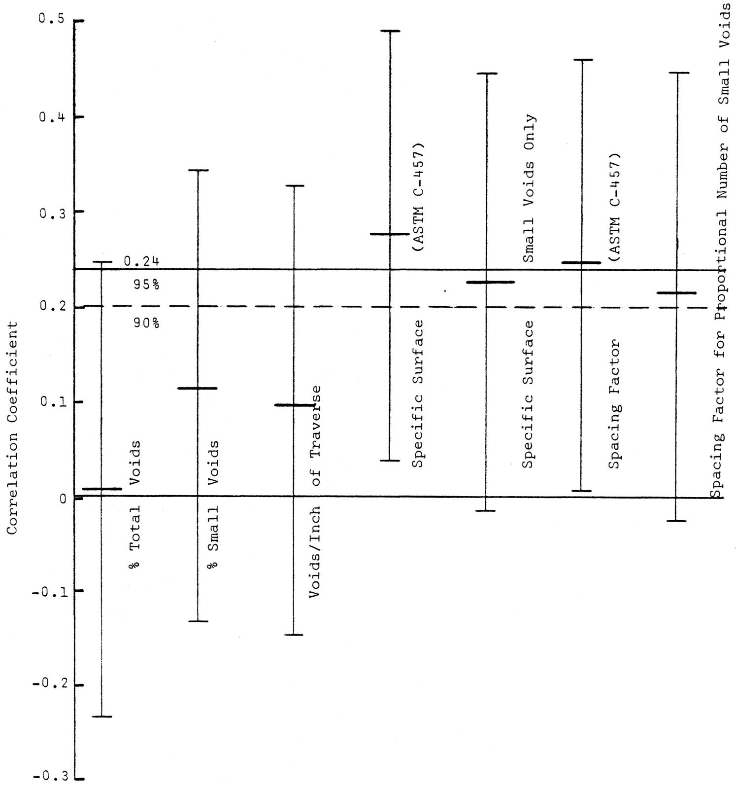
Figure 7. Correlation coefficient - durability factor versus parameters of air void system
