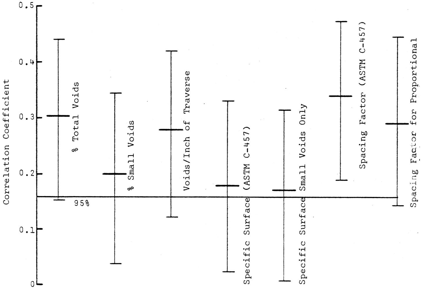
Figure 4. Correlation coefficient - weight loss versus parameters of air void system
