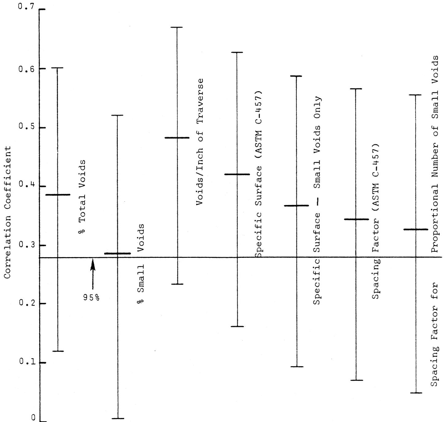
Figure 5. Correlation coefficient — durability factor versus parameters of air void system
