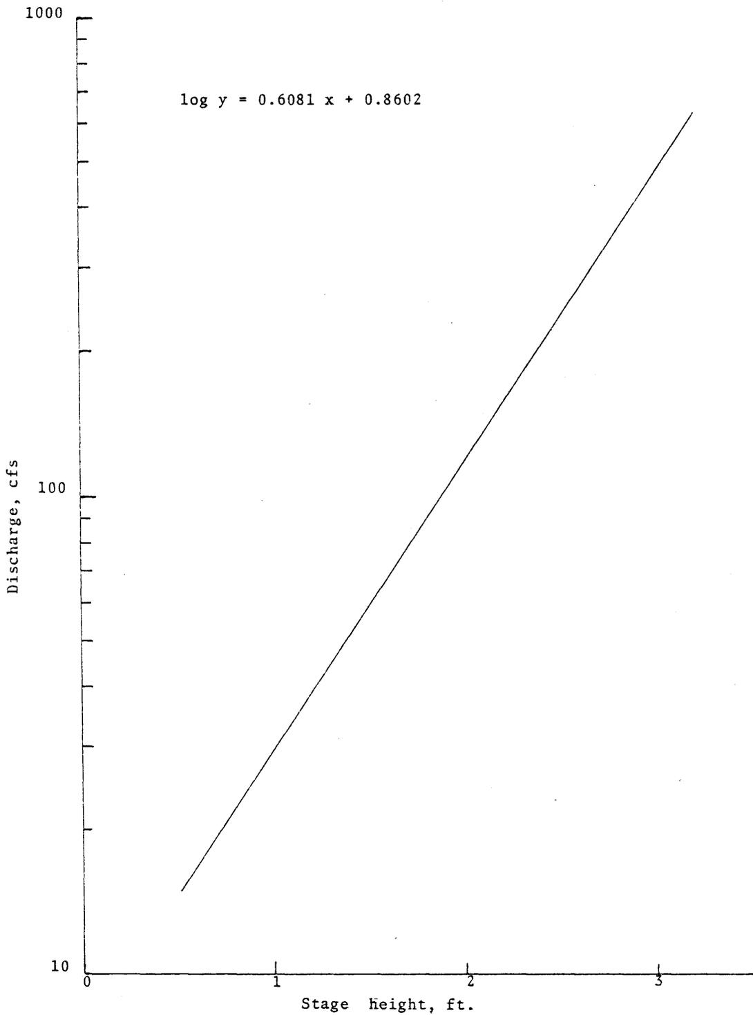
Figure B-2. Stage-discharge curve for Mechums River.
