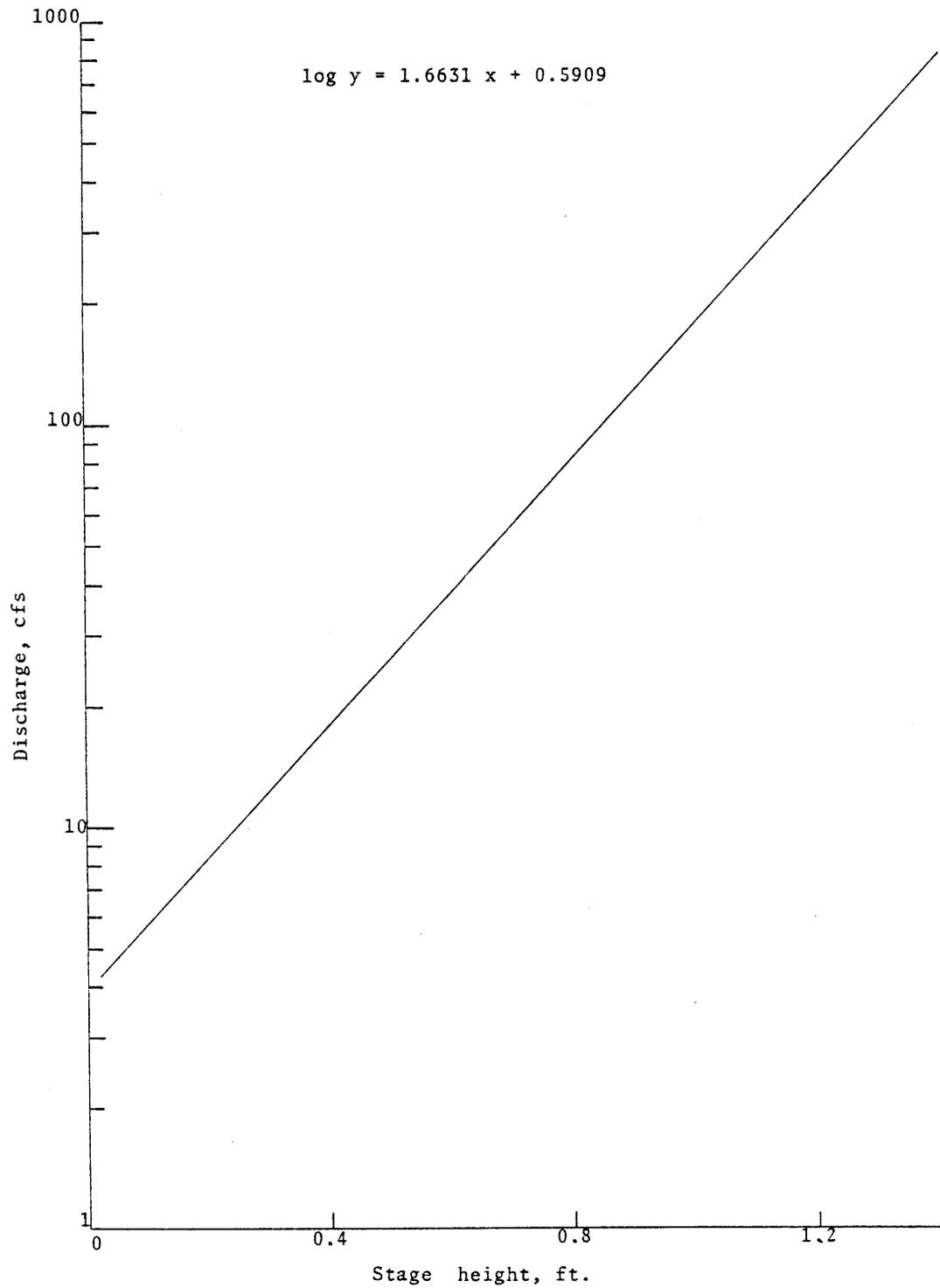
Figure B-10. Stage-discharge curve for Sinking Creek.
