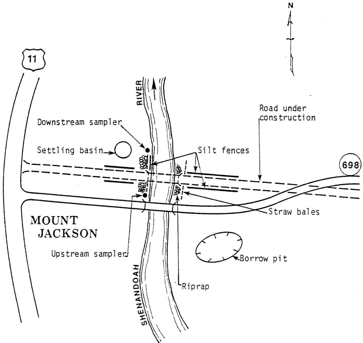
Figure B-11. Plan view of North Fork of Shenandoah River erosion controls and sampler locations.
