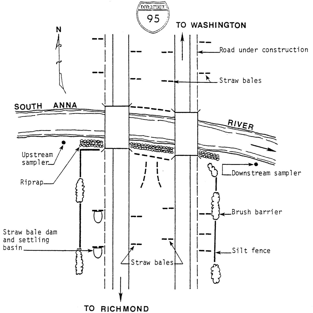
Figure B-13. Plan view of South Anna River erosion controls and sampler locations.
