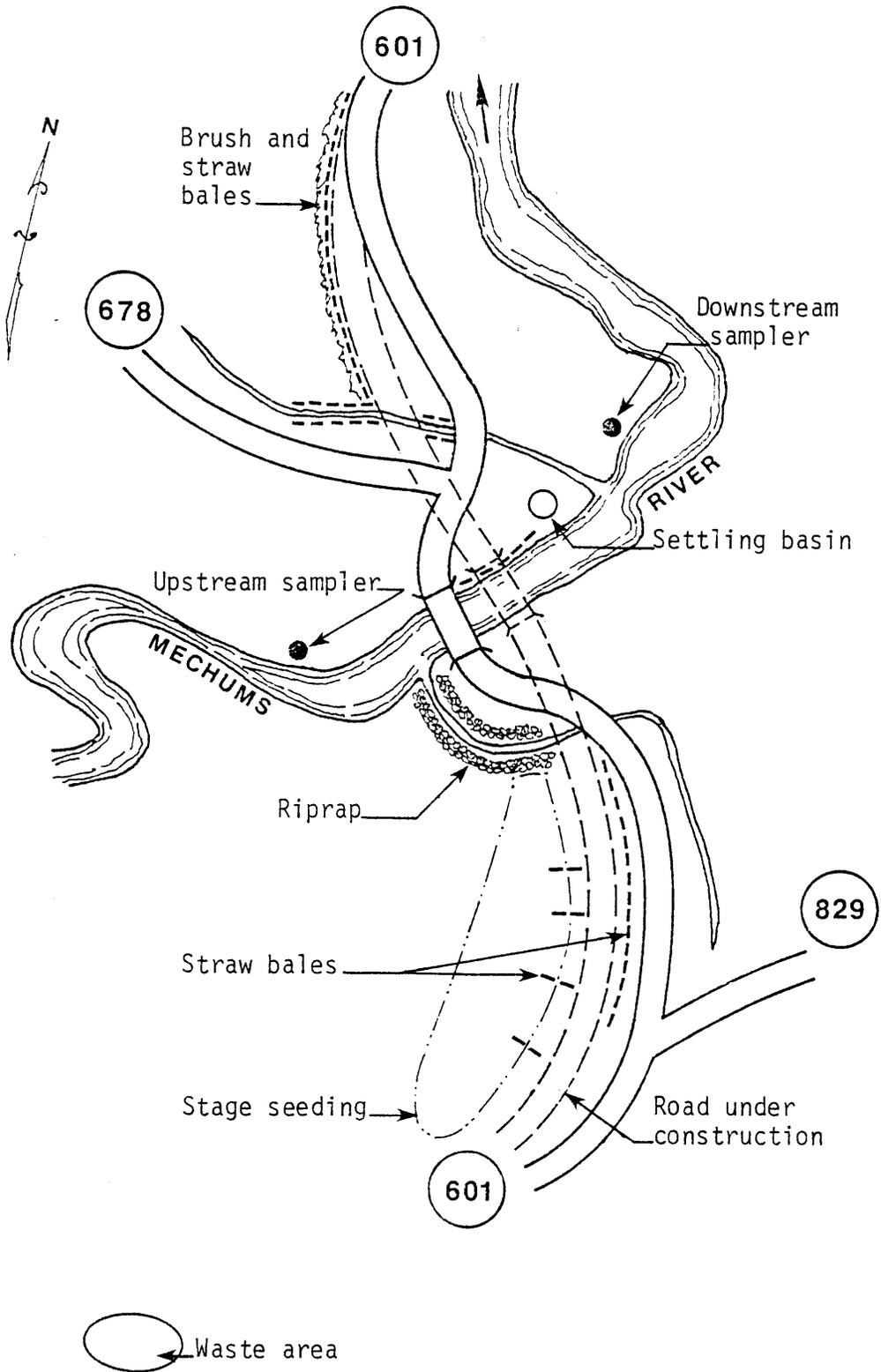
Figure B-1. Plan view of Mechums River erosion controls and sampler locations.
