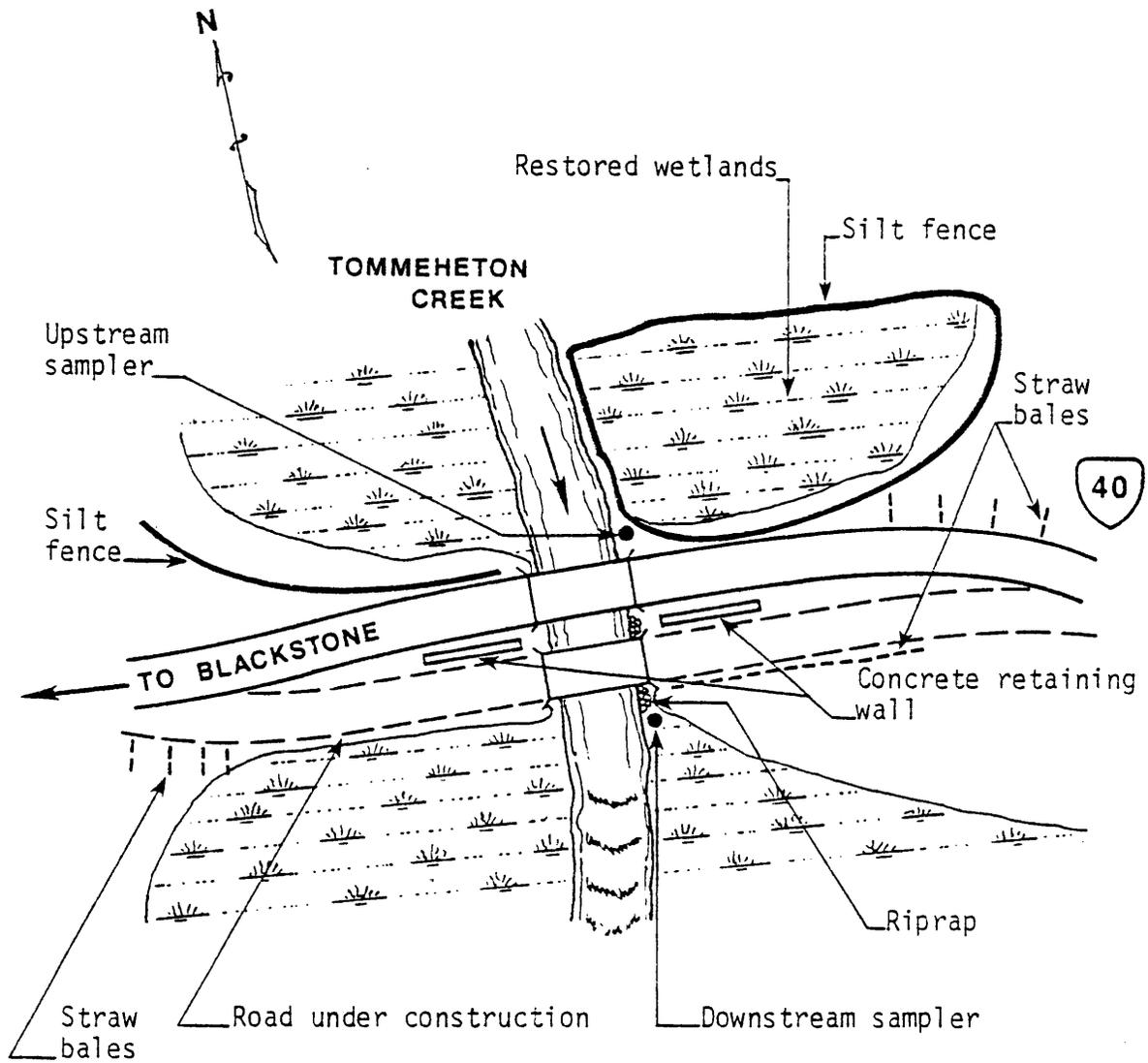
Figure B-7. Plan view of Tommeheton Creek erosion controls and sampler locations.
