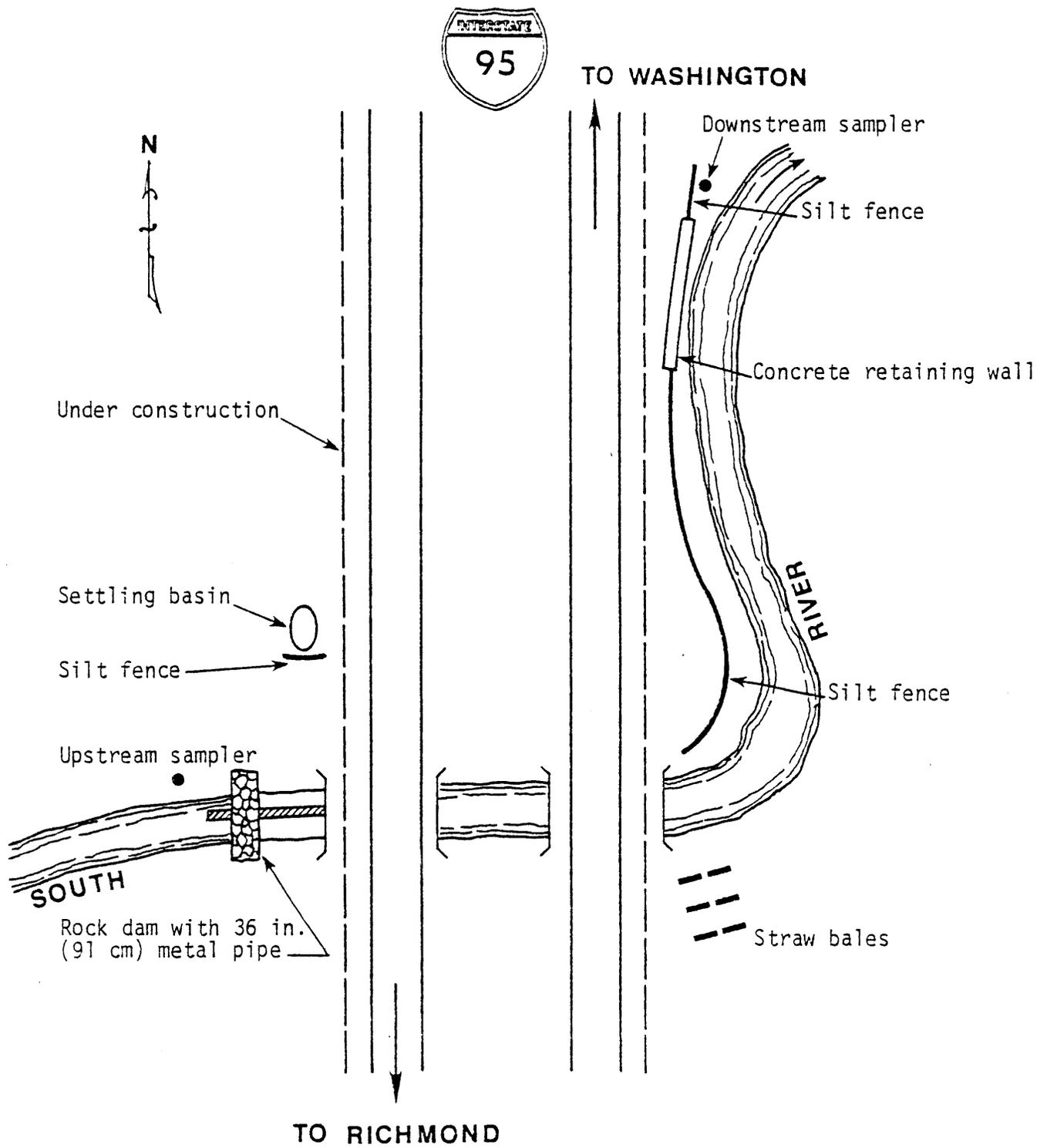
Figure B-15. Plan view of South River erosion controls and sampler locations.
