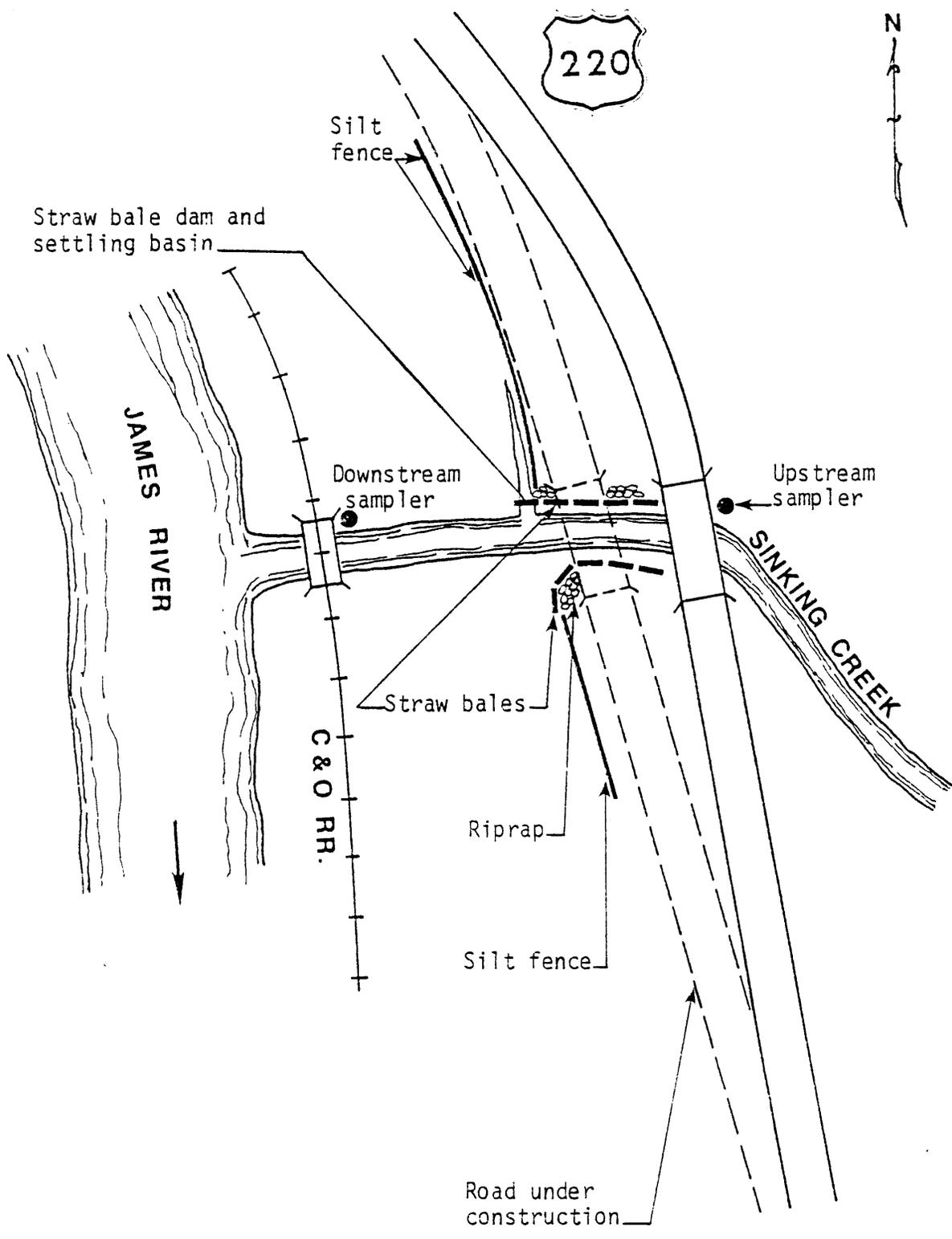
Figure B-9. Plan view of Sinking Creek erosion controls and sampler locations.
