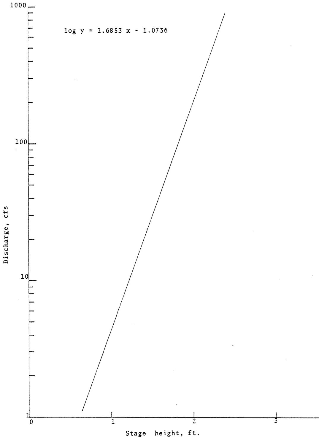
Figure B-6. Stage-discharge curve for Couches Creek.
