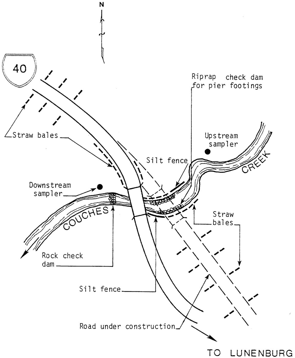
Figure B-5. Plan view of Couches Creek erosion controls and sampler locations.
