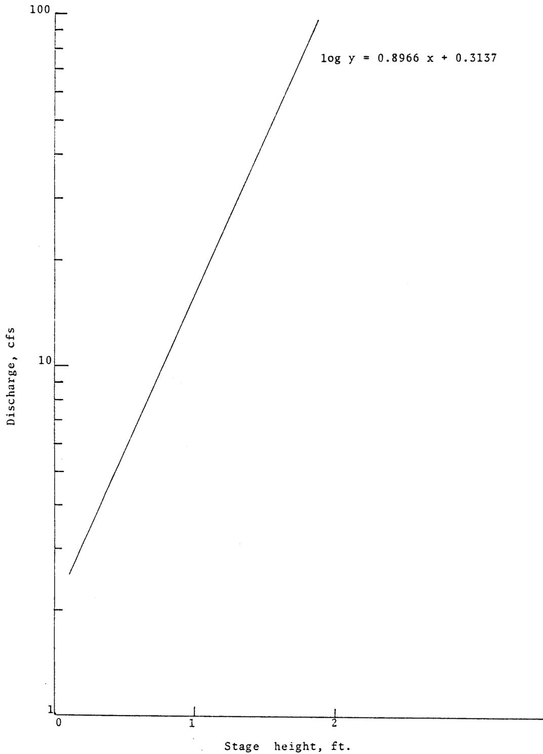
Figure B-4. Stage-discharge curve for Wreck Island Creek.
