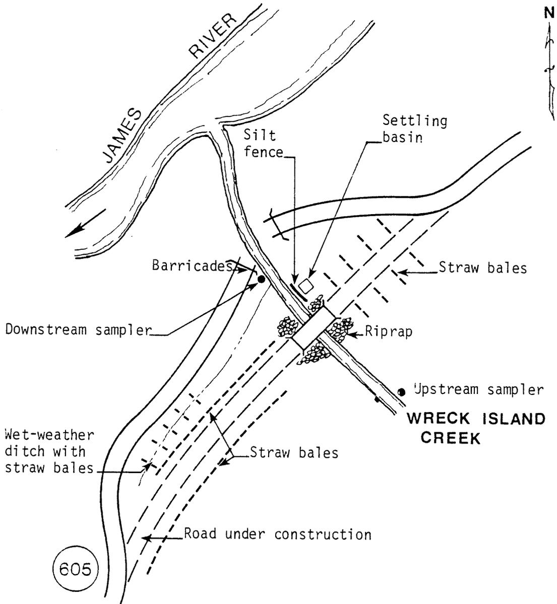
Figure B-3. Plan view of Wreck Island Creek erosion controls and sampler locations.
