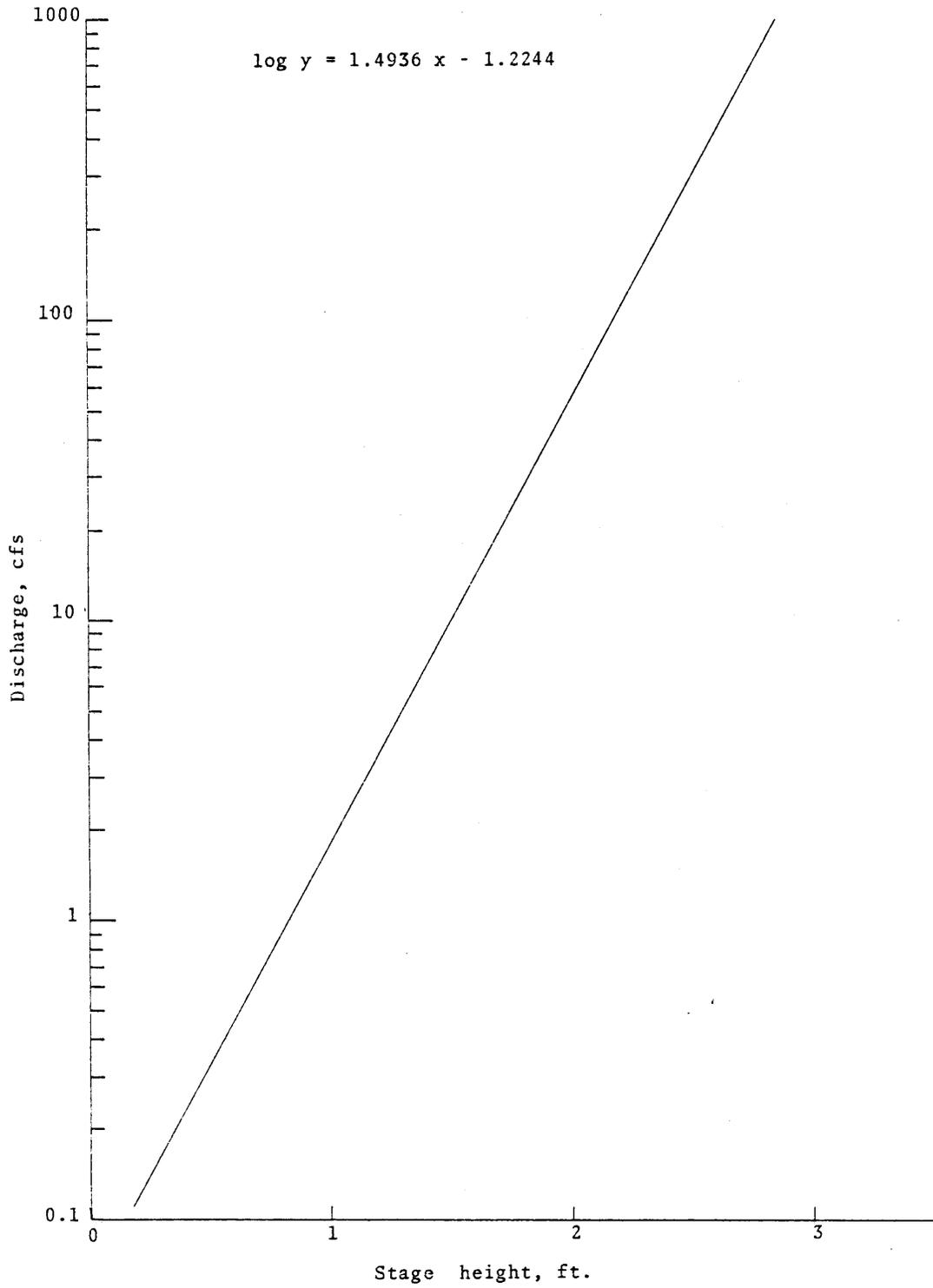
Figure B-16. Stage-discharge curve for the South River.
