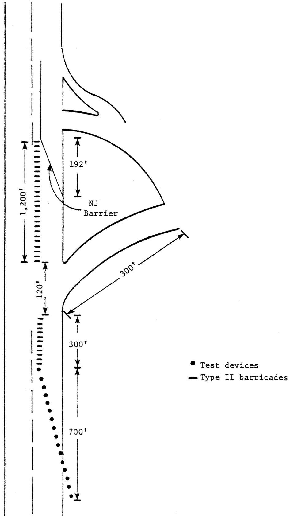
Figure 3. Lane closure for the field tests.
