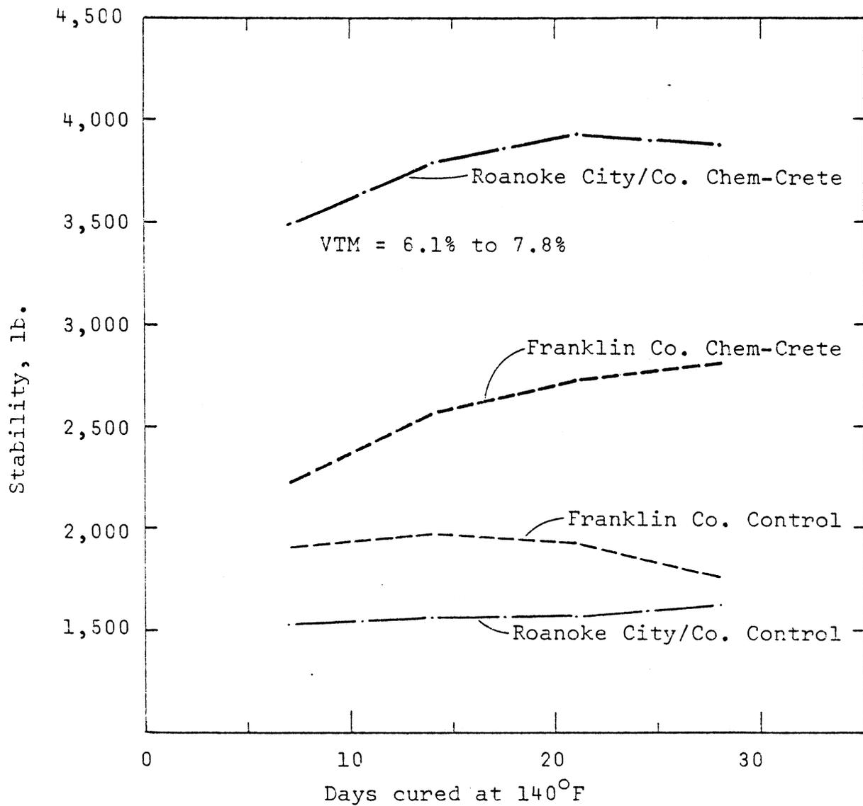
Figure 3. Marshall stability vs. days at 140°F for specimens at pavement density. Tests by Materials Lab. 1 lb. = 4.45 N; °C = 9/5 (°F-32).
