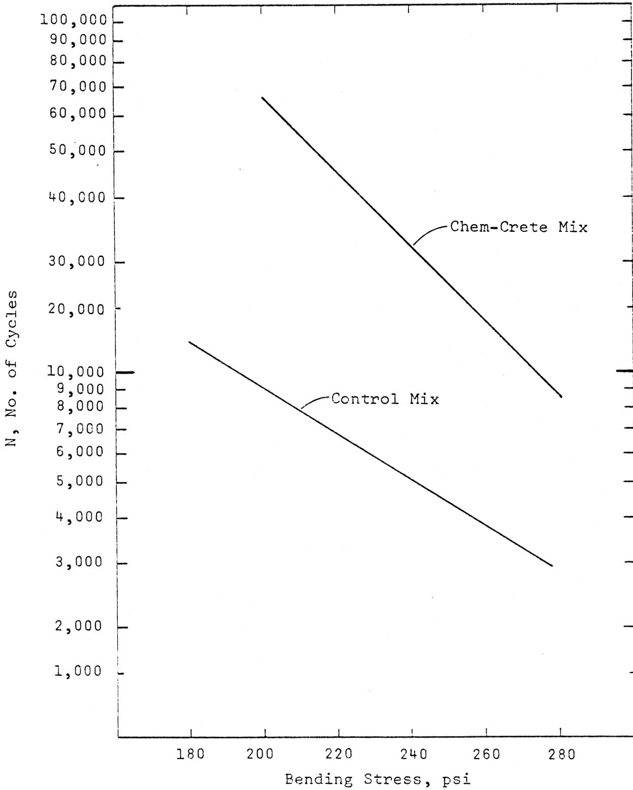
Figure 6. Constant stress fatigue tests.
