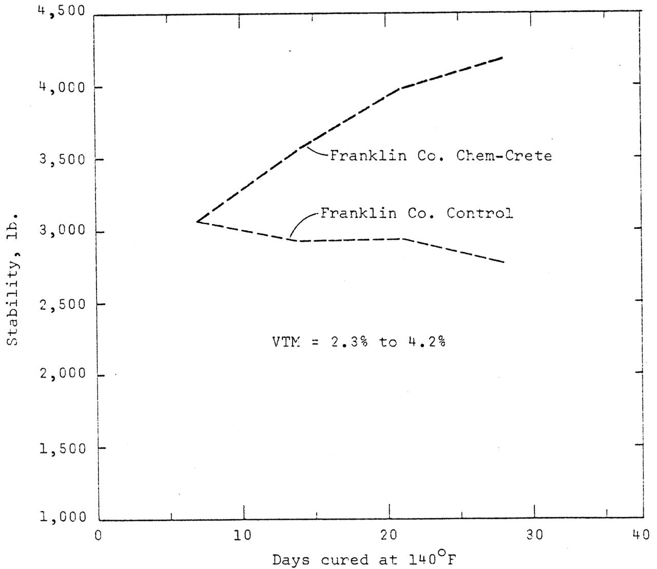
Figure 4. Marshall stability vs. days at 140°F for specimens compacted with 50 blows. Tests by Materials Division. 1 lb. = 4.45 N; °C = 9/5 (°F-32).
