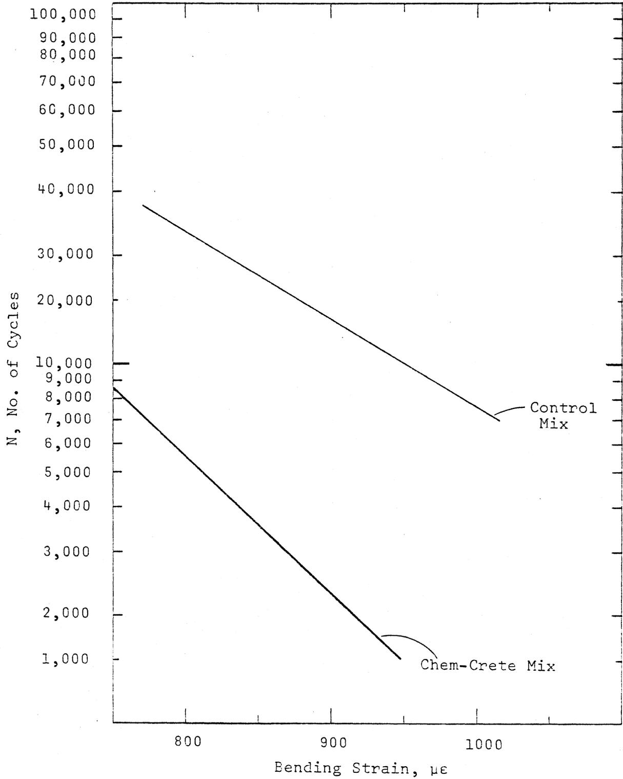
Figure 7. Constant strain fatigue tests.
