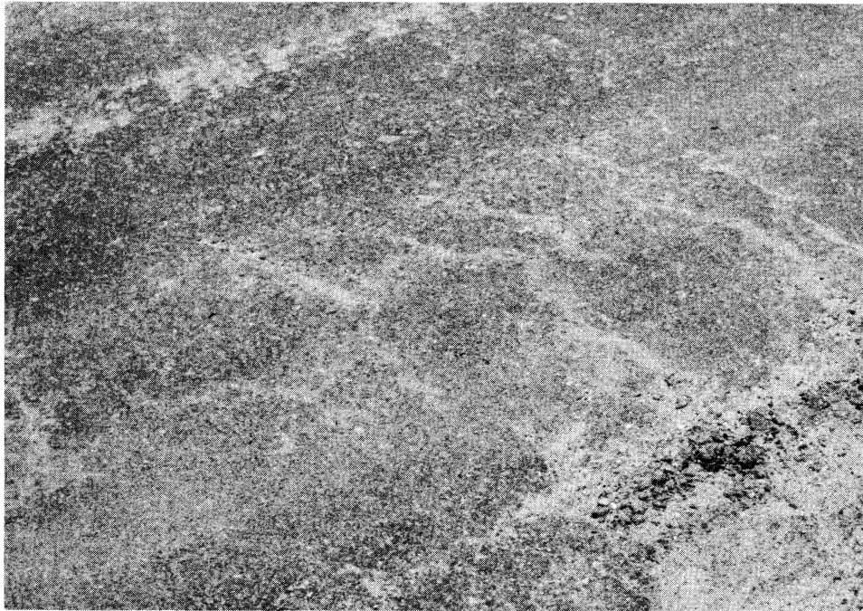
Figure 5. Failures due to final rolling with steel-wheel roller.
