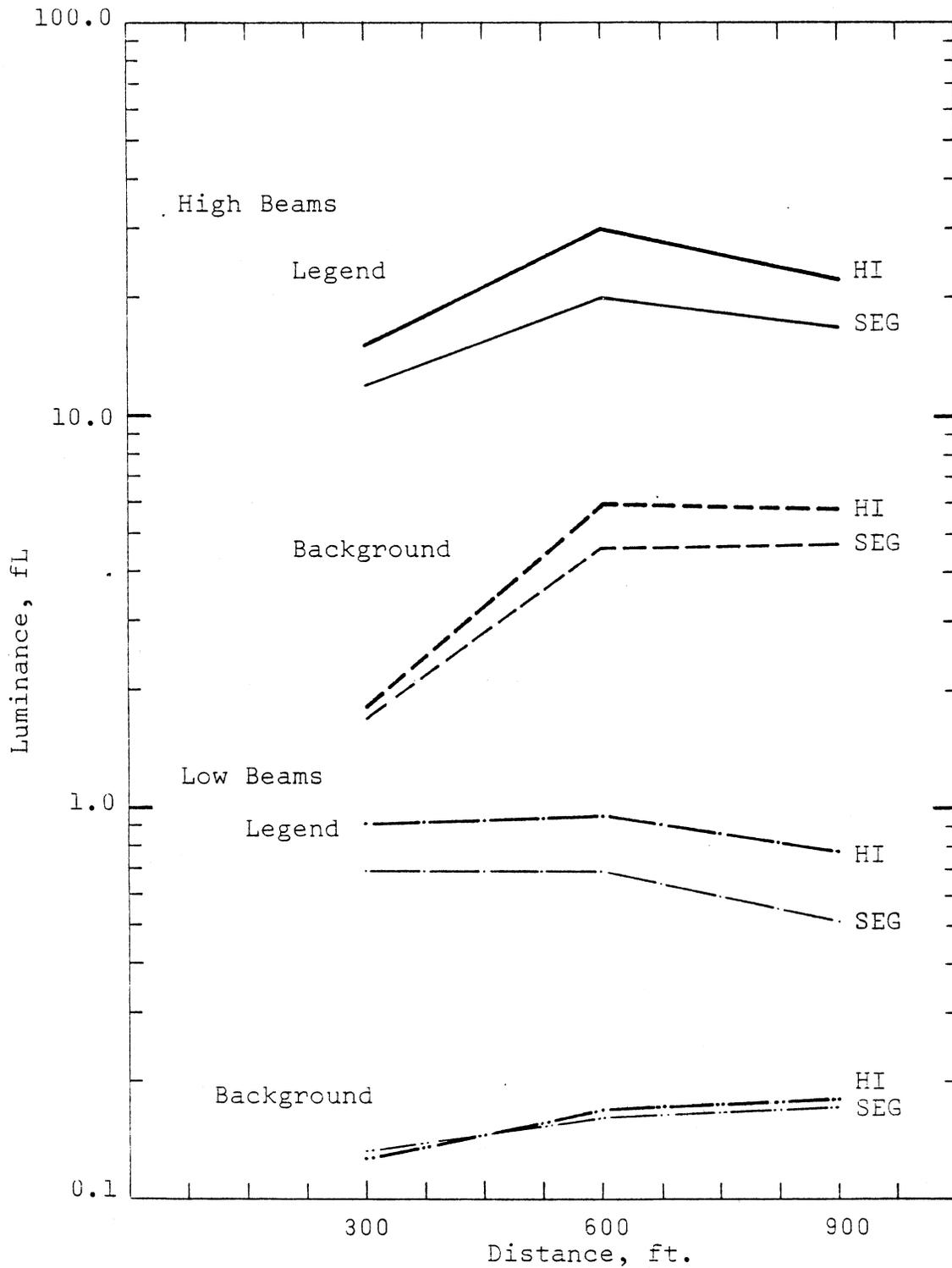
Figure 4. Luminance versus distance — overhead signs.
