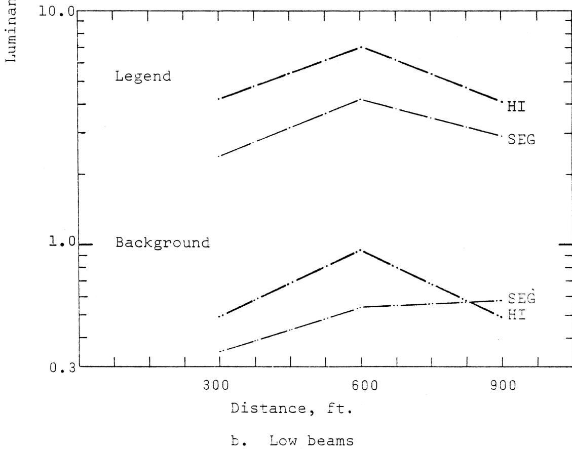
Figure 5. Luminance versus distance — ground-mounted signs.
