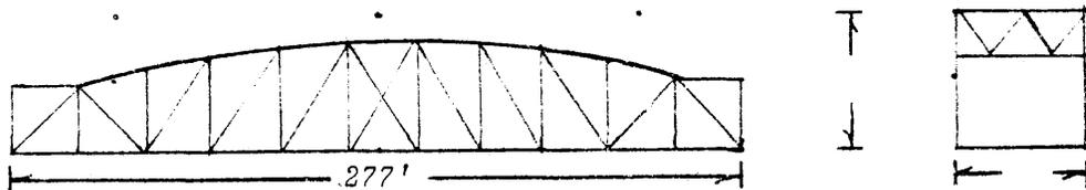
Secondary span type: Pratt camelback Through
