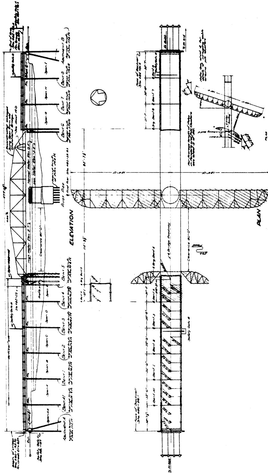
Figure 12. Elevation and plan drawings of the Pungo Ferry Bridge show the asymmetrical nature of the bobtailed swing bridge type.
