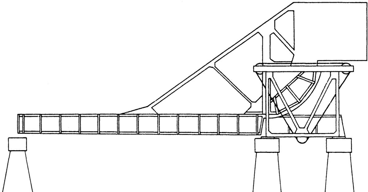
Figure 5. The Scherzer rolling-lift span of the Hodge's Ferry Bridge illustrated in a simple line drawing.
