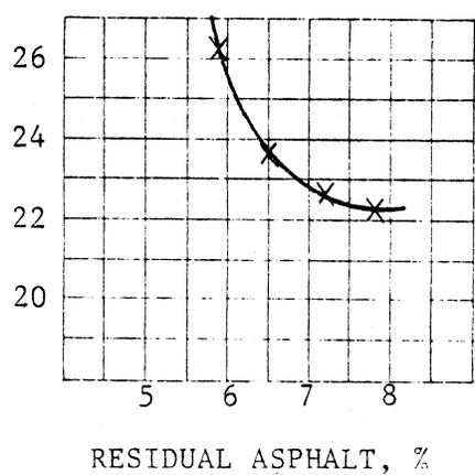
Figure 8. Mix design for sand with Chevron emulsions.
