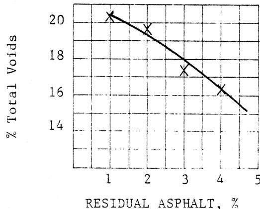
Figure 4. Mix design for granite aggregates with Chevron emulsions.
