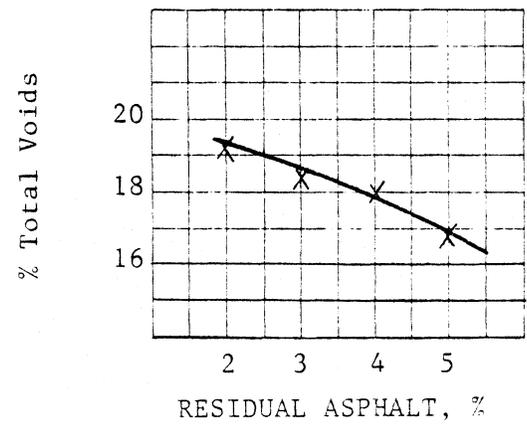
Figure 1. Mix design for limestone aggregate with Central Oil emulsion.
