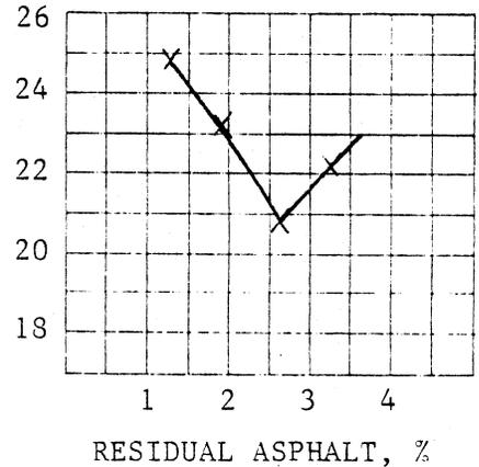
Figure 5. Mix design for recycled aggregates with Central Oil emulsions.
