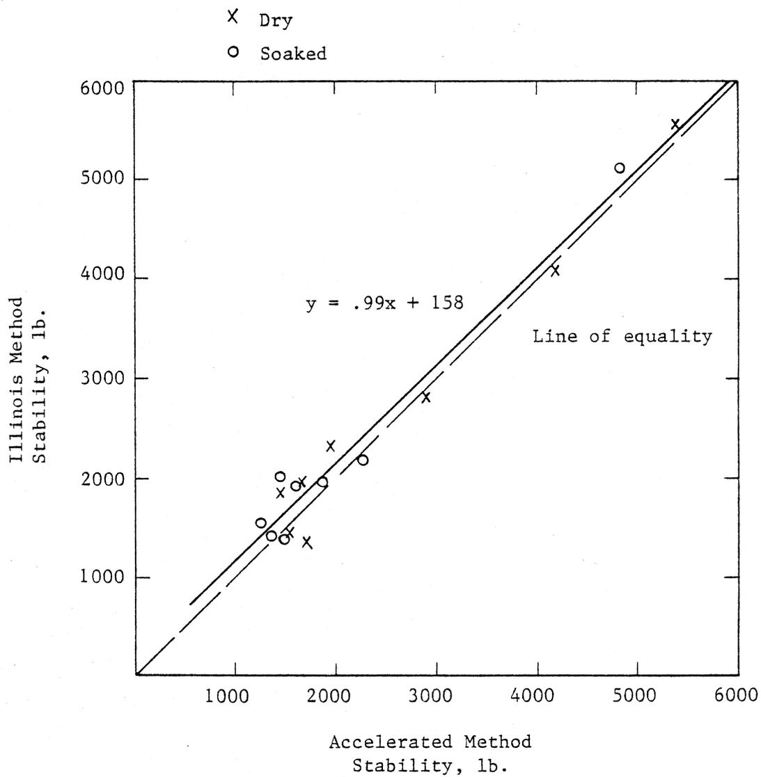
Figure 9. Correlation of Illinois and accelerated cured and soaked specimens.
