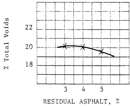
Figure 3. Mix design for granite aggregates with Central Oil emulsions.
