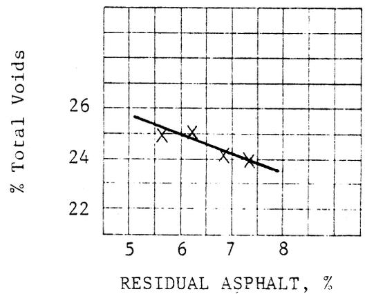
Figure 7. Mix design for sand with Central Oil emulsions.
