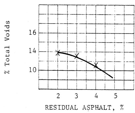
Figure 2. Mix design for limestone aggregates with Chevron emulsions.
