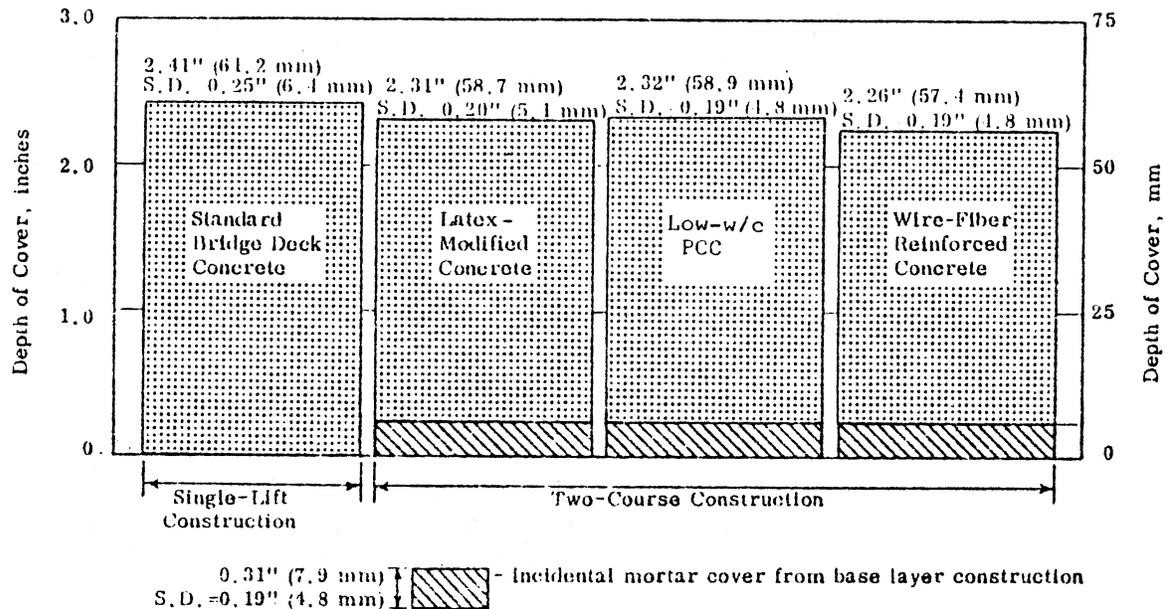
Figure 2. Average depth and variability of cover over topmost reinforcing steel for eight study spans.
