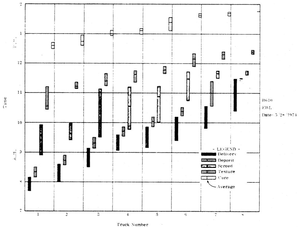
Figure 5. Sequence and times for installation activities for control spans (WBL span above, EBL span below).
