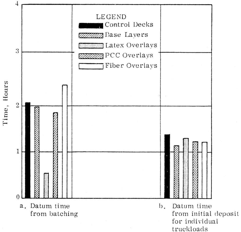
Figure 4. Average times to completion of the screeding activity.
