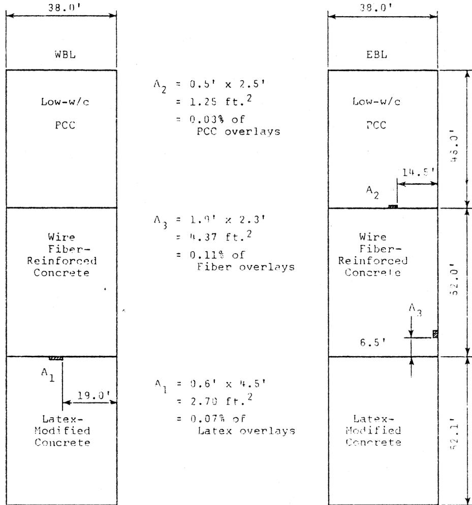
Figure 3. Unsound areas on two-course study spans detected using chain drag, hammer, and FHWA "Delamtect".
