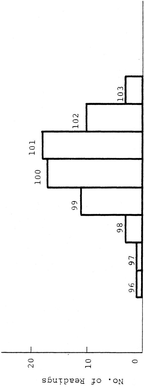
Figure 1. Percentages of rodded weight for 69 readings on low-slump concrete, for NBLs with a w/c of 0.328.
