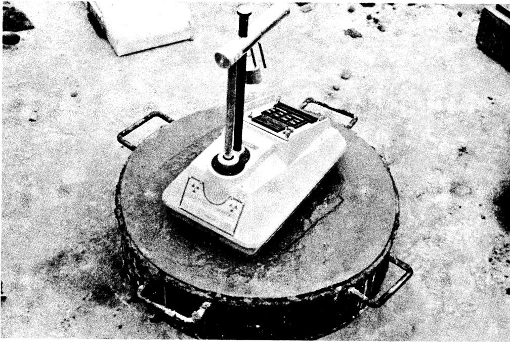
Figure 3. Nuclear gage and metal container used to determine correction factors.
