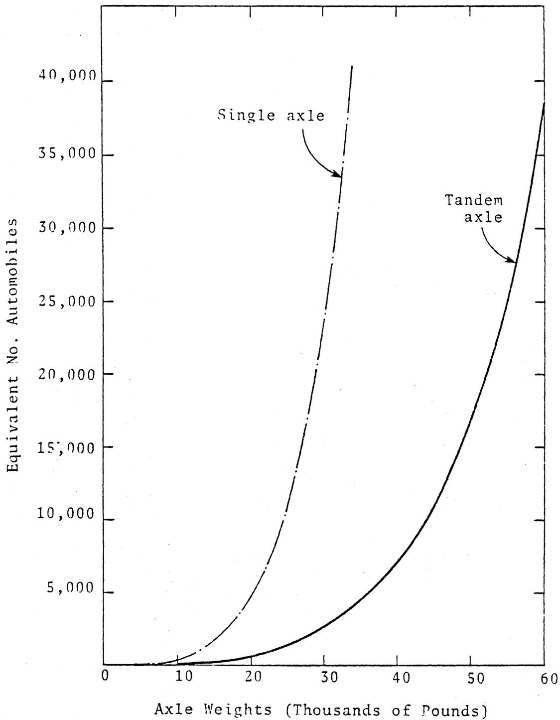
Relative Damage Caused by Increase in Axle Weights
