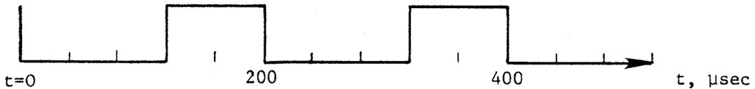
Figure 4. Central processor normal control signal.
